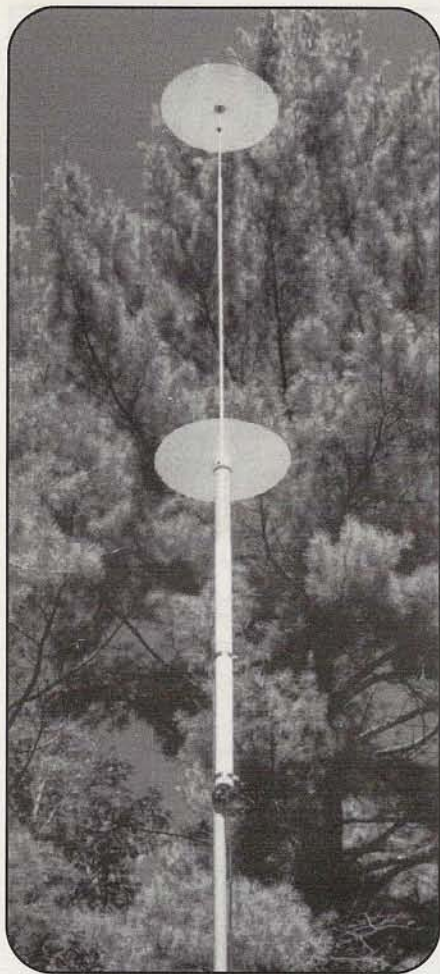
The discpole antenna is light enough to be mounted on 36-foot telescopic mast without guying. (Photos by the author)
