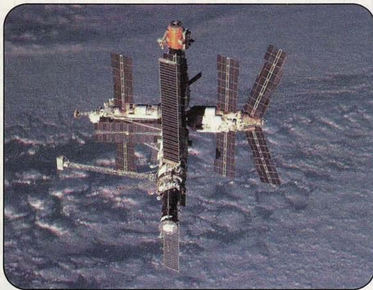
The Mir space station complex includes two ham stations: one on 2-meter FM voice and packet, and another on 70-centimeter voice and packet, including an FM repeater. These photos were taken during shuttle mission STS-79 in September, 1996. (NASA photo S79E5327)
