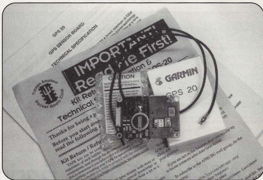
The Garmin GPS 20, as received from TAPR. The antenna cable with the MCX connector is shown. Since the unit is not weatherproof and is static-sensitive, you must mount it inside a case.
