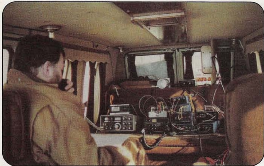
KØDAS/R interior. The rigs are secured to a plywood sheet laid across the rear bench seat. The operator here is Joe Culwell, WBØYFL.
