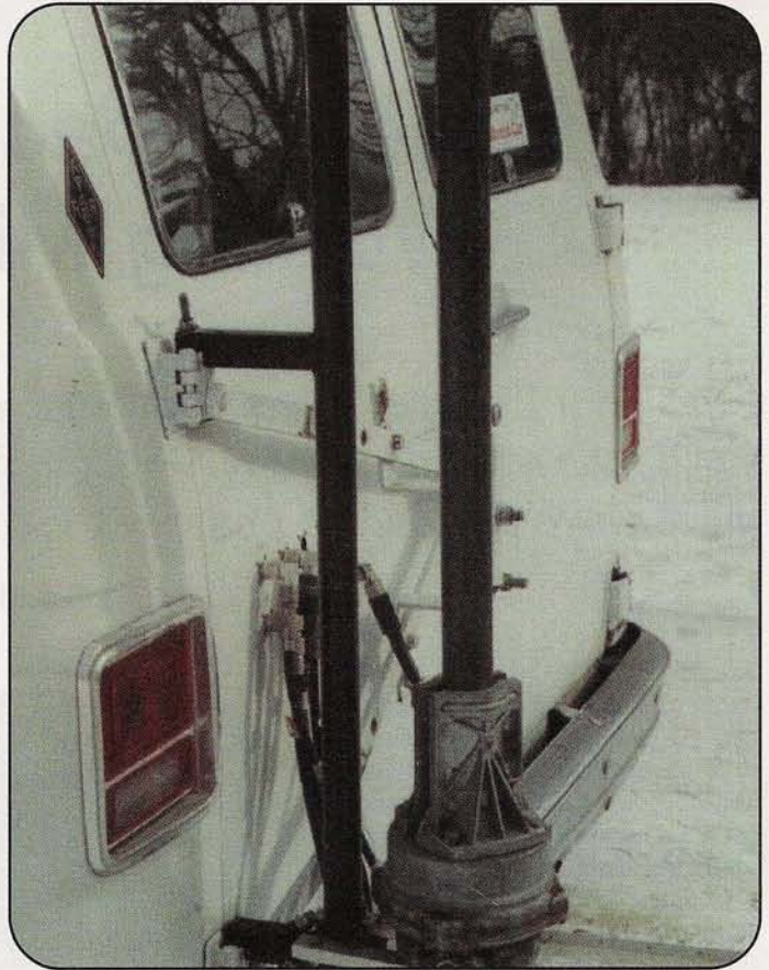
Close-up of KAØYSQ/R's rotator assembly. The rotator and main mast pivot at the lower door hinge. An eight-foot stub pipe, mounted to both door hinges, secures the main mast at the top. Half-inch super-flex hard-lines to the antenna connect through bulkhead coaxial connectors in the rear door. No open windows for winter roving here!
