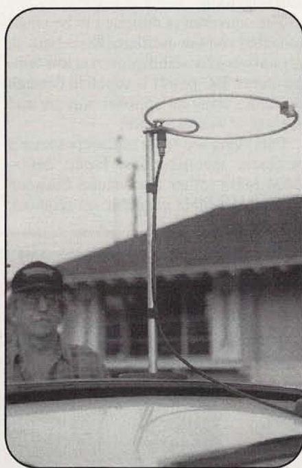
Loop antennas, such as this KB6KQ "Super Loop," are popular among 2-meter SSB mobile operators who use horizontally polarized antennas. (All photos by the author)
