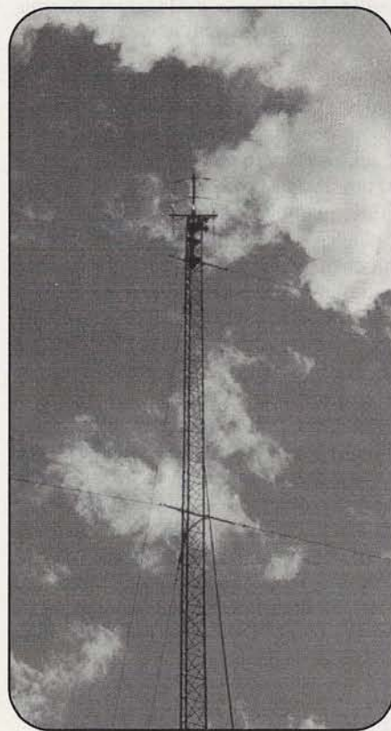
Antenna array at the Boulder, Colorado, ionosonde station. The antennas create a conical pattern used for "taking pictures" of the ionosphere directly overhead. (Photos by the author)
