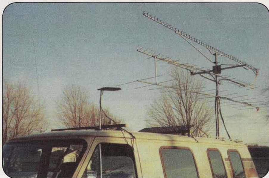
Exterior view of the author's rover van. A 6-meter whip and 2-meter M 2 Loop are mounted forward. At the rear, mounted on a telescoping rotatable mast, are Yagis for 144, 432, 903, and 1296 MHz. The rotator mounts on a plate bolted to the trailer hitch. A cross brace and mast bearing clamped to the top door hinges secure the upper part of the mast.
