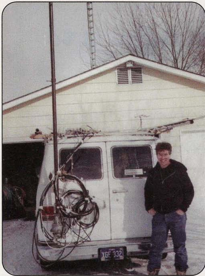
Rear view of KAØYSQ's rover station. Bryan has a 20-foot-tall, tilt over, rotatable steel mast and carries Yagis for seven bands (50 through 2304 MHz) on the van rack. He and a trained accomplice can stop, mount all antennas (including mast-mounted pre-amps and power amplifiers for the top three bands) and be on the air in less than 15 minutes!
