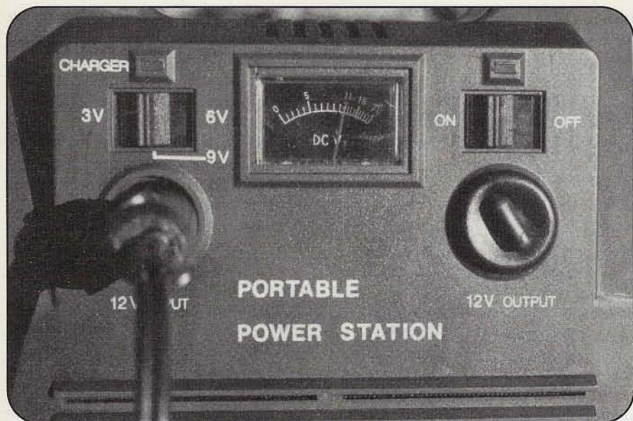
The meter that comes with the Power Station is very hard to read in the 12- to 15-volt range. Replace it if you can (see text for details).
