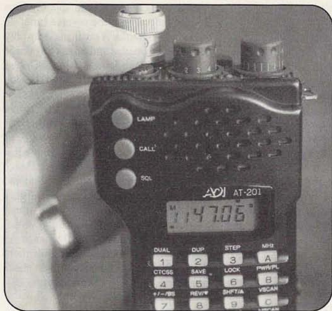
↑ The squelch control on the AT-201 is recessed but accessible, unlike some HTs today that make squelch a menu function.
