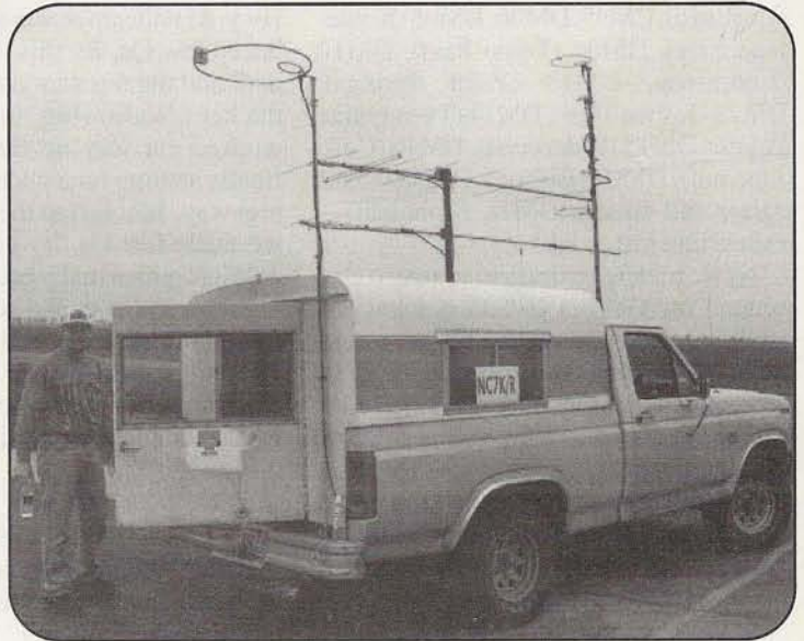
It's leg-stretching time in CM99. This photograph, taken at a stop in grid square CM99, provides an excellent view of the rover's antennas (described in detail in the text).
