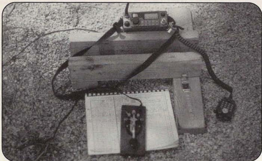
WB2AMU/R's makeshift station setup at one of his operating stops. Wood planks found on the ground held up the rig and "station clock," while his hand key kept the logbook in place. No computer logging on this operation!
