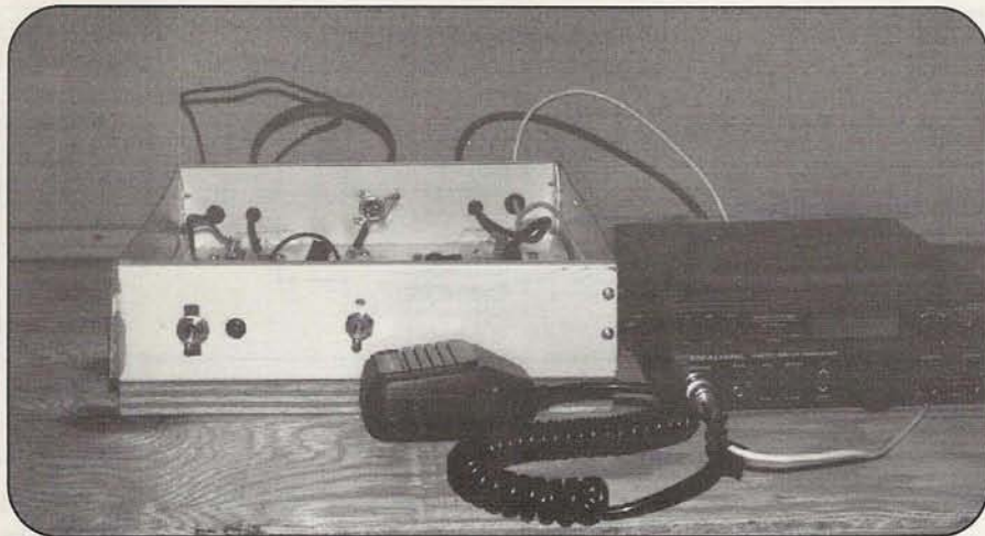
The author's completed 2-meter CW/SSB station. The transverter is on the left, and the 10-meter transceiver used as the IF is to its right.
