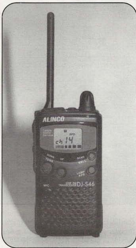
Look familiar? Alinco's DJ-S46 HT for the Family Radio Service is identical in design to its DJ-S41T 70-centimeter ham rig. Sharing development costs let Alinco price the ham HT under $150.
