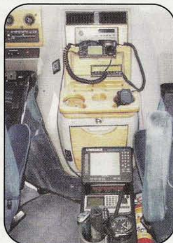
"NOA's ARC"—CQ VHF Senior Contributing Editor Gordon West, WB6NOA, recently traded in his 20-year-old station wagon for a customized "Amateur Radio Communications" van, which he's dubbed, "NOA's ARC." The van is equipped with radios and antennas for 1.8 MHz through 10 GHz, plus a 4.5 kilowatt generator to power everything. There are three operating positions inside, one each for HF, VHF/UHF and satellite/microwave. One of the operating positions is shown. (Tnx WB6NOA)
