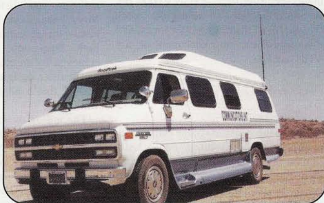
"NOA's ARC"—CQ VHF Senior Contributing Editor Gordon West, WB6NOA, recently traded in his 20-year-old station wagon for a customized "Amateur Radio Communications" van, which he's dubbed, "NOA's ARC." The van is equipped with radios and antennas for 1.8 MHz through 10 GHz, plus a 4.5 kilowatt generator to power everything. There are three operating positions inside, one each for HF, VHF/UHF and satellite/microwave. One of the operating positions is shown. (Tnx WB6NOA)
