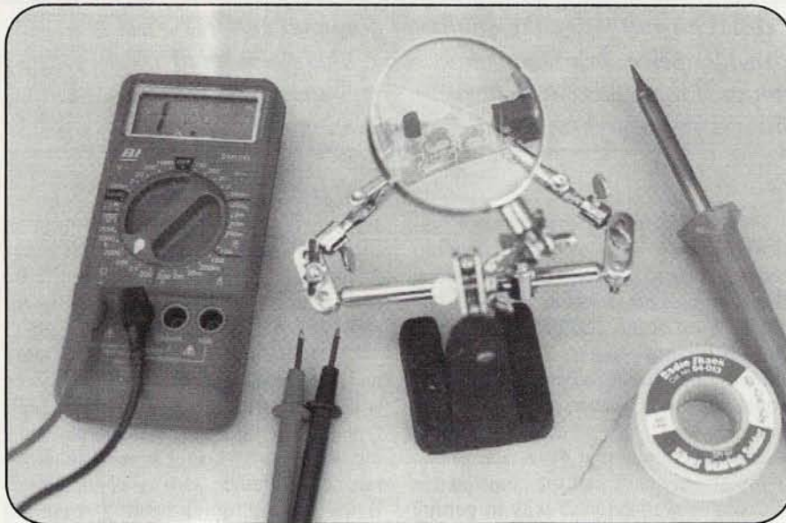
Photo D. A few special tools make working with small projects and crowded pc boards a cinch. Shown here is a multirange pocket Volt-Ohm-Milliamp meter, a "third hand" jig with magnifier, a 15-watt soldering iron with fine tip, and ultra-thin silver bearing solder.
