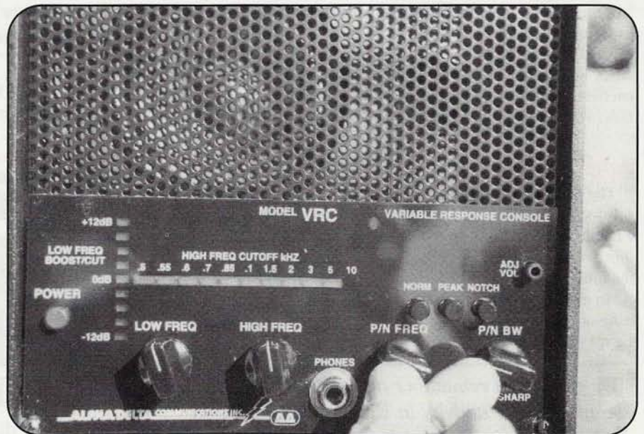
The front panel of the Alpha Delta VRC Speaker System contains controls to let you customize the speaker's response to the specific type of signal you're trying to hear (or to notch out).
