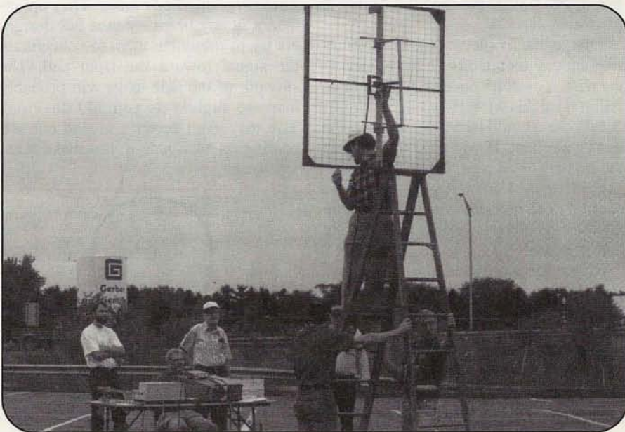
Photo B. John Rose, WW1Z, uses a homebuilt 222-MHz antenna standard (based on an NBS/EIA design) as a reference antenna to calibrate the range. Joe Reisert, W1JR, is seated at the table, adjusting the network analyzer.
