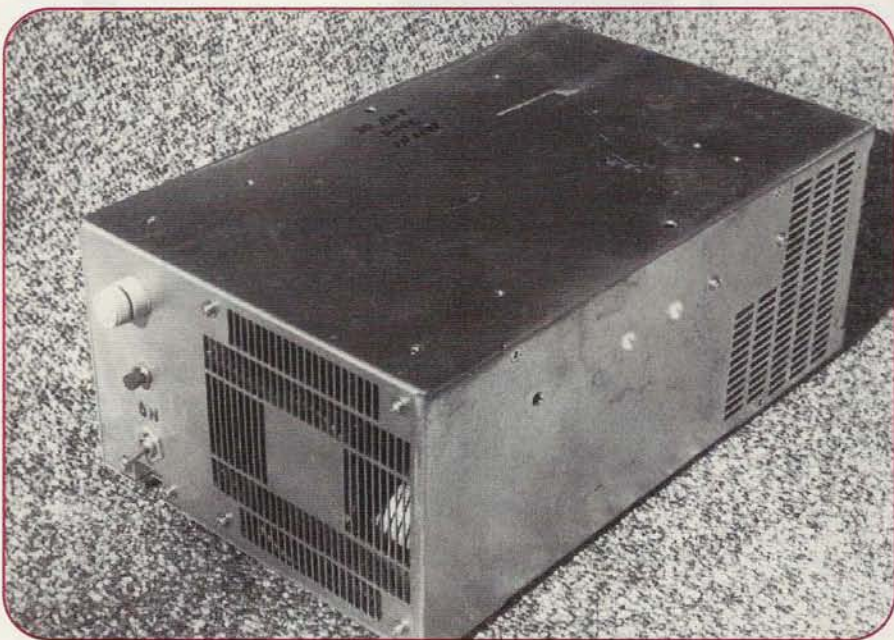
Exterior view of the K3YWY power supply. It provides a reliable source of 12-volt power at current levels of up to 25 amps. (Photos by the author)
