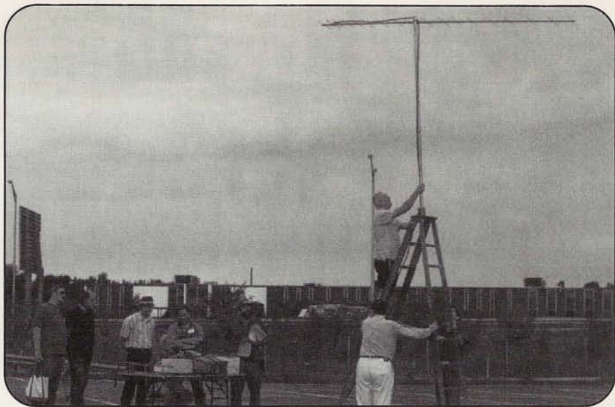
Photo E. Here Stan Hilinski, KA1ZE, tests his 18-element 432-MHz Yagi. Its gain was measured at 14.12 dBd.
