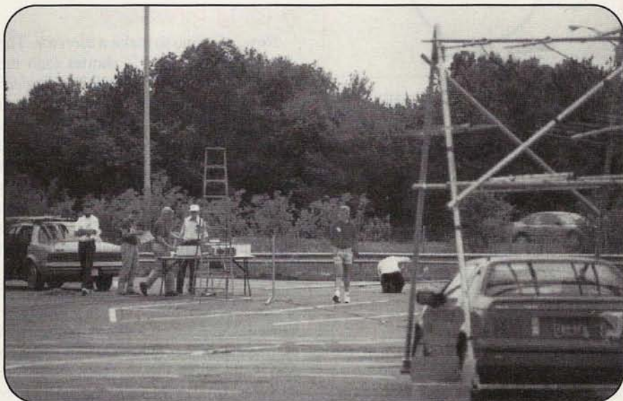
Photo A. The antenna range at a recent Eastern VHF/UHF Conference. The car contained the "source" antenna, while the test antennas were held above the ladder at the opposite end of the range. (Photos by the author)
