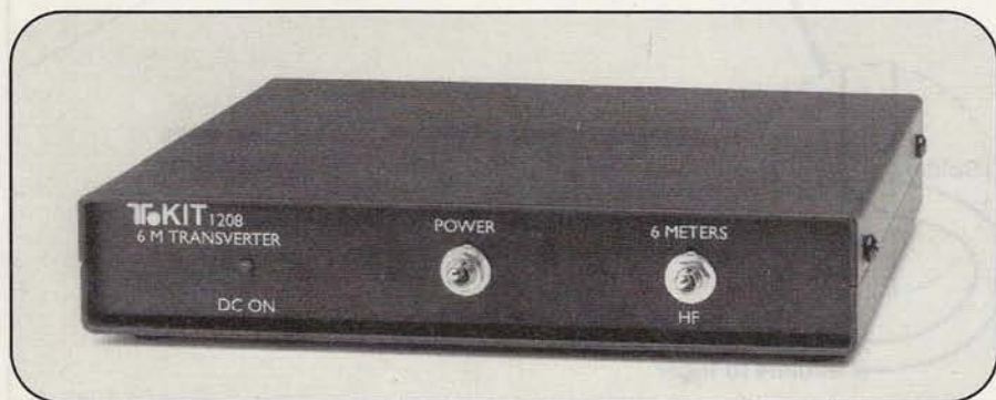
Photo B. Ten-Tec's 6-meter transverter kit is an ideal way to add 50 MHz operation to HF-only transceivers. The unit is quite affordable, goes together in approximately 16 hours time, and works great on SSB, CW, and FM.
