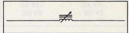
Figure 8. Schematic symbol for a variable inductor. These serve similar roles to variable capacitors in tuning the inductance of a circuit to an exact value.
