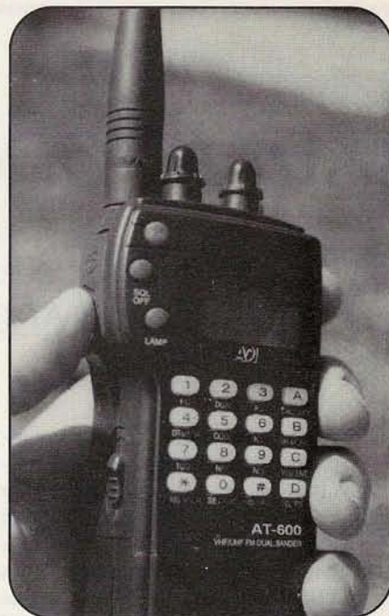
The push-to-talk (PTT) switch on the AT-600 can be tricky. Be sure you press the lower part of the side button, as the top part is the "function" switch.
