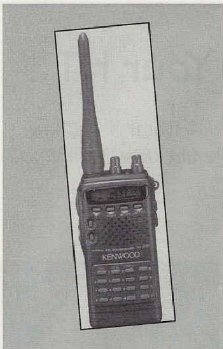
Kenwood's TH-22AT is typical of modern handhelds, packing a 5-watt transmitter into a very small case. The manual warns of overheating danger if you transmit too long on high power.
