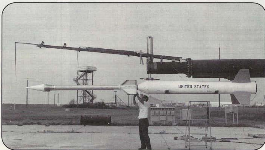
This is one of the most successful ionospheric sounding rockets in history, the Nike-Cajun, which stands over 25 feet long. It was first launched for this purpose in 1956 from Wallops Island, Virginia. (NASA photos)
