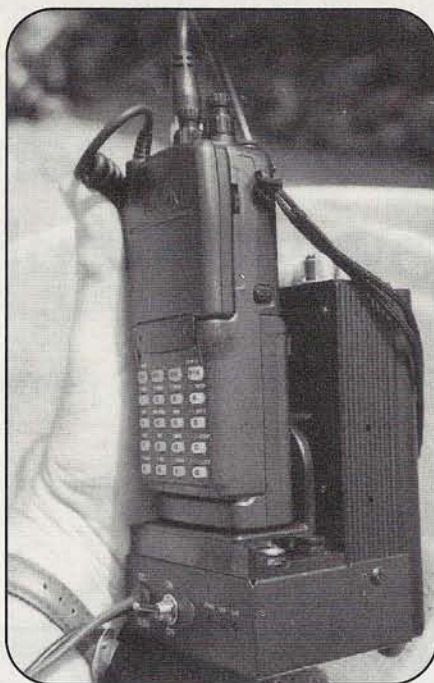
The unit is small enough and light enough to hold in one hand, but be careful about picking it up when you've been using it for a while. The amplifier may be hot.
