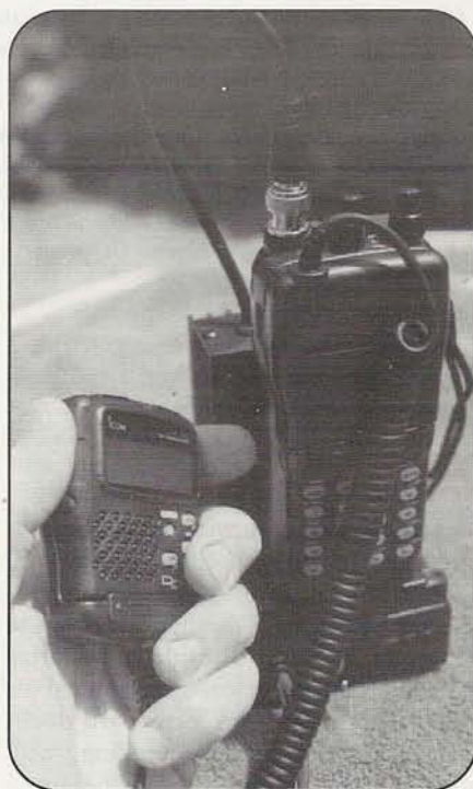
Maha's HT docking booster, model MH-A302, provides a combination HT support stand and dual-band power amplifier.
