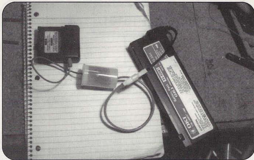
The whole switching regulator circuit—the PT-5101 plus two capacitors—can be built into an empty film can, which goes between a long-life battery and the HT power pack.
