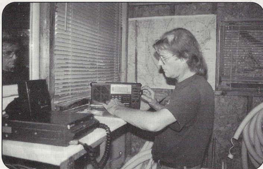
You don't need to invest in a high-cost FM receiver for DXing the broadcast bands. Whatever you have available will get you started. This is a photo of the author using a Realistic DX-440. With this receiver and a five-element commercial beam, he's heard WKGK-FM in Panama City, Florida from Canada via sporadic-E. He has also used the same setup for meteor scatter. (Photos by the author)
