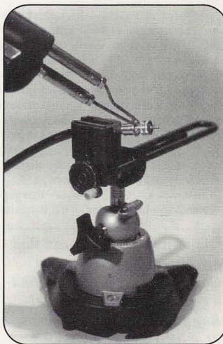
A Panavise unit holds larger jobs to make soldering easier. Several different heads are available for the unit, including a circuit board holder.
