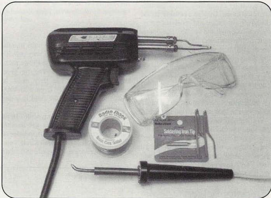
A good basic soldering kit consists of a 100/140-watt gun (upper left), 25-watt pencil (bottom), solder, safety glasses, and spare tips for the gun and pencil. (All photos by the author)
