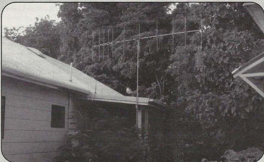
Photo C. Here's what David uses to stay in touch with the mainland—an 11-element 2-meter beam mounted outside his room in the Heron Island staff quarters.
