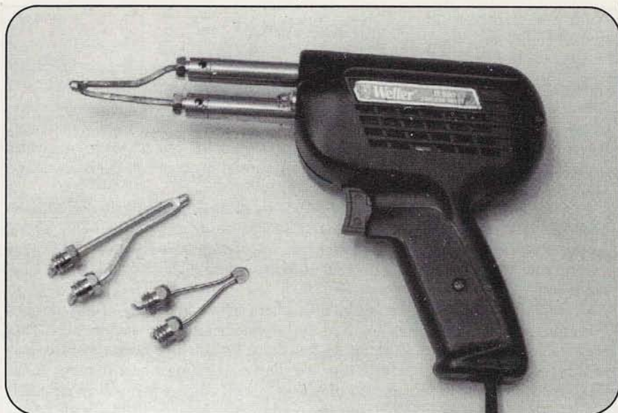
A good, high-wattage solder gun is best for soldering coax connectors and heavy antenna wires. This early version of the Weller D-550 provides an ideal 240/325 watts of heating power for big jobs. Current models provide 200/260 watts and are still adequate for this work.
