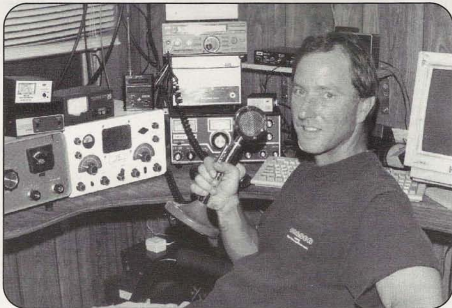
The author at his station in Santa Clarita, California. The radio with the white faceplate and black dials is a Gonset G-50 AM transceiver. To its right (behind the Astatic D-104 "lollipop" mic) is a Swan 250 SSB rig, both for 6-meters. (WA6ITF photo)
