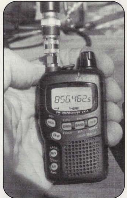
The Yaesu VX-1R dual-band handheld is smaller than palm-sized, but it's packed with features including full 430- to 450-MHz transmit coverage on 70 centimeters, and reception capabilities from the AM broadcast band to 999 MHz, including the 856-MHz public service band shown here. See Table for details of frequency coverage.
