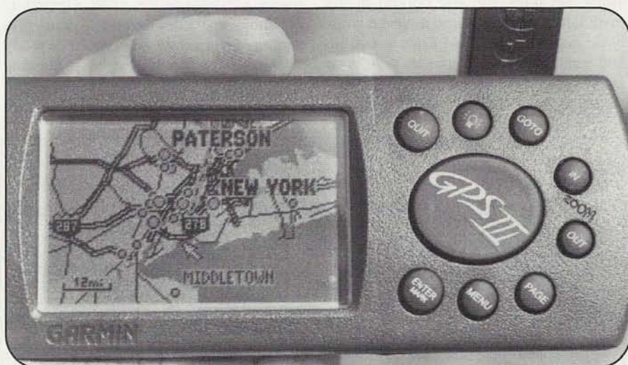
Built-in map data sets apart Garmin's new GPS-III Global Positioning System receiver from everything else in its price class. You can zoom in and out for varying levels of detail. The handheld unit includes map data for all of North America. (WB6NOA photos)
