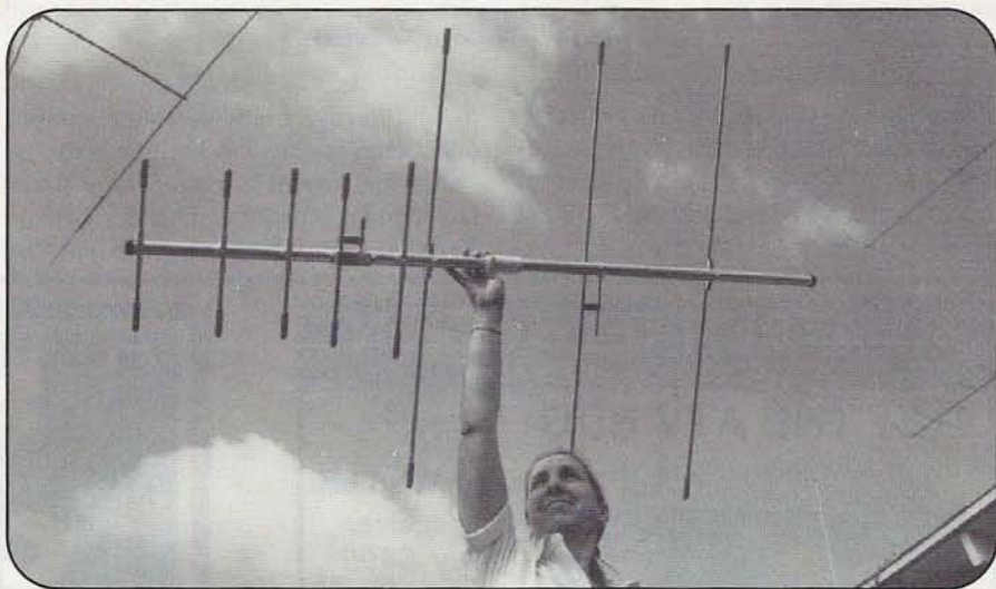
The Comet CYA-240 Yagi antenna goes together in about 20 minutes and weighs less than 5 pounds. Note that the 2-meter elements are at the back of the boom and the 70-centimeter elements are mounted separately at the front end. That's Gordon's wife, Suzy, N6GLF, showing you how light the antenna is. (All photos by the author).
