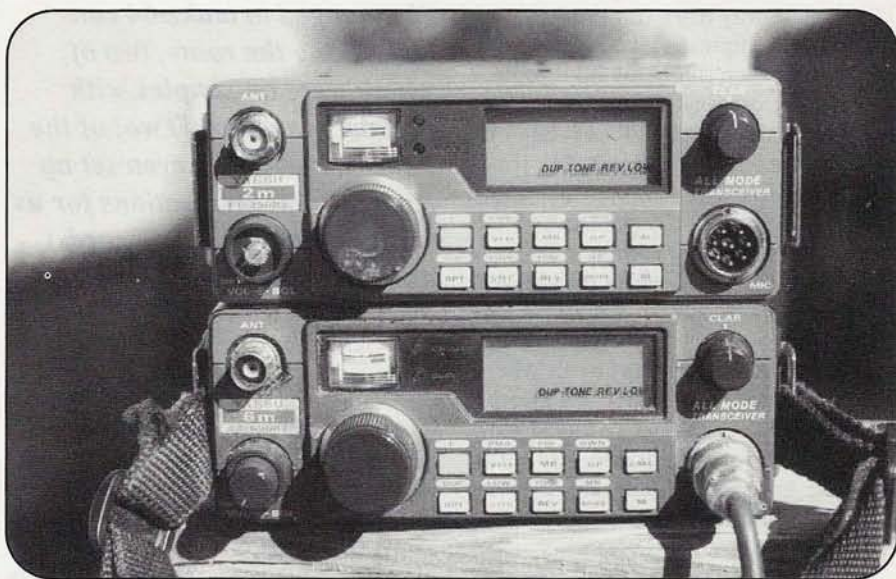
Photo A. This is not a pretty picture, certainly not the kind you'd see in an advertisement. The FT-290 and FT-690 shown here are two war-horses from WB2AMU's personal collection and they've both seen a lot of mileage from numerous portable and mobile operations, particularly during VHF contests and Field Day. (Photos by the author)
