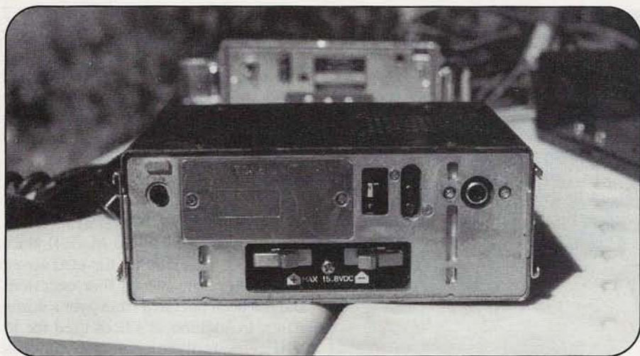
Photo C. The back end of the front section of the radio. Here's where you connect either the battery pack or the linear amplifier. An optional tone unit can be installed in the compartment on the upper left. Plugging in an amplifier instead of the battery pack also deactivates the antenna jack on the front panel (there's an SO-239 output jack from the amplifier).
