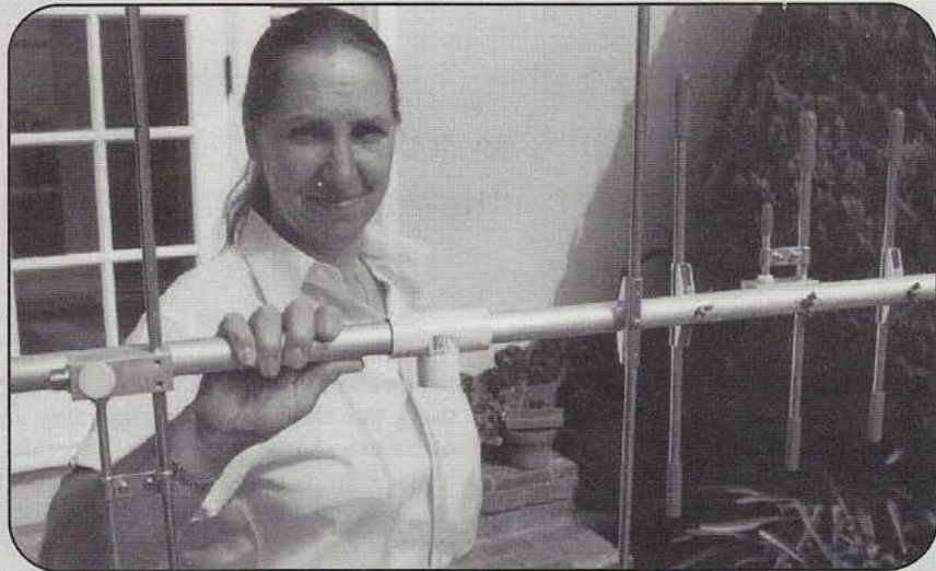
N6GLF holds up the antenna as modified by WB6NOA. The PVC "tee" in the middle of the 2-meter section (see text for exact location) makes field mounting easier than the factory-supplied rear mount with heavy stainless steel hardware.
