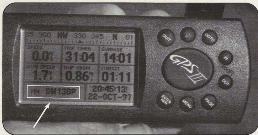
If you're buying a GPS receiver mostly for VHF ham use, be sure to get one that offers a direct readout of Maidenhead grid squares, such as DM13bp, shown here.
