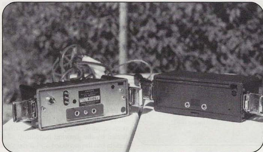
Photo B. On the left is the 10-watt linear amplifier back end for the FT-690; on the right is the 2.5-watt battery pack that can attach to any of the Yaesu VHF portable units. Either assembly clips on easily and quickly to the front end of the unit.
