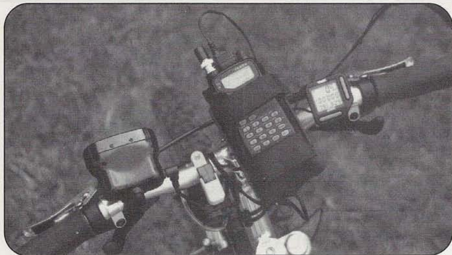
Detail of the author's hi-tech handlebars. To the left of the HT is his 115-dB air horn, and over on the right is his "Radar cyclocomputer," which reads out more information than most automobile dashboards.
