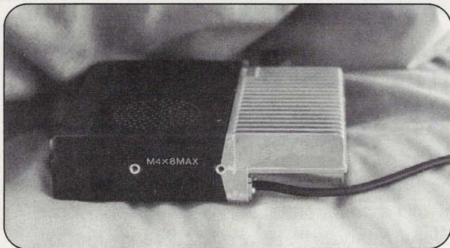
Photo E. Half of the TM-261A is heatsink (the fins on the right) and even that's not enough to keep the radio from getting very hot to the touch after extended operating at high power. The black cable at the right front is the coax "pigtail" to which your antenna feedline gets connected. Be careful to keep it relatively straight and away from the hot fins of the heat sink.
