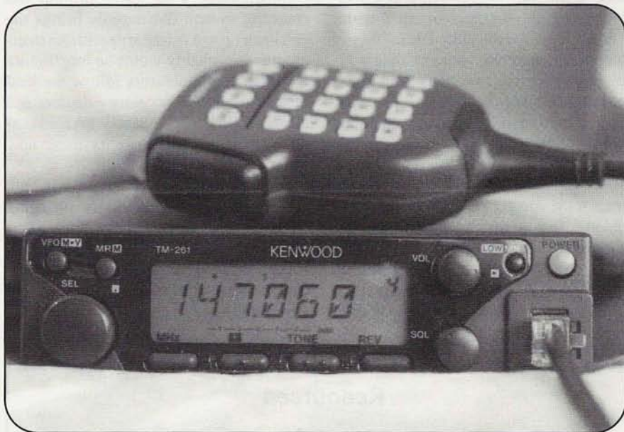
Photo A. The Kenwood TM-261A features 50 watts of output power, more than 60 memories, intuitive programming, and an easy-to-read backlit LCD display.
