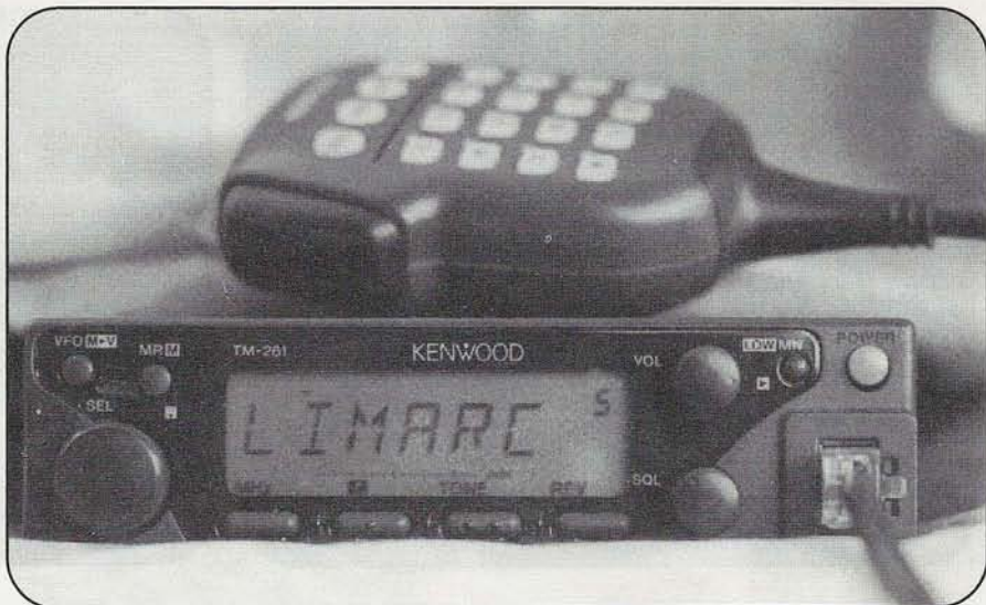
Photo D. Alphanumeric labeling of memory channels lets you put in a club name, location, or whatever else you can say in six letters/numbers instead of the frequency readout.
