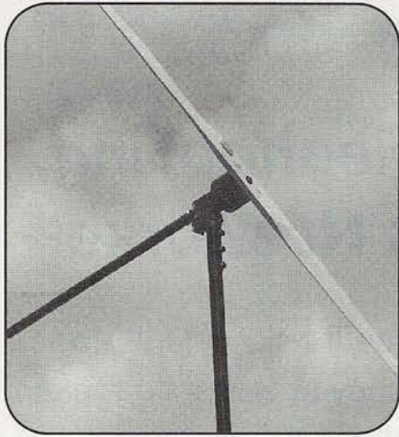
Photo D. Have you ever considered powering your big rig or entire house by alternative energy? A few large solar panels and a wind generator, like the "Whisper" unit shown here, plus a hefty charge controller, inverter, and battery bank will do the job! (Photo courtesy Alternative Energy Engineering)
