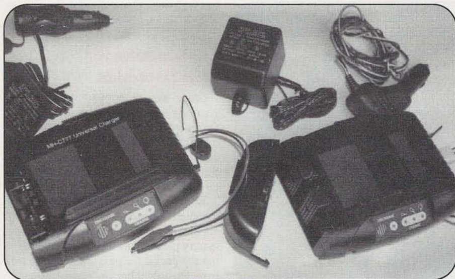
While the Maha (left) and Periphex (right) "universal chargers" look identical and will each safely charge just about any type of NiMH or NiCd battery, there are minor differences in the circuitry. See text for details.
