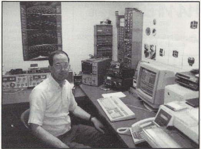
Down Under—Rich Burgan, WC8J, operates a satellite station from the basement of his home in Akron, Ohio. A basement shack requires longer runs of feedline than an attic station, but, on the other hand, it's more convenient for installing a good RF ground (see text).
