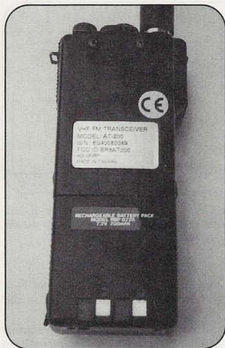
Photo C. By applying simple mathematical calculations to a battery pack's marked voltage and current ratings, a variety of charge times and current rates can be determined. You then use these figures to determine the specifics of the solar charger you can build based on this article.
