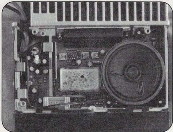
Photo B. Top interior view of the TM-261A. Note the neat and uncluttered parts layout, which will make servicing easier.
