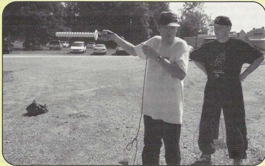
Now, this is Kent Britain, WA5VJB, testing the gain of a W6OAL 15-turn microwave helix at the 1997 Central States VHF Society Conference antenna range. In case you’re wondering, the gain was +15 dBic (decibels over isotropic, with the “c” noting that it’s circular).
