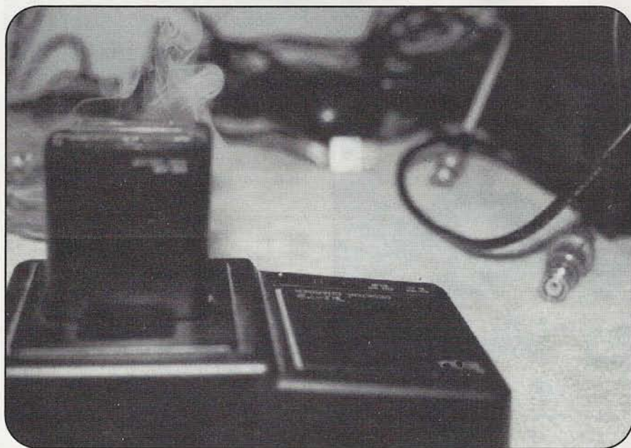
Putting an NiMH battery pack in a fast-charger designed for NiCd cells can have unplanned consequences—such as setting off your smoke detector! (Photos by the author)
