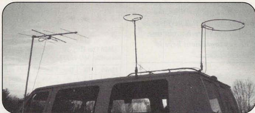
Photo F. While they're less than ideal for SSB work, vertical whip antennas (seen in between the horizontal ones here) can still get you on the air with a decent talk range.
