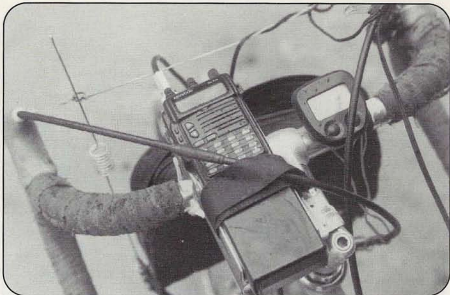
AA6WK's "operating position." The HT is strapped into an old headlight mount, and an external push-to-talk switch is mounted to the handlebars (not visible in photo).
