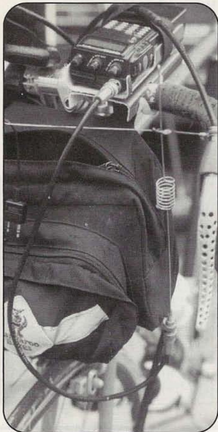
Detail of AA6WK's bike-mobile antenna. Note the string about \frac{3}{4} of the way up—it stretches from one brake lever to the other and keeps the antenna stable on even the bumpiest roads or trails.
