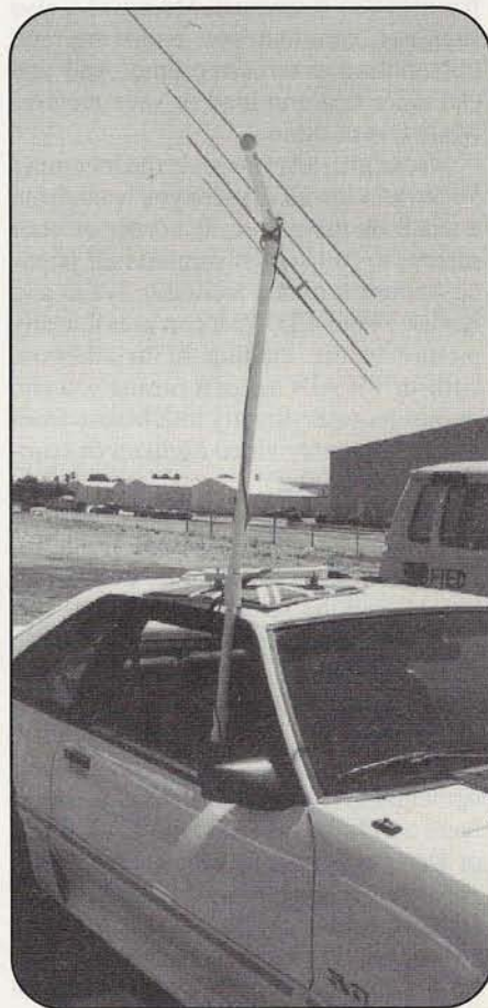
Photo A. A rotating 2-meter Yagi in a support made from ordinary PVC sprinkler pipe can get you started in mobile T-hunting within one afternoon.
