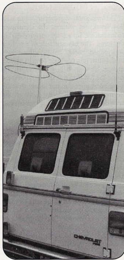
The Laddy Cloverleaf—a modern version of the Big Wheel antennas from the past—came in 1 S-unit higher than the smaller single loops. It also takes up much more space.
