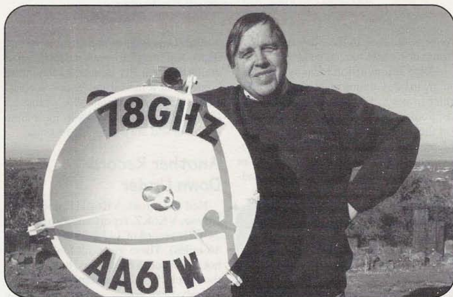
Photo A. Lars Karlson, AA6IW, and his 18-inch dish for 78 GHz. Lars and Will Jensby, WØEOM, set a new U.S. record for the band last December by making contact over a 7.6-mile path.
