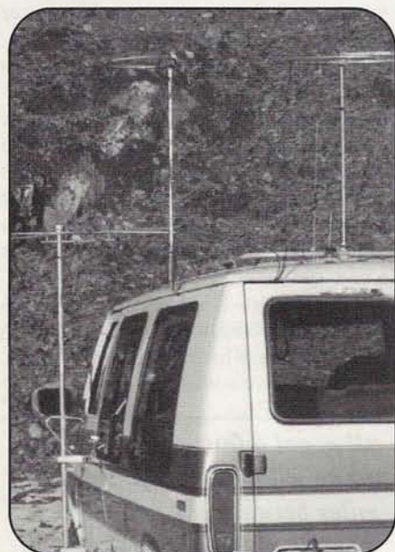
A two-band mobile setup with omnidirectional halo antennas for 6 and 2 meters (the bigger one is for six), plus a 2-meter beam for distance.
