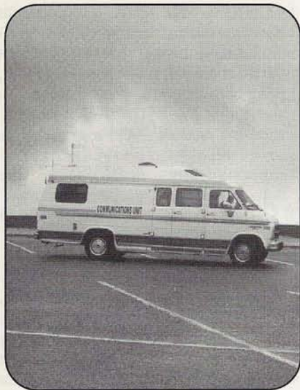
The test course was an empty parking lot overlooking the Pacific Ocean. The lack of nearby cars and buildings minimized reflections that might have skewed the readings.
