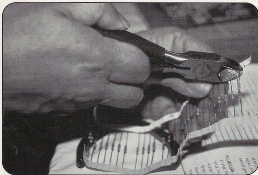
Photo C. One of the "niceties" of Heathkits was that parts such as resistors were taped together in the order in which you'd be using them. This minimized the chances for errors or lost parts.
