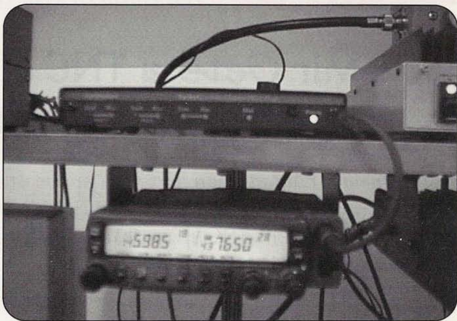
Closeup view of the KPC-9612 Plus TNC (above the radio). If you want to see it now, you'll have to visit Mir...or Moscow. An identical twin is set up at the Russian space agency.
