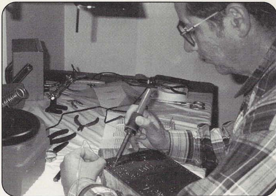
Photo D. Soldering the circuit board is an exacting process, but it was a lot easier to work on the Heathkit board from the early '80s, which was designed for discrete components and normal-sized fingers, than on one of today's super-tiny surface-mount boards.
