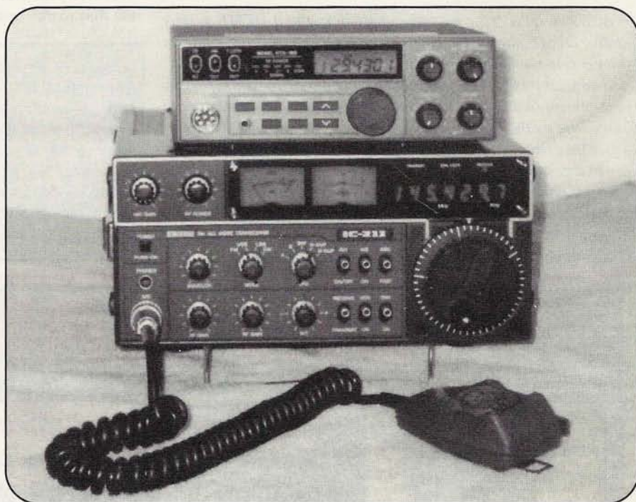
Photo A. Mode A Satellite Station made of an ICOM IC-211 and a Realistic HTX-100. (The IC-211 is now a proud part of KB2YJH's Satellite Station.)
