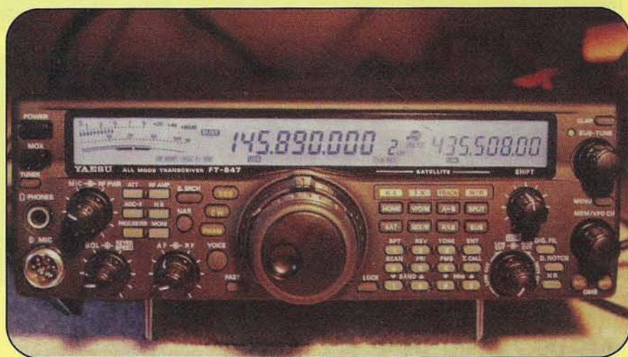
Photo A. The compact FT-847 is the first commercially made radio to operate from 160 meters to 70 centimeters without the need for add-on modules. It offers 100 watts out on HF and 6 meters and 50 watts out on 2 meters and 70 centimeters. (WB6NOA Photo)
