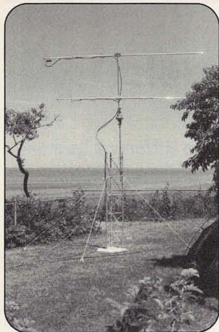
These are the 2-meter and 70-centimeter multi-element arrays with Long Island Sound in the background. Connecticut and Rhode Island were within reasonable reach of all of the VHF stations.
