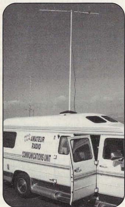
Add a small antenna, such as this Maspro 2-meter Yagi, and you're on the air with a 20-foot mast from any place you can reach by car.
