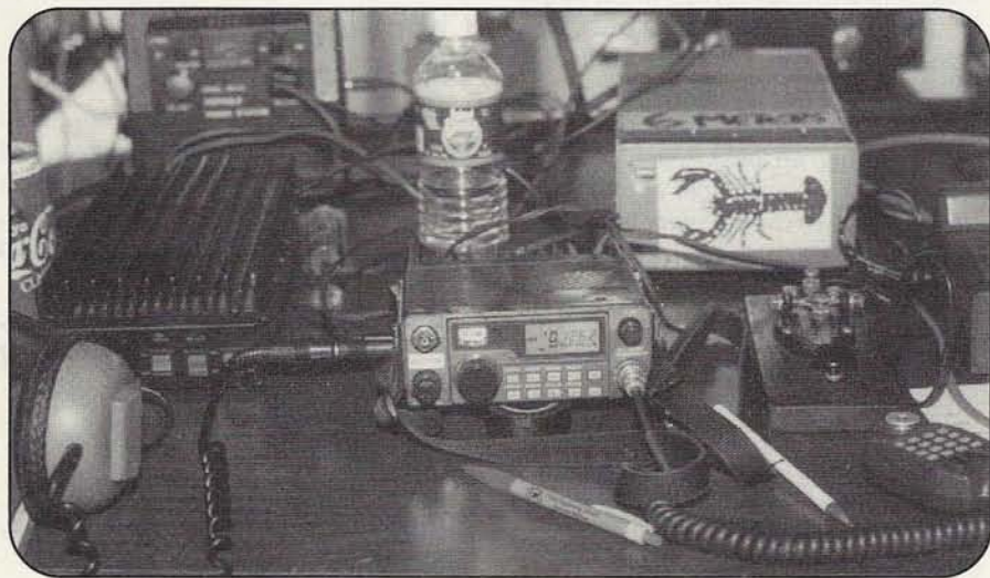
Close-up of the Peconic ARC 6-meter Field Day station. The FT-690 puts out 10 watts and is fed into a Mirage linear amplifier (left) for 150 watts output. Most 6-meter contacts were on SSB with some on CW and FM as well.
