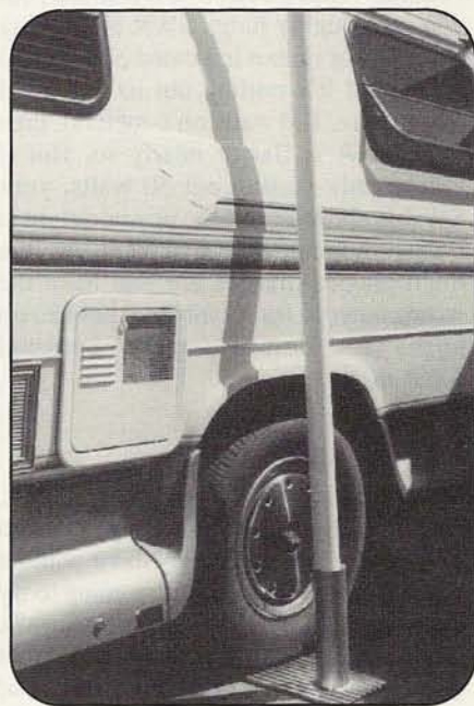
Here's the collapsed flagpole/mast anchored in the wheel plate, ready to be telescoped upward. The collapsed length is 90 inches.
