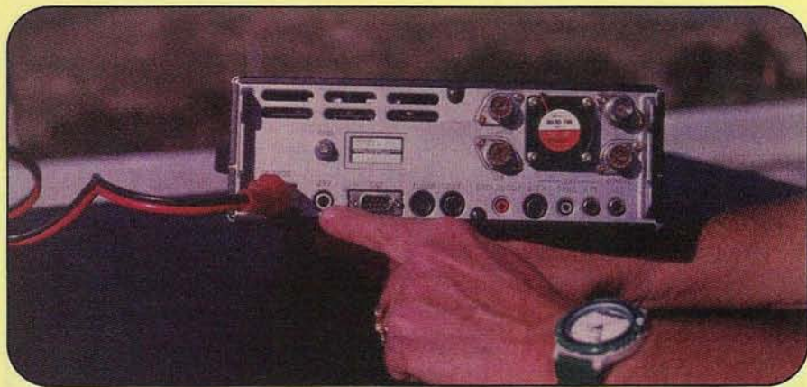
Photo B. There are four separate antenna jacks on the back of the radio: one each for HF, 6 meters, 2 meters, and 70 centimeters. In the photo, Gordon is pointing to the computer control jack that allows the FT-847 to be used as a remote base. (K7JA photo)
