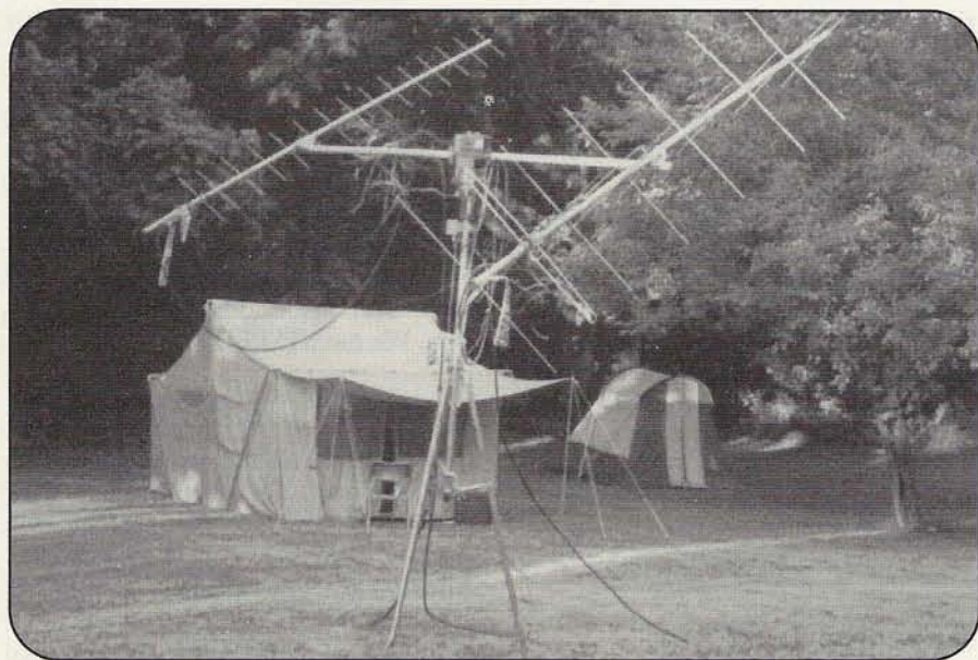
Photo B. The WA2PNU Satellite Antenna System Mounted on its Tripod Tower. See text for details.
