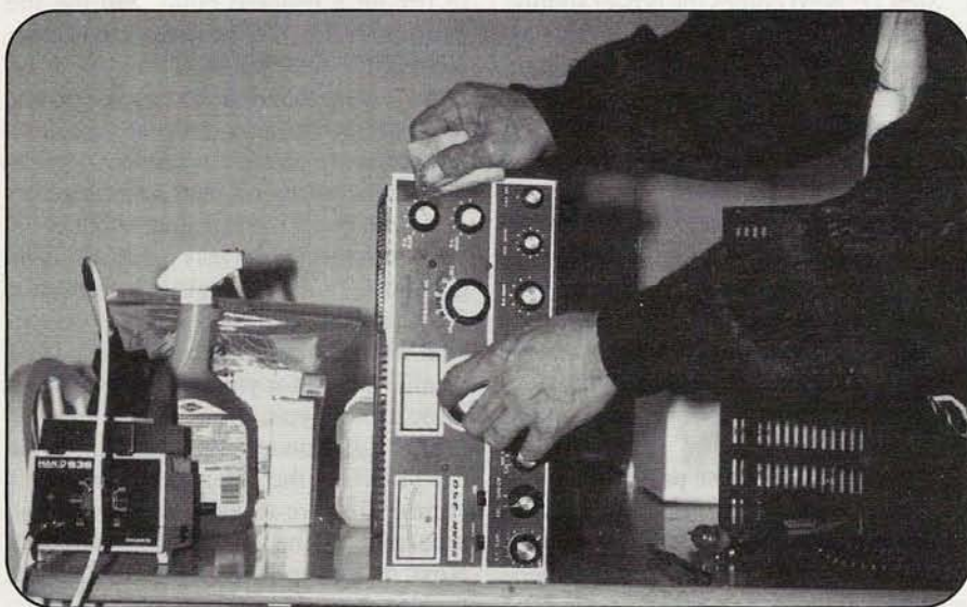
Photo C. Next, remove and set aside tubes and relay covers. Knobs also need to be removed and cleaned in a solution of dishwashing detergent and water (see text for details).
