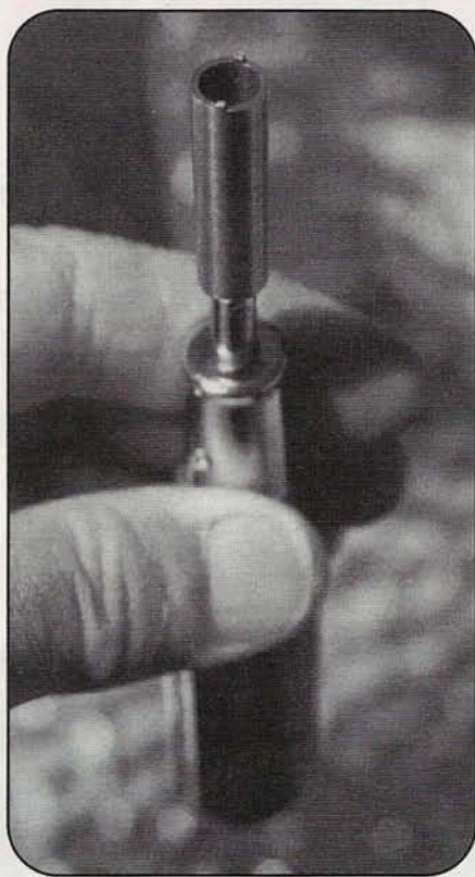
Photo E. Opening up the case on the T8A requires removing the collar on the SMA antenna connector. And that requires this special tool, called an "L2." They're used widely in the auto stereo industry.
