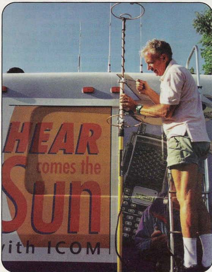
Photo B. Gordon West, WB6NOA, installs a pair of KB6KQ Superloop 2-meter SSB antennas on the ICOM Fun Mobile.
