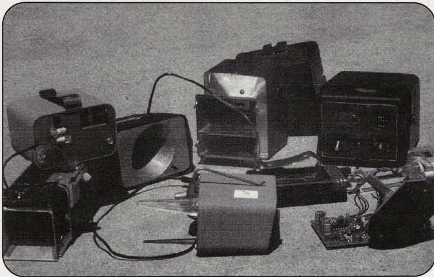
Photo A. Switched-diode radar detectors. These are some of the few that Kent hasn't already cannibalized for other microwave projects.
