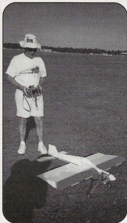
The pre-flight checkup includes tests to make sure every system on the airplane is working properly and will respond to commands from the ground. While Sandy is not a ham, there are hams who enjoy R/C flying, and a portion of the 6-meter band is devoted to "radio remote control."
