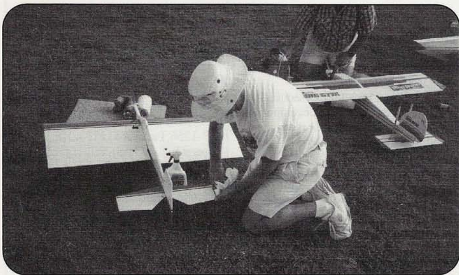
Post-flight cleanup and inspection. After each flight, you need to check for damage and give the plane a thorough cleaning to remove any oil, exhaust residue, and bug remains.
