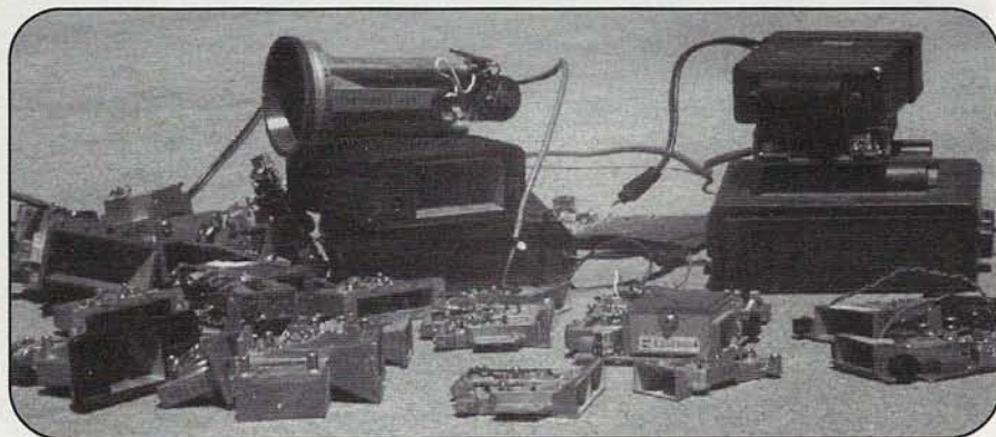
Photo C. Kent hasn't made as much progress yet in cannibalizing his collection of superhet radar detectors. You can find your own at fleamarkets for $5 or less. In most cases, says Kent, the microwave part of the unit works even if the rest of it doesn't!
