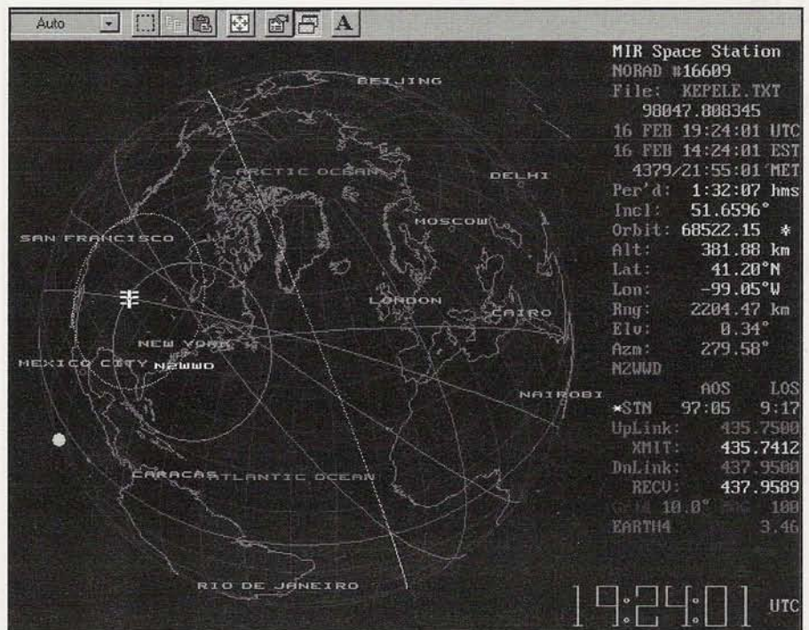
Figure 1. The orthographic projection, or globe display, produced by STSPLUS. This is kind of a "satellite's eye view" of the planet. The circle around the satellite (Mir, in this case) indicates the area within its "view" at any given moment.
