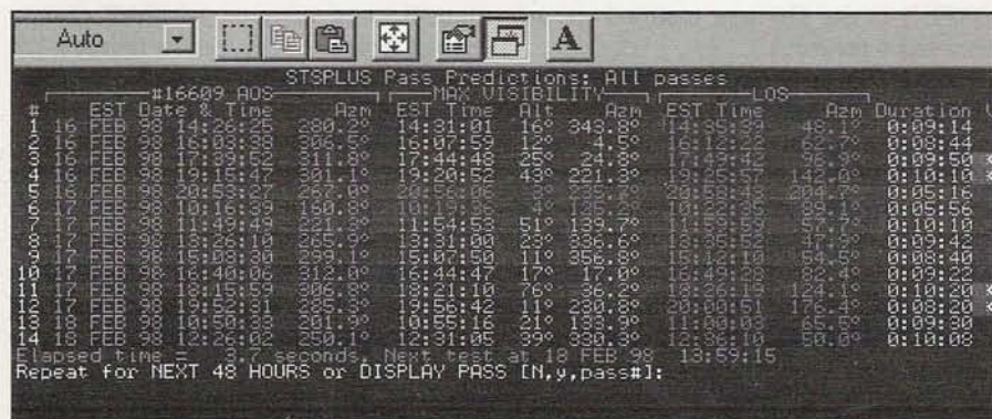
Figure 3. A text version of STSPLUS's satellite pass predictions. This is known as a Tabular Line-of-Sight screen, showing all predicted passes of a selected satellite during a given time period. Each line provides information on the beginning (AOS) and end (LOS) of each pass, plus the period of "maximum visibility."
