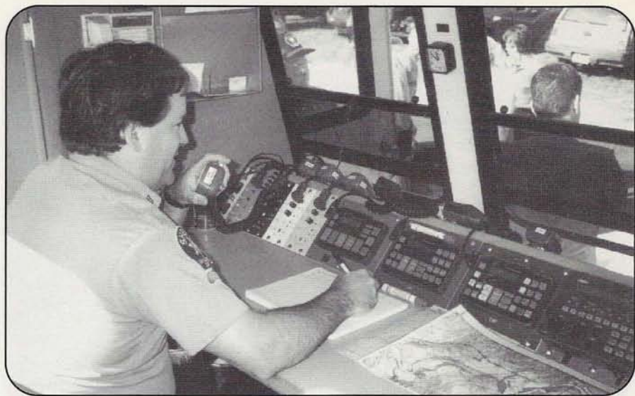
Bob Stadtherr, KI6WO, dispatching from the SLOSAR communications van. The van is able to simultaneously monitor and communicate on all police, fire, aircraft, and amateur frequencies in use for a search and rescue mission.
