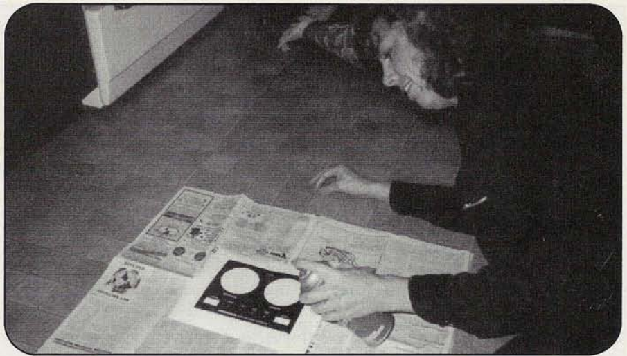
Photo B. After printing out the label, you will need to spray the front of it with several coats of clear lacquer finish. Make sure you have good ventilation when you're spraying.
