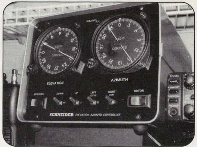
Photo E. Here's the finished label glued to the panel. The meters and switches are installed and the front panel is mounted in the case.
