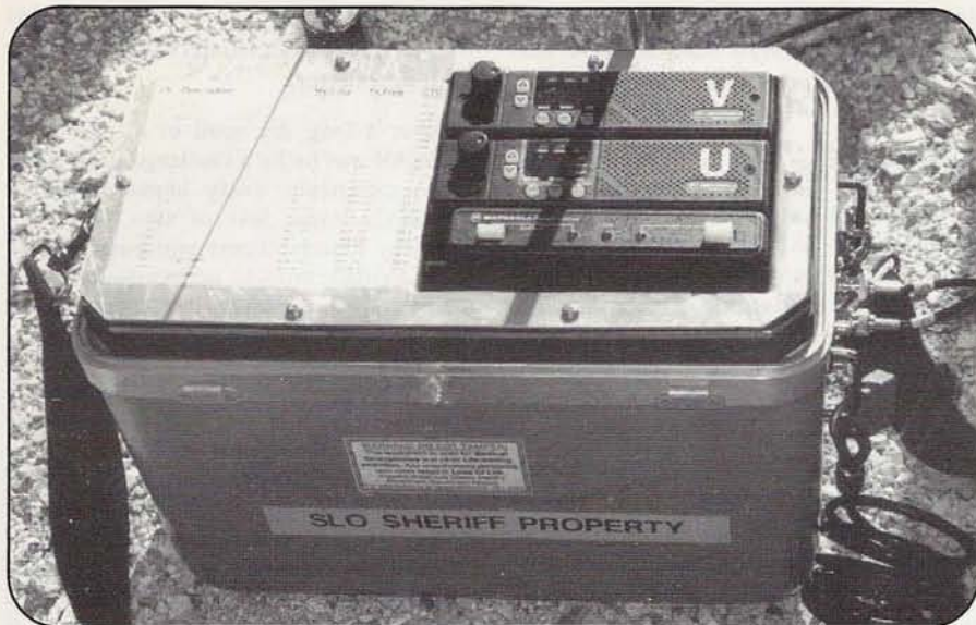
The SLOSAR portable cross-band repeater. This operates on VHF and UHF public service frequencies used by the SAR teams.
