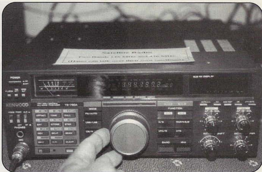
The big tuning knob can be switched between free-spinning for USB/CW contacts or satellite work to a “stepped” control, complete with clicks, for FM operation.
