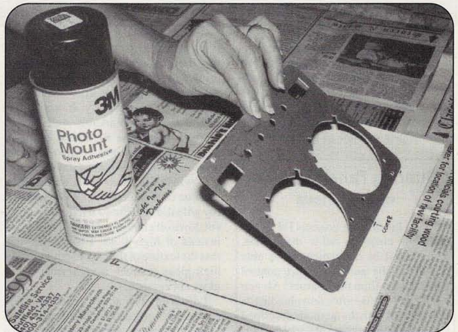
Photo C. Here, the label is now lying facedown with adhesive already sprayed on the back. The metal panel, with holes cut out, is lined up on the marks and is being lowered onto the sticky label.
