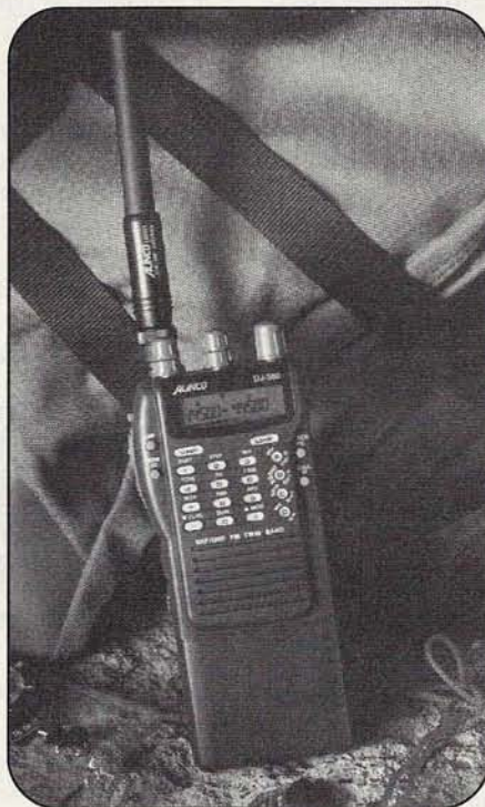
Photo A. Close investigation of an FM rig's keypad usually reveals its toning capabilities. The secondary function of this Alinco DJ-580's "6" button, for example, operates its CTCSS decoder and the secondary function of its "B" button operates the rig's DTMF/DSQ paging system. (Photo courtesy Alinco)
