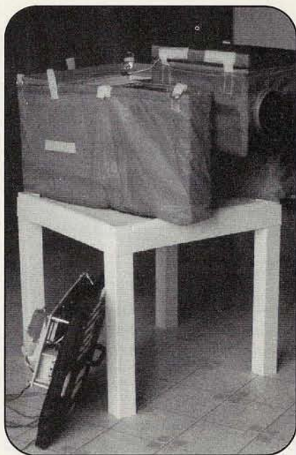
Photo F. The "Sagan," first of two new KNSP projects for 1998. This capsule is designed specifically for carrying a camcorder into near space, and providing great flexibility in aiming the camera lens.
