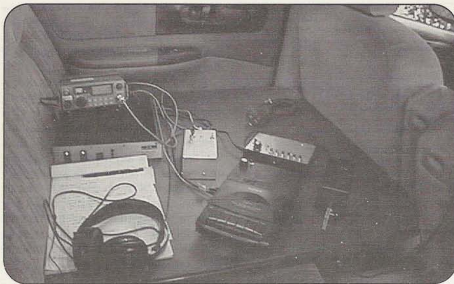
Photo C. Simple HSCW contest setup in the back seat of the author's car. CMOS Super Keyer III is behind the Modified Tape Recorder (MTR) and homemade paddles are to the right. Rig and amp are to the left, with switchbox in the middle.
