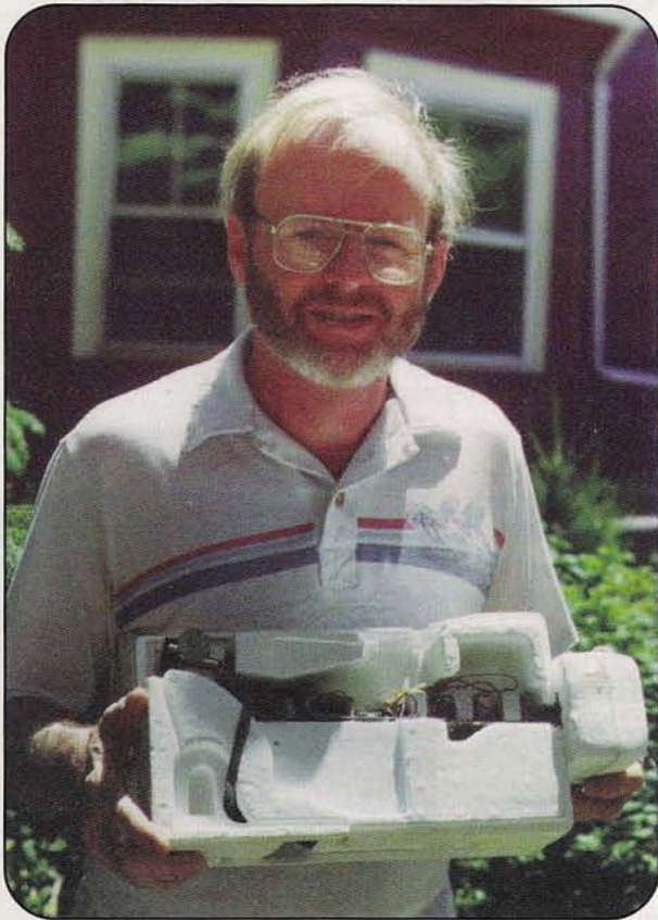
Photo A. Hank Riley, NILTV, holds the "hamradiosonde" launched in Massachusetts on May 30. Components, from left to right, are the altimeter, microcontroller, tone generator, and 2-meter transmitter. (Photo by Mike Riley, W1AQS, courtesy NILTV)
