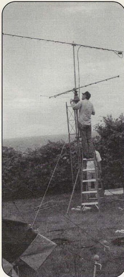
Six meters wasn't the only VHF/UHF band on the air at W2AMC. Here, Peconic ARC "Technical Maven" Charlie Burnham, K2GLP, is setting up Yagis for 2 meters and 70 centimeters, making sure the three major VHF-plus bands were available for FD contacts.
