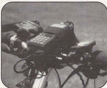
The battery switch can be housed in something similar to the author's Velcro® HT holder. In this photo, you can see the switch mounted below the HT, providing easy access for switching from low to high power.
