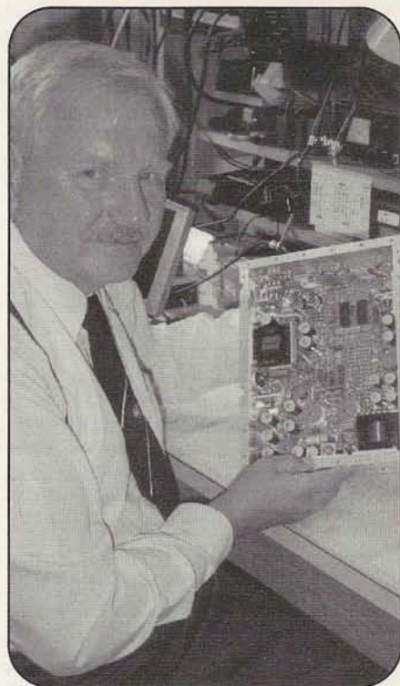
Dr. Andras Gschwindt, HA4WH, holds the P3D Battery Charge Regulator (BCR), built by a team he led at the Technical University of Budapest, Hungary. The BCR will control the power to all components of the spacecraft.
