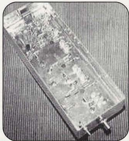
Photo C. Another option for a local oscillator is the G4DDK DDK004 board. This would have to be modified to produce a signal on the correct frequency for the 'WDG transverter, but the transverter manual includes instructions for making the mods.
