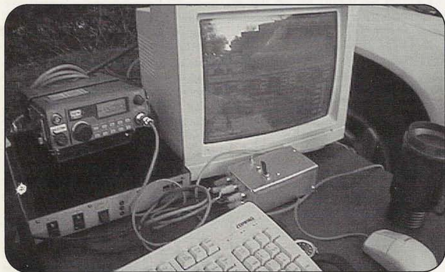
Photo D. A sunrise behind you will sure make it hard to see a computer monitor! Displayed on the screen is the popular HSCW software, MSDSP, by 9A4GL. To the left is a Yaesu FT290 transceiver stacked on top of a TE Systems amp. Chassis box in the middle is a simple homebrew switchbox to handle the PTT line by either a toggle switch or VOX control.
