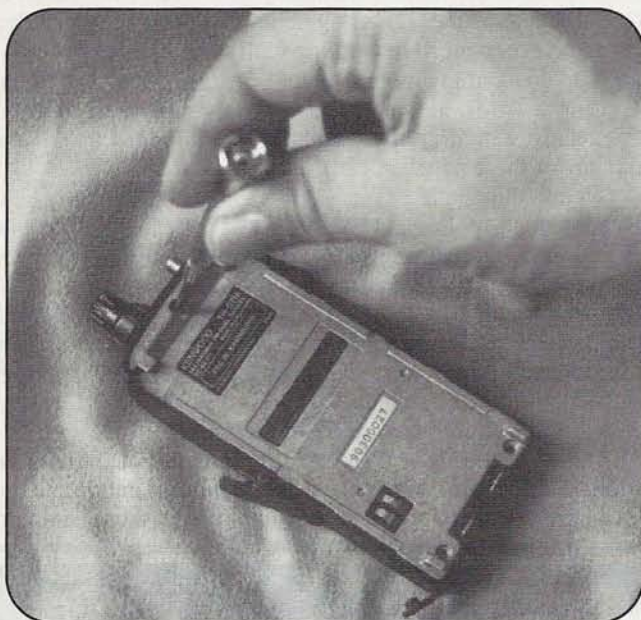
Photo C. To make the extended-frequency modifications to the TH-G71 (see text), you start by removing the battery pack and antenna, opening the rubber covers for external jacks, and removing the tiny screws holding on the radio's back plate.
