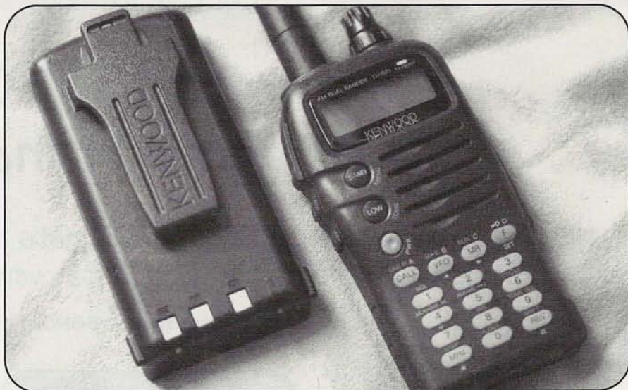
Photo B. The battery pack makes up half the size of the TH-G71, as is the case with many of today's HTs. Putting the belt clip on the back of the battery pack, though, makes quick-changing batteries in the field inconvenient, unless you're ready to buy a belt clip for each battery pack.
