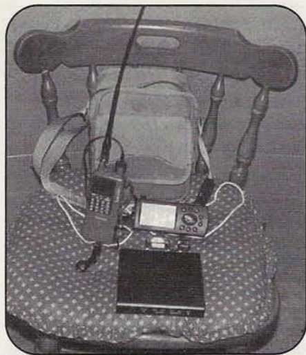
The totally portable APRS Tracker station assembled by Herb Gerhardt, KB7UVC. The HT, GPS receiver, and TNC can all be packed into the camera bag in the rear of the photo. (KB7UVC photo)
