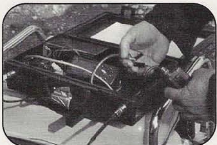
A typical APRS Tracker unit—this one put together by Michael Colyar, K7ITL—with HT, GPS receiver, and TNC in an equipment case, with external connectors for GPS and 2-meter antennas. (KC7NUD photo)
