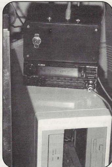
The author's interface board (in the black box at top of photo) connects his Internet link with a local repeater by feeding audio between a VHF/UHF radio (center) and his soundboard-equipped computer (bottom). The UHF section of the radio is used for the control link that can remotely turn the unit on or off.
