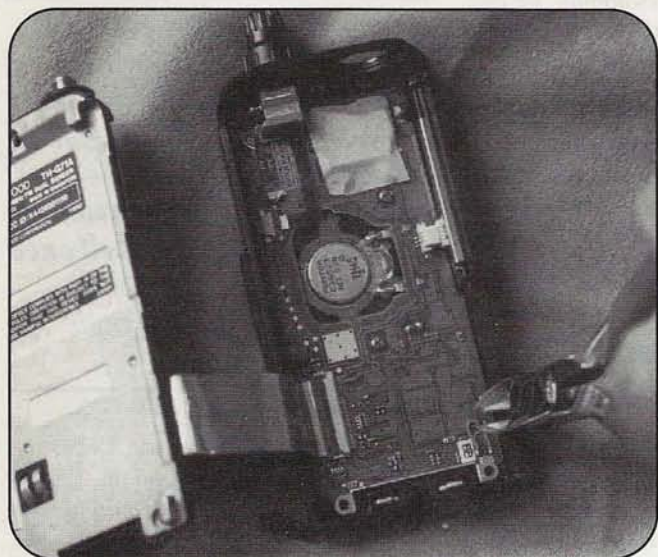
Photo F. To make only the MARS/CAP modification, opening both transmit and receive coverage to either side of the ham bands, simply snip the green wire with a pair of wire-cutters. But be sure to read about all of the mods before making this one.
