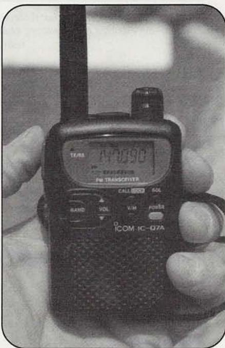
*The ICOM IC-Q7A is tiny enough to fit in the palm of your hand, but offers full transceive capabilities on 144 to 148 and 440 to 450 MHz, plus broadband receive from 30 to 1300 MHz (minus cellphone frequencies).*
