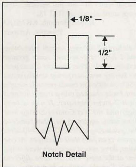
Figure 2. Detail of notch to be cut into one end of parts A, B, D, E, and G in Figure 1. These notches will hold the quad elements and the support cable in place.
