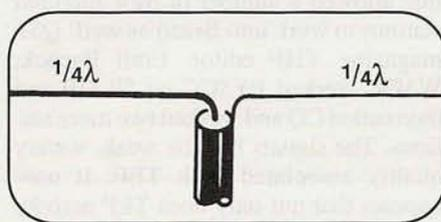
Figure 1. A half-wave dipole is the simplest of antennas, with a quarter-wavelength ( $\lambda$ ) element attached to each side of a piece of coax. Mount it to any convenient non-metallic surface at least six or eight inches away from any metal objects. See the Table for sample element lengths.
