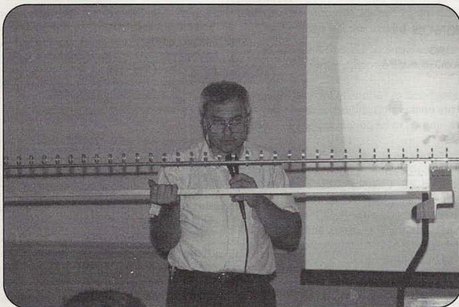
Photo F. Dave Olean, K1WHS, holds up one of his "blowtorch" antennas—mega-wavelength loop Yagis for the microwave ham bands.
