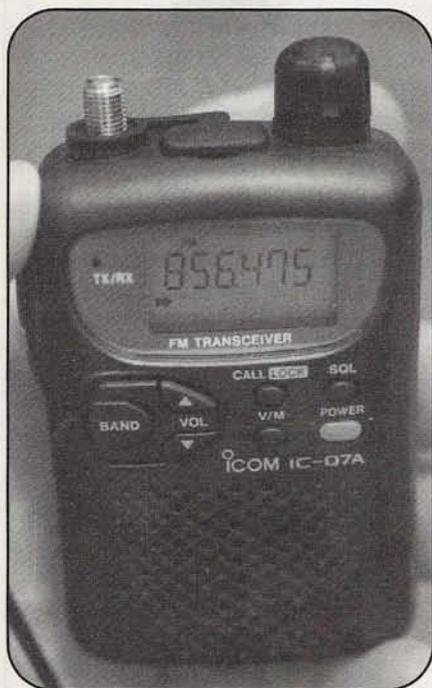
The antenna connector on the IC-Q7A is the SMA style, and the supplied "duck" is so big in comparison to the radio that it often falls over when you try to stand it up! The 856-MHz frequency on the readout is typical of the many public service frequencies you can monitor on this versatile HT.
