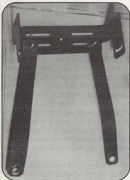
Photo C. Under-seat mounting bracket for the C5718DA. The author attached two aluminum strips to the mobile mounting bracket on one end and to the bolts holding the front passenger seat to the floor on the other end. This not only anchors the radio under the seat, but also assures a solid ground connection for the rig.
