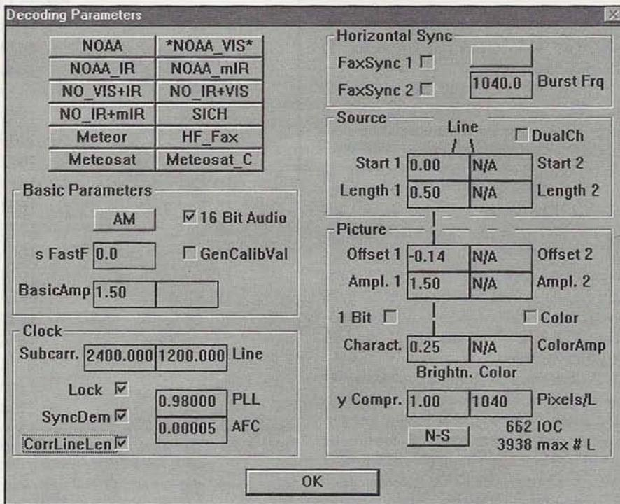
Figure 1. WX-SAT image decoding Parameters. This example is set up for capturing visible wavelength pictures from an NOAA satellite.
