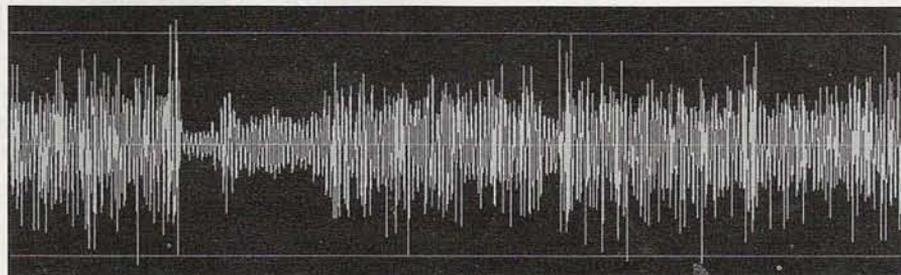
Figure 2. The WX-SAT Test tool. Use this to set the audio peaks so the largest ones go past the gray lines (as shown), but do not clip beyond the borders.
