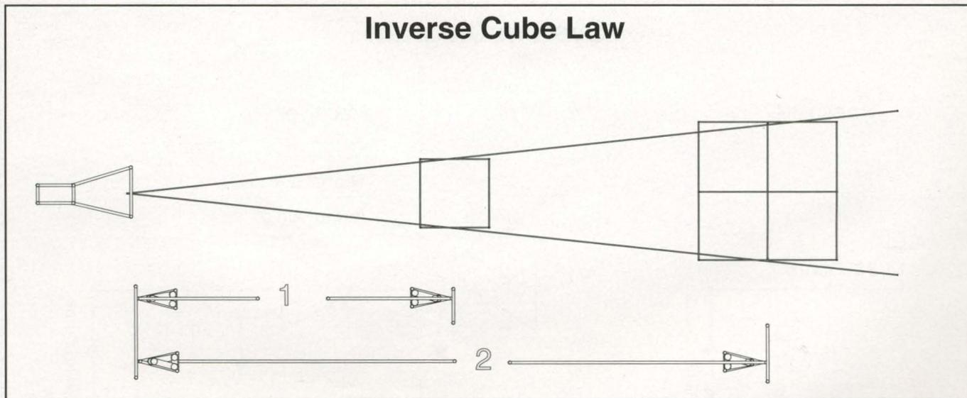
Figure 4. An illustration of the Inverse Cube Law. As a signal doubles its distance from its source, it doubles in both height and width, making the signal at the twice-as-far point only  $1/4$  as strong as the first point of measurement. If it's then reflected back to the source, it arrives with only  $1/16$  the strength with which it left.
