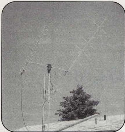
Photo C. Circularly polarized beam antennas for 2 meters and 70 centimeters are a sure sign of a nearby OSCAR satellite enthusiast. The combo shown here belongs to Bill Braithwaite, W4NML, in Idaho and has a nice clear sky view for top performance.
