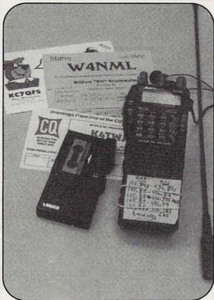
Photo B. Equipment comprising K4TWJ's QRP satellite station includes an Alinco DJ-580 2-meter/70-centimeter FM talkie, a Premier RD-78 dual-band whip, earphones/earbuds, and tape recorder for no-fumble logging. Note frequency relationship chart rubber-banded to rig. QSLs are from a couple of previous AO-27 QSOs.
