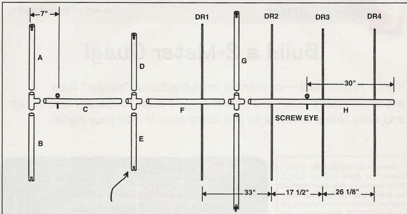
Figure 1. Exploded view of the KI6US Quagi and separation distances for various elements. See the Table for lengths of each of the marked segments. Note that parts D and E, the driven element supports, are shown vertically only for clarity in this illustration. They should be mounted horizontally prior to final gluing.
