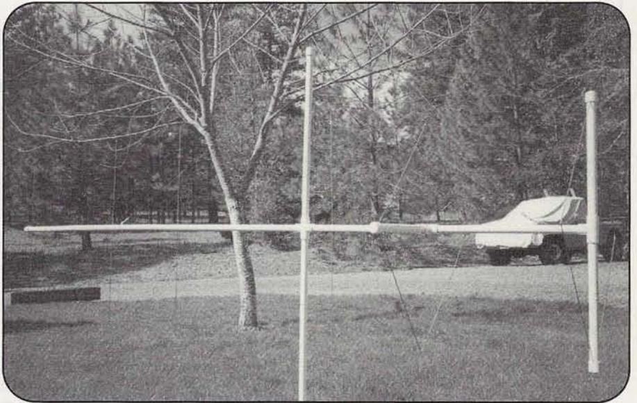
*K16US's assembled Quagi antenna. It'll work better, of course, if you can install it a little bit higher off the ground (but, then again, it's easier to take a picture while standing on the ground than while hanging from a tower!).*
