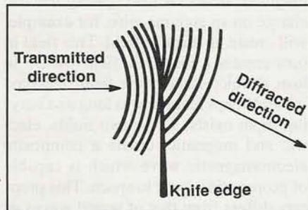
*Figure 1. Long-distance radio communication depends on the deflection of signals that would otherwise be radiated into space. One of the many forms and types of deflection that affects radio signals, knife-edge diffraction, is shown here and explained in the text.*
