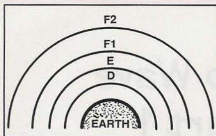
Figure 2. The ionosphere, which is responsible for most long-distance propagation, contains four layers that affect radio signals: D, E, F<sub>1</sub> and F<sub>2</sub>. The role of each layer is explained in the text.
