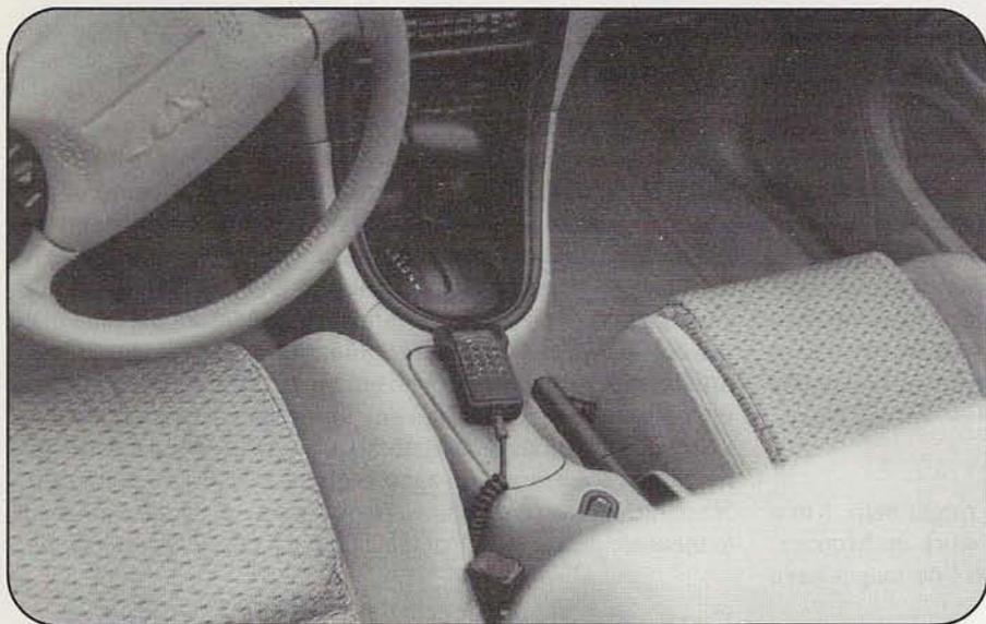
Photo D. All that's visible of the C5718DA in Debbie's car is the speaker/mic/display and a bit of coiled cord—the perfect solution to mounting a radio, with no holes and no wires, in a car with no on- or under-dash mounting space.
