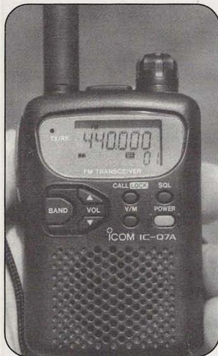
Out of the box, the IC-Q7A won't transmit below 440 MHz, but it can be modified to cover more of the 70-centimeter ham band. Like other micro handhelds, it does not offer a DTMF tone pad for making autopatch calls.
