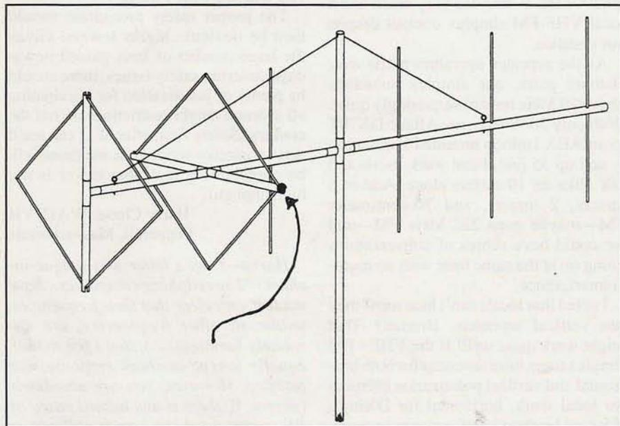
Figure 3. View of the completed Quagi antenna. Note that, in a quad antenna, the coax is fed from the side for vertical polarization, and at the bottom (or top) for horizontal polarization.
