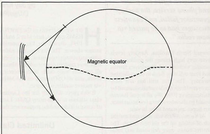
*Transequatorial Propagation (TEP) allows contacts between stations that are equidistant from the magnetic equator, which tends to wander in relation to the geographic equator. Occasional sporadic-E links may make contacts possible over even greater distances.*
