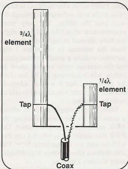
Figure 3. The simple J-pole antenna. The construction material can be any good conductor. See text for details on element spacing and feed systems.
