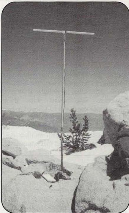
Photo C. AC6XX's portable setup atop San Jacinto Peak: a handheld, a long-life battery, and a home-built three-element Yagi antenna mounted on top of a PVC pipe, which was in turn attached to the author's walking stick.
