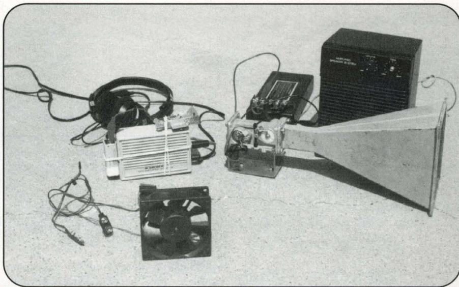
Photo A. Two of the Doppler radar units I've built for demonstrations, along with a muffin fan which I also use in radar demos. Read why in the text. (All photos by the author)
