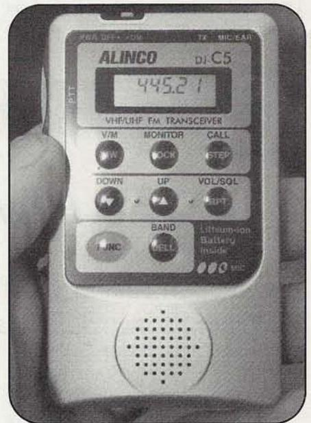
The Alinco DJ-C5T is a credit-card sized dual-band handheld, complete with a built-in speaker and a rechargeable lithium-ion battery. It transmits "out of the box" on 144 to 148 MHz and 420 to 450 MHz, the entire 70-centimeter band. (All photos by the author)
