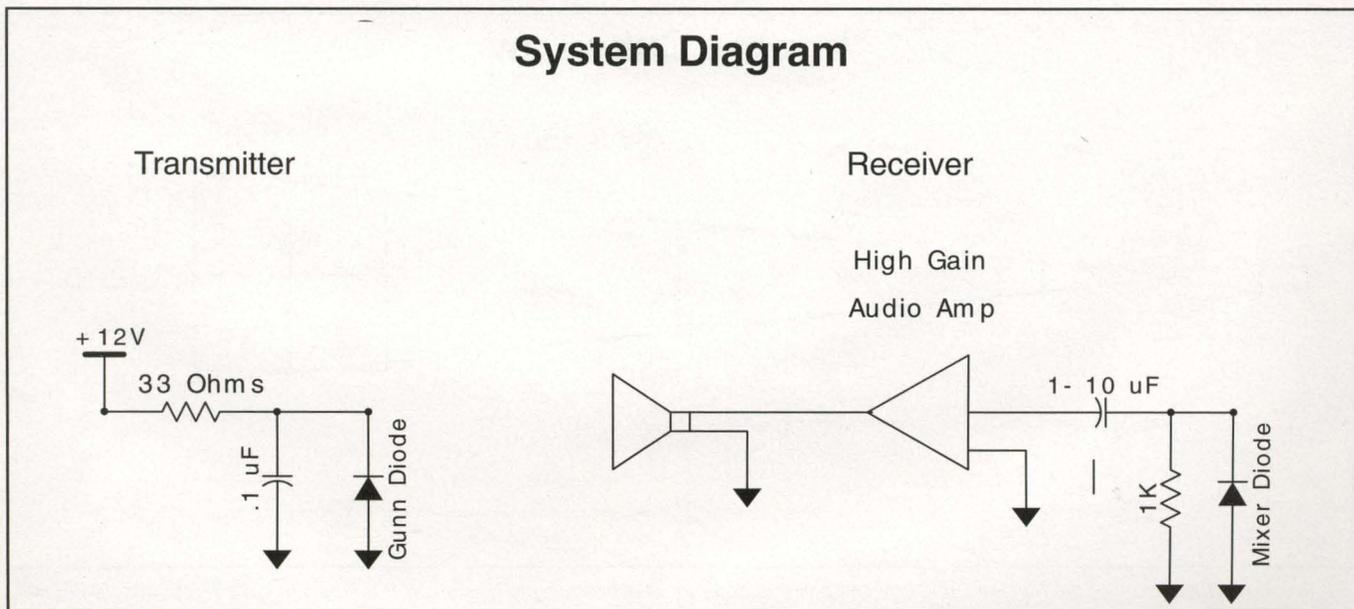
Figure 3. A schematic diagram of a Doppler radar system. None of the component values are critical (see text), so it is really a pretty easy "junkbox" project.
