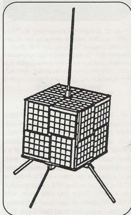
Figure. Line art sketch of AO-27. The little satellite is covered with photocells and is small enough to sit on an auto's rear seat. Sketch courtesy AMSAT.
