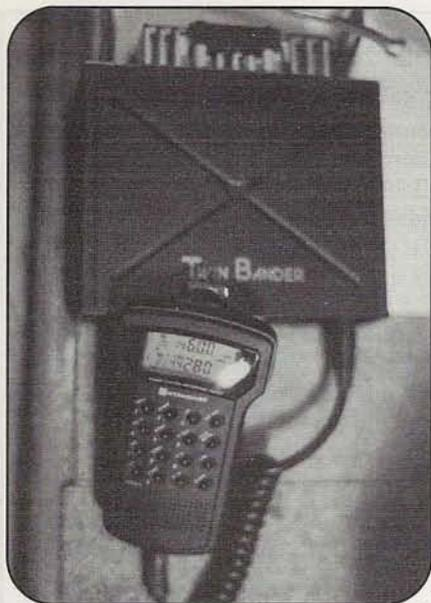
Photo B. The Standard C5718DA has all controls, and even the dual-band frequency read-out, right in the speaker/mic. This enables you to install the main transceiver unit in an out-of-the-way place and still have full control over all functions.
