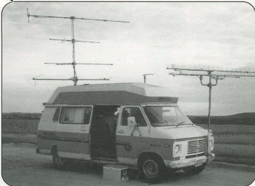
Photo B. WB5VYE's VHF/UHF/microwave rover van. The loop Yagis in front are for the microwave bands.
