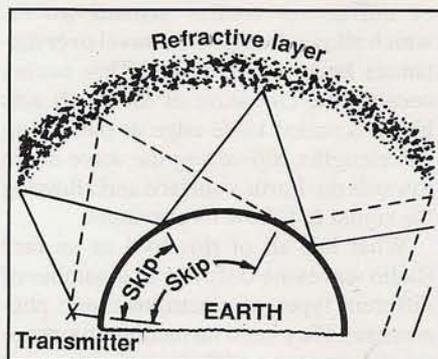
Figure 3. Skywave propagation is the most common means of making long-distance contacts on the HF and low VHF bands. Signals head toward space until hitting a refractive layer that bends them back toward the Earth. The lower the angle of transmission, the greater the distance covered in any one hop, and multiple hops are possible.
