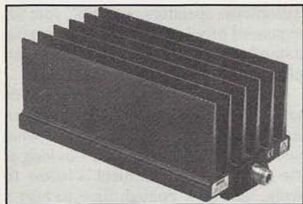
The 500 WT Series are dry, convection-cooled devices that weigh approximately 7.9 pounds. The loads measure approximately 4.3 x 5.4 x 10.38 inches (HWL) and attenuators are approximately 4.3 x 5.4 x 11.2 inches (HWL). The finish is black anodized aluminum. Available tri-alloy plated connectors are IEC 7/16, N or TNC.
