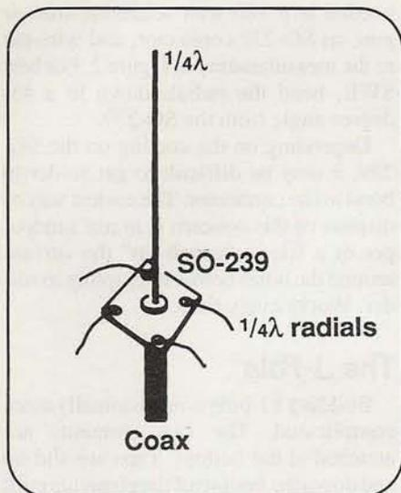
Figure 2. The quarter-wave groundplane antenna using an inverted SO-239 for attaching the elements. Terminate the cable with a garden-variety PL-259 and screw it into the SO-239. The vertical radiator is soldered to the pin that normally accommodates the coax center conductor. Again, see the Table for sample element lengths, and bend the radials down at a 45-degree angle.
