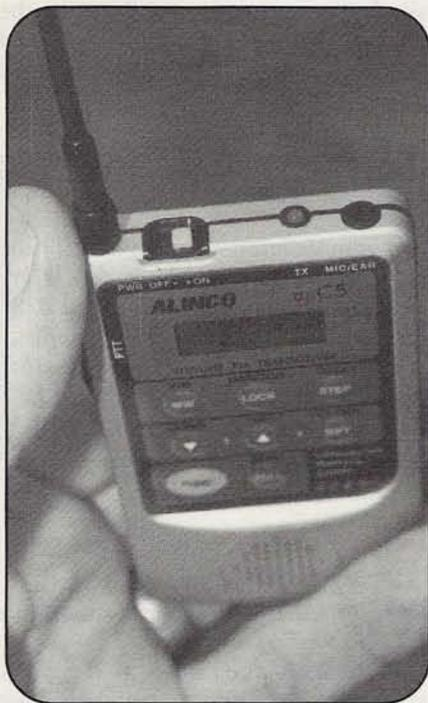
This top view gives you an idea of just how thin the DJ-C5T is—less than a half inch thick! Features on the top include the screw-in antenna, power on-off switch, transmit indicator LED, and socket for an external mic/earphone.
