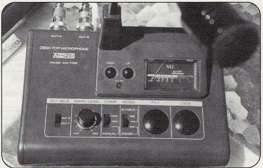
Photo D. The Model AM-708 is the "little brother" to the 7500 and doesn't have the built-in equalizer. However, it does have a dual output, letting you hook up to two rigs at once and simply switch between them.
