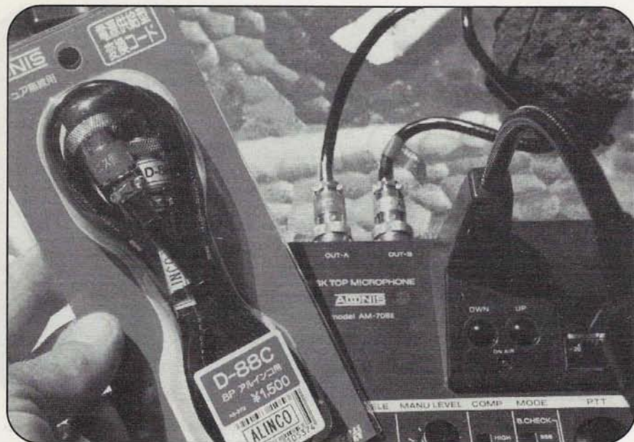
Photo B. Each Adonis mic requires a $9.95 connector cable, prewired for your specific radio. This provides the flexibility to use the mic with several different radios simply by swapping the cables.
