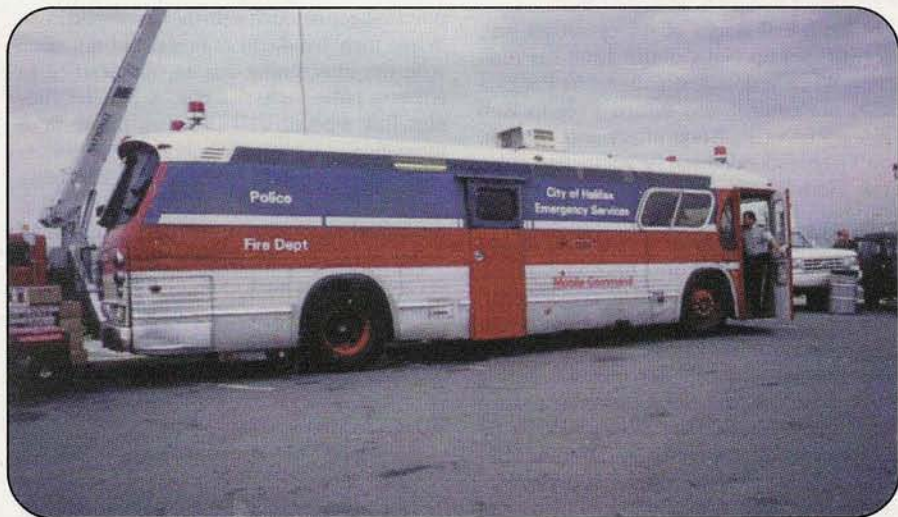
Photo C. The Command Bus operated by the Halifax Regional Municipality. The front part serves as a command area and the back as a communications center. Photo by Joe MacPherson, VE1CH.
