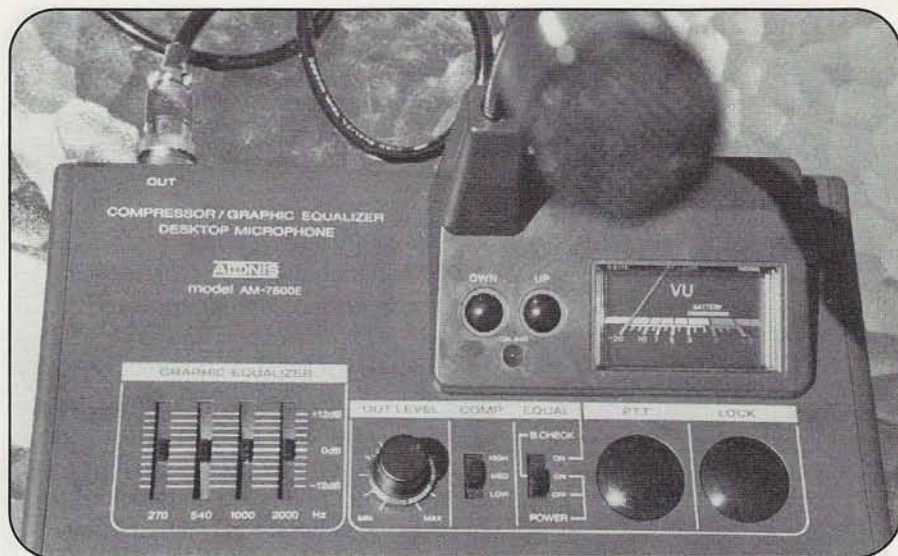
Photo C. The Adonis AM-7500 is the company's top-of-the-line desk mic, featuring audio compression, a graphic equalizer, and a multi-function VU meter built into the base.
