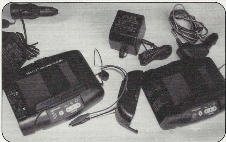
Here are two examples, from Maha (left) and Periphex (right), of "smart" chargers which allow you to safely fast-charge NiMH battery packs. But their higher cost must be included in your overall cost calculation of whether it's more economical for you to stick with NiCds or switch to NiMHs.
