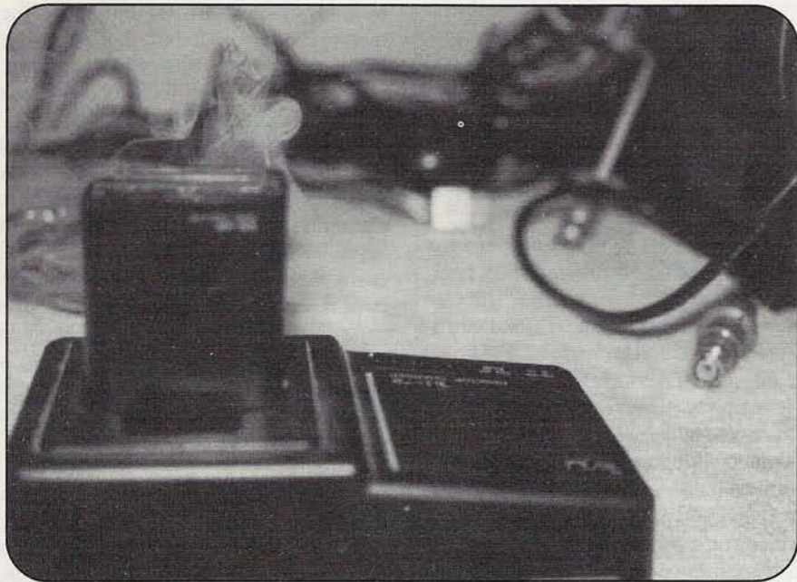
Can you see the smoke rising from the battery pack? Overheating, possibly leading to meltdowns and fires, can be a major problem if an NiMH battery pack is fast-charged in a "standard" NiCd desk charger. Microprocessor-controlled "smart" chargers are safer but considerably more expensive.
