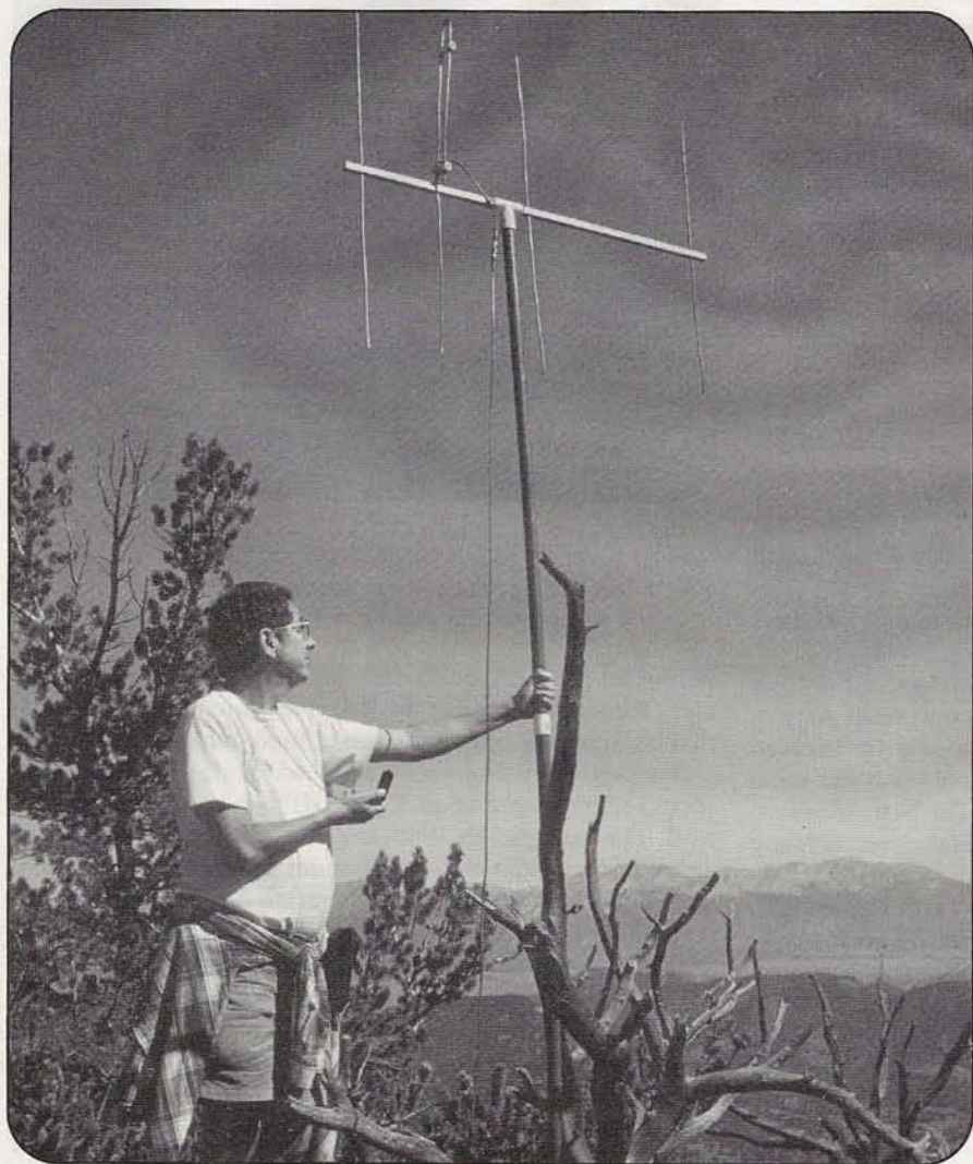
Photo C. Sam Vigil, WA6NGH, uses a compass to aim his four-element "Cheap Yagi" antenna, built from WA5VJB's plans here in CQ VHF. (KF6NEV photo)
