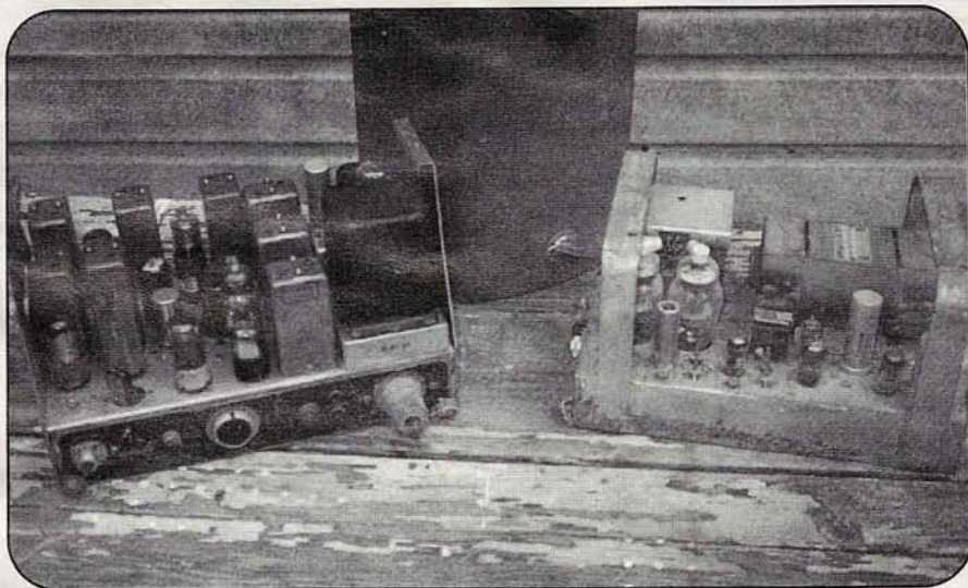
Radios were typically purchased surplus and converted into early ham repeaters. On the left is a pre-WW II 30- to 40-MHz receiver with an AC power supply. On the right is a GE transmitter for the same frequency range, circa 1946. Transceivers, combined transmitters and receivers in a single case, didn't appear until the mid-1950s.
