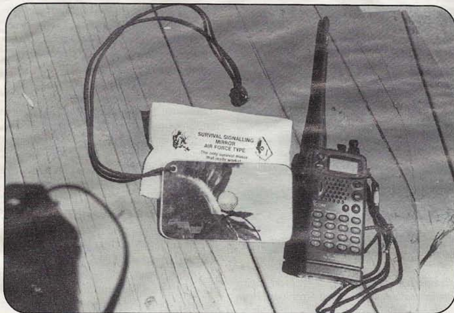
Photo B. Basic ham radio mirror signaling gear: a 3 x 5-inch "Survival Signalling Mirror, Air Force Type" (note the hole in the center for aiming) and a handheld radio. These signaling mirrors are available from hiking and outdoor stores for about $8 each.
