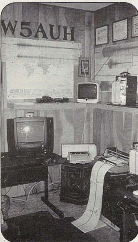
Photo C. W5AUH's homebrew earthquake monitoring station. Both he and W5VID have transmitted charts of ground vibration via ATV while an earthquake is in progress somewhere in the world.
