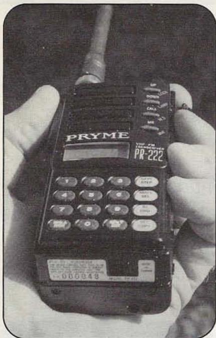
Photo B. The PR-222 (and the PR-52) feature flat bottoms so you can stand them on a table without fear that they'll fall over. The battery pack takes up the entire back of the radio.
