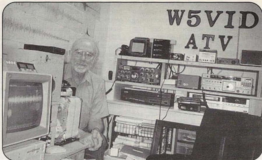
Photo B. W5VID's combination amateur radio/amateur seismology station. Note the seismograph readings on the computer monitor.
