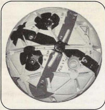
Photo D. NASA's shuttle-based "Sprint" AERcam—a sphere containing two TV cameras that floats in space outside the space shuttle (with control from inside) during spacewalks. It sends back video with a low-power radio signal. Will you be the first to successfully monitor these transmissions on Earth? (Courtesy NASA)
