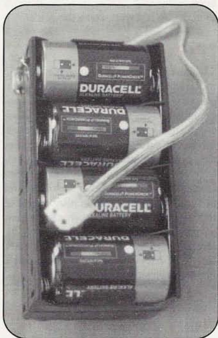
Photo A. The Mercury ARA battery pack. This eight-D-cell, 12-volt battery pack is the basis of a standardized power system used by members of the Mercury Amateur Radio Association in California. The pack and its various accessories use the ARES national power connectors. (Photos courtesy of the author)
