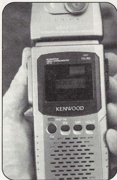
Photo E. The Kenwood VC-H1 Visual Communicator makes up the second part of this all-in-one portable station, plugging into the TH-D7A to send and receive slow-scan TV pictures. It takes about 15 seconds to send one still frame at 9600 baud. (WB6NOA photo)
