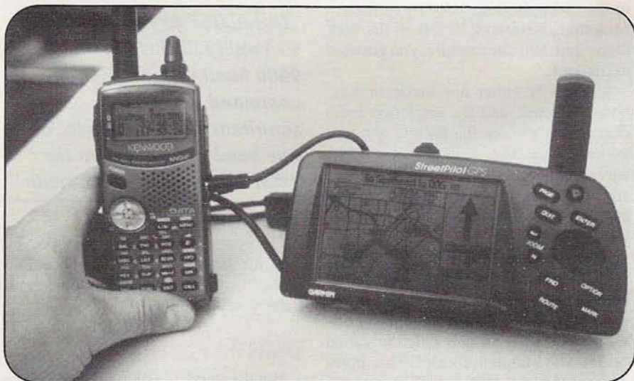
Photo D. If you plug in the optional cable to connect the TH-D7A to a GPS (Global Positioning System) receiver, such as this Garmin Street Pilot, the HT will display your location by latitude, longitude, and six-character grid square. And it can transmit that information via APRS. (N3JF photo)
