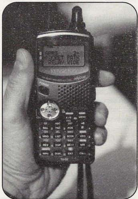
Photo C. There's a 1200/9600-baud packet TNC built into the TH-D7A, along with software for sending and receiving APRS (Automatic Position Reporting System) data and messages. (N3JF photo)
