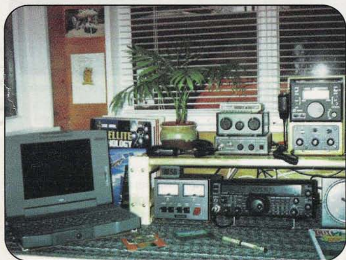
VE7FM and VE7SBM's "Earth station." Main rig is a Yaesu FT-847. The station is active on HF, 2 meters, 70 centimeters, and 2.4 GHz, operating mostly QRP on SSB, SSTV, CW, RTTY, and packet.
