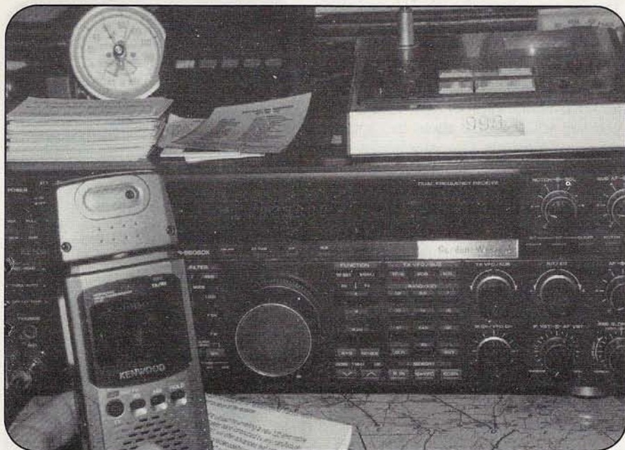
Photo H. The VC-H1 is not limited to use with the TH-D7A or even to VHF/UHF. Its built-in SSTV software automatically selects the transmission mode in use, allowing it to be used as a video source and monitor for SSTV on HF as well. Look in on 14.230 MHz sometime. (WB6NOA photo)
