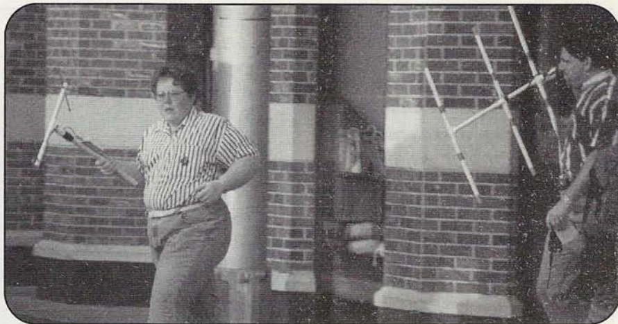
Photo C. Compact, rugged beams and quads are preferred by most foxhunters for on-foot use.
