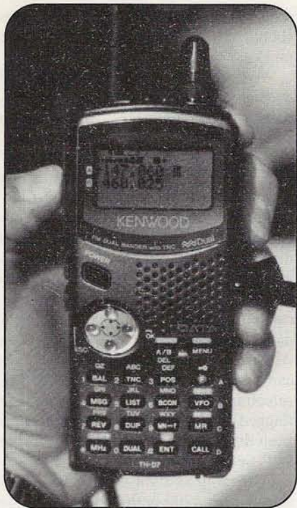
Photo B. At its most basic, the Kenwood TH-D7A is a full-featured dual-band handheld. But as the funny button on the left and the cable on the right suggest, this radio is more than just another dual-bander. (N3JF photo)
