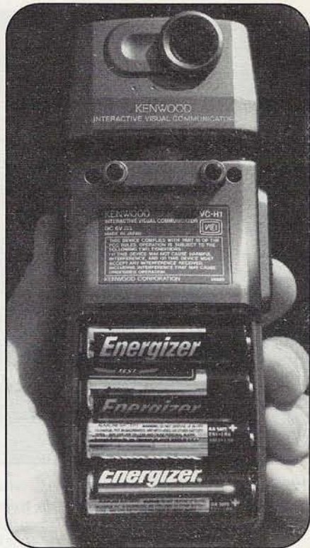
Photo G. The VC-H1 has its own power source—four AA batteries—so it's not a drain on your HT batteries. A single set of AA batteries kept the VC-H1 running all through the 1999 Pasadena Rose Parade. (WB6NOA photo)
