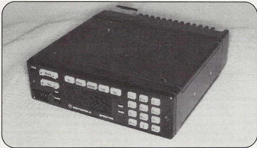
Photo B. This is the more common automotive "dash-mount" version of the Spectra. Not shown are the required external speaker and the microphone.
