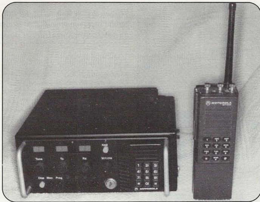
Photo D. The MCX100 railroad radio (left) requires expensive EPROMs and a special programmer to change the operating frequencies. The MT500 (right) can be purchased very inexpensively, but it uses individual transmit and receive channel elements, which can be very costly to purchase. Like most other commercial HTs, it's available with or without a keypad.
