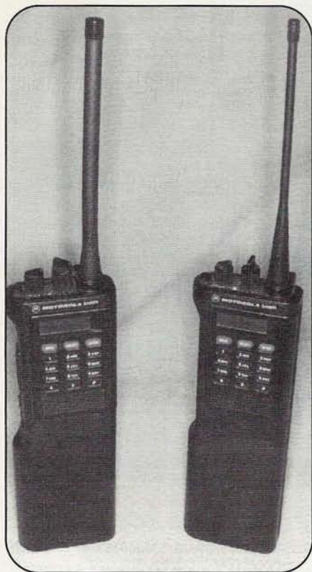
Photo E. These Motorola Saber Handie Talkies correspond to the Spectra mobiles in design and age. The VHF Saber will program to any frequency between 146 and 174 MHz, with any repeater offset you wish, and offers a full range of subaudible tone and digital squelch control capability.
