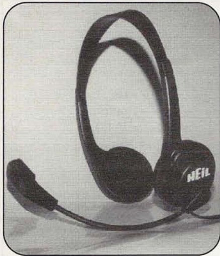
Photo B. New Heil mini headset with boom mic is lightweight for comfortable long-term operations, and it sounds terrific on both transmit and receive. Mic case will accept various Heil elements for customizing to your voice. All Heil elements are dynamic type and designed to match the input impedance of modern solid-state transceivers. Photo courtesy Heil Sound Ltd.
