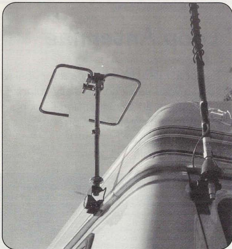
Photo B. The HO loop mounted on WB6NOA's communications van. While designed primarily for mobile use, the antenna is equally at home in base station installations where space is limited or you want an omnidirectional antenna.
