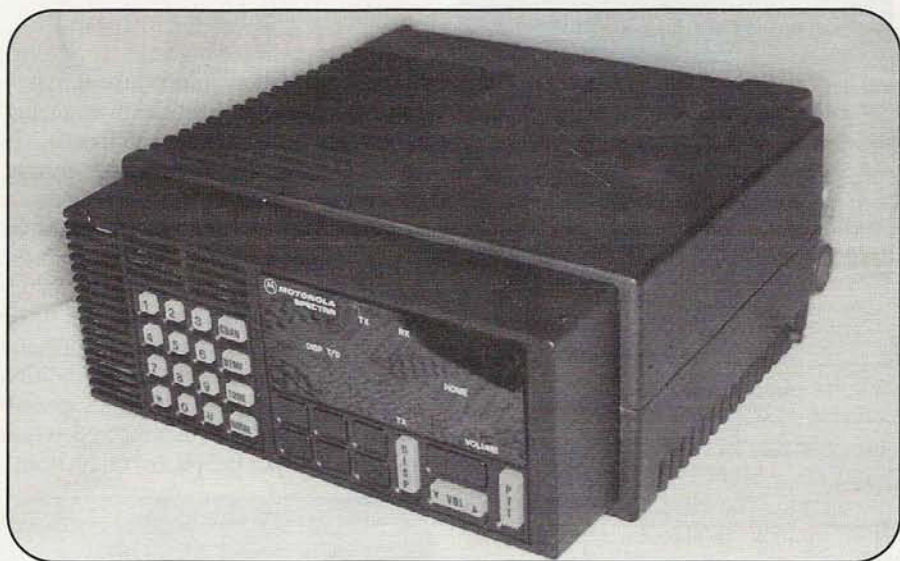
Photo A. Motorola's "Railroad Spectra" is an adaptation of the company's popular high-end automotive radio. Special features include a dual-voltage power supply option and extensive DC filtering and conditioning. Remember...these were used in cabooses, where they were battery powered, and in locomotives, where they had to coexist with hundreds of volts and thousands of amperes of traction power.
