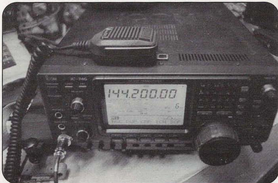
Photo A. ICOM's IC-746 covers all nine HF ham bands plus 6 and 2 meters, with 100 watts out on all bands. In addition, the radio includes a general coverage receiver tuning 300 kHz to 60 MHz and 108 to 174 MHz.
