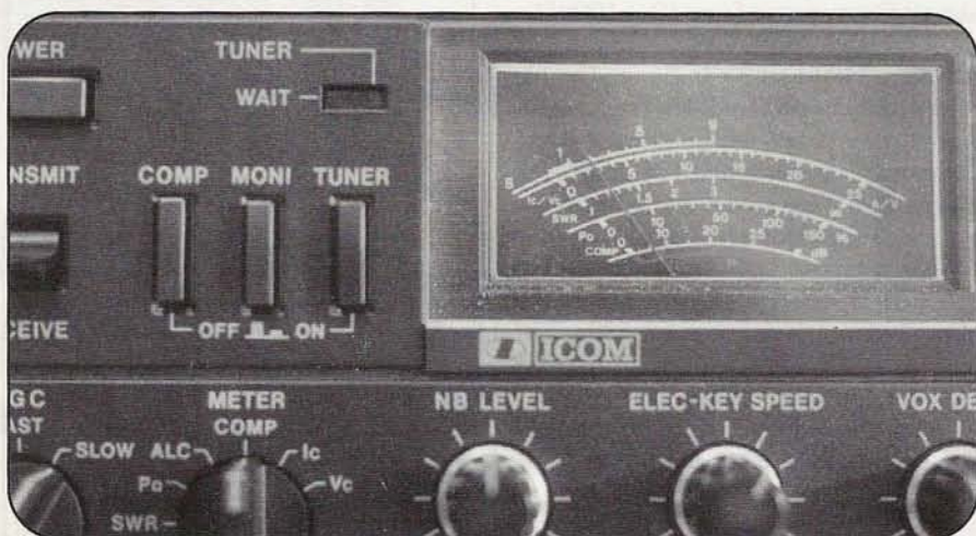
Photo E. The speech compressor in most SSB transceivers is also beneficial for enhancing your transmitted audio, if properly adjusted and used. You want just enough compressor action to accentuate high tones but not compress the audio and cause "pumping." Typically, this equates to minimum rather than maximum ALC-metered action.
