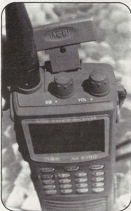
Photo E. If you enjoy broadcast-band DXing, the supplied ferrite rod antenna can be added on to dramatically improve reception on the AM broadcast band.
