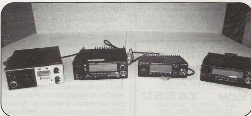
Photo F. Mobile rigs through the years for 222 MHz include (from left): 1970s Tempo 220, Kenwood TM-631A dual-bander and TM-331A single-bander, and the ICOM IC-2330A dual-bander. Of these, the TM-331A is the only one still offered new, along with ADI/Premier's new Pryme AR-247 (not pictured), and transceiver kits available from Ten-Tec and Ramsey.
