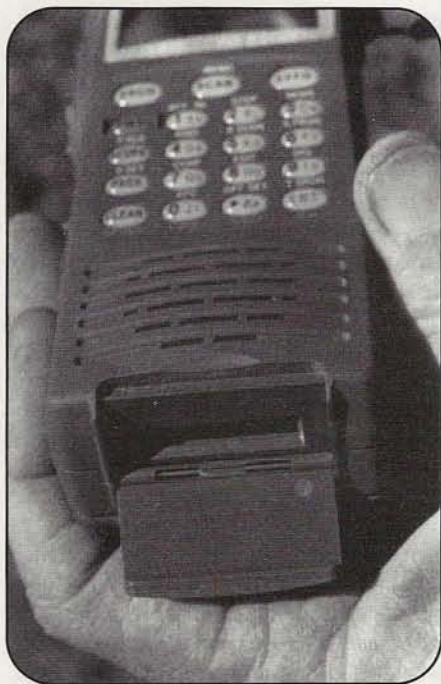
Photo B. The AR8200 has a trap door to accept one of five "slot cards" that provide additional options (kind of like a PCMCIA card on a laptop computer). See text for details.
