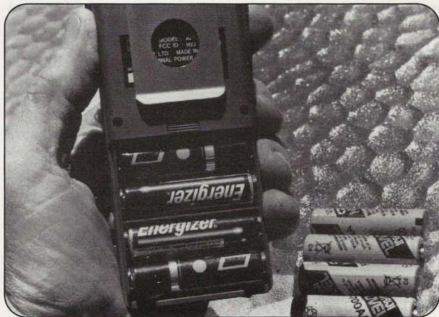
Photo C. This handheld scanner/shortwave receiver comes with rechargeable nickel-cadmium (NiCd) batteries, but will also work with standard alkaline cells. Alkaline batteries will last twice as long as the NiCds, but can't be recharged.
