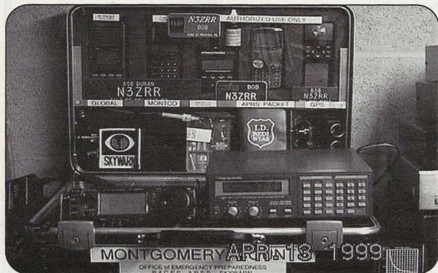
Photo E. N3ZRR's "EOC on the run" contains a full HF/VHF/UHF station, regular and trunk-tracking scanners, and a frequency counter that automatically tunes one of the scanners to any active frequency. See "Tools of the Trade" for specifics on what's "in the bag." (N3ZRR photo)
