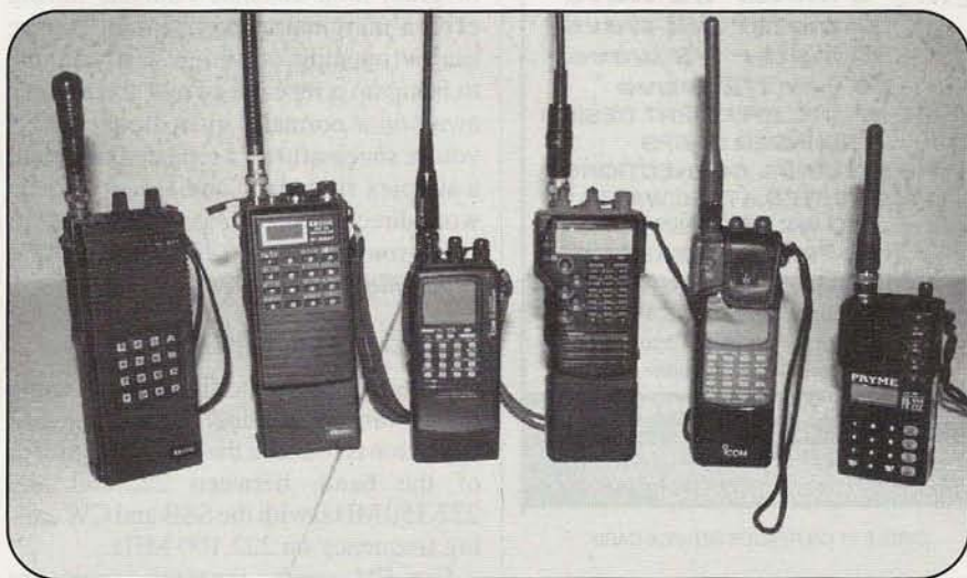
Photo E. Some of the 222-MHz handhelds offered over the years, including (left to right) ICOM's IC-3AT, IC-03AT, and IC-V21AT (dual-bander); Standard's dual-band C-228A; an ICOM IC-3SAT; and, the only one of these currently in production, the new Pryme PR-222. Alinco and Yaesu also offer 222-MHz handhelds.
