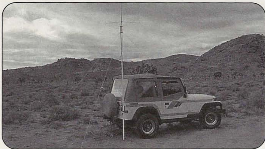
Photo B. Dave Stone, KC6UUR, set up his dual-band vertical "Tram 1480" antenna to assist with communications. Dave says, "At eight feet long, I can just fit it under the back seat and passenger seat for transport." (KC6UUR photo)
