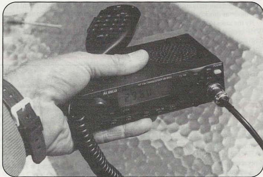
Photo A. The Alinco DR-M03 10-meter FM mobile transceiver is small enough to hold in one hand, but puts out a 10-watt signal that's more than capable of being heard when the band is open. There's a matching 6-meter version as well, the DR-M06. (WB6NOA photos)
