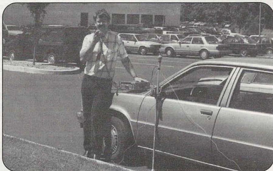
Photo A. The author with his portable 10-meter station that he sometimes uses during lunch hour at work. His rig is wired directly to the car battery and the antenna is a stainless steel vertical with wires as radials. (Photos by the author)
