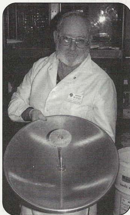
Here, W5DID is holding P3D's high-gain S-band dish antenna. This will be used for 13-centimeter communication when the satellite is in the portion of its orbit that is farther from the Earth.
