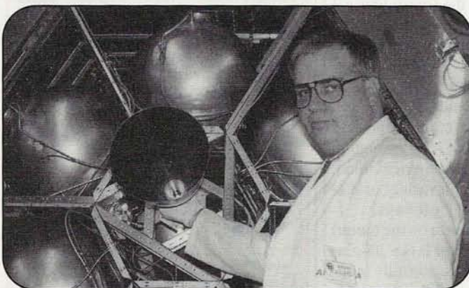
KA1RHL holds the P3D motor in place to show where it will be mounted on the satellite. The round tanks surrounding the motor will hold fuel for maneuvering the spacecraft in orbit.
