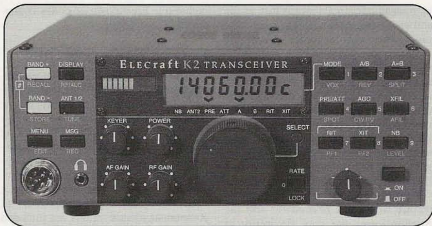
Photo D. Close-up view of the K2's front panel. See text for descriptions of the various functions, and Elecraft's "tap-hold" method of getting double use out of most keys.
