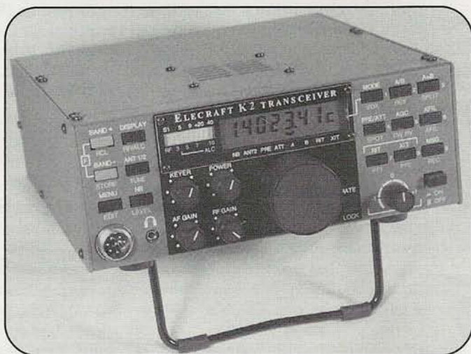
Photo A. The Elecraft K2 Transceiver runs on 12 volts DC and puts out 10 watts on all HF bands, making it a perfect choice for driving a transverter during portable operations. (GM4PLM photos)
