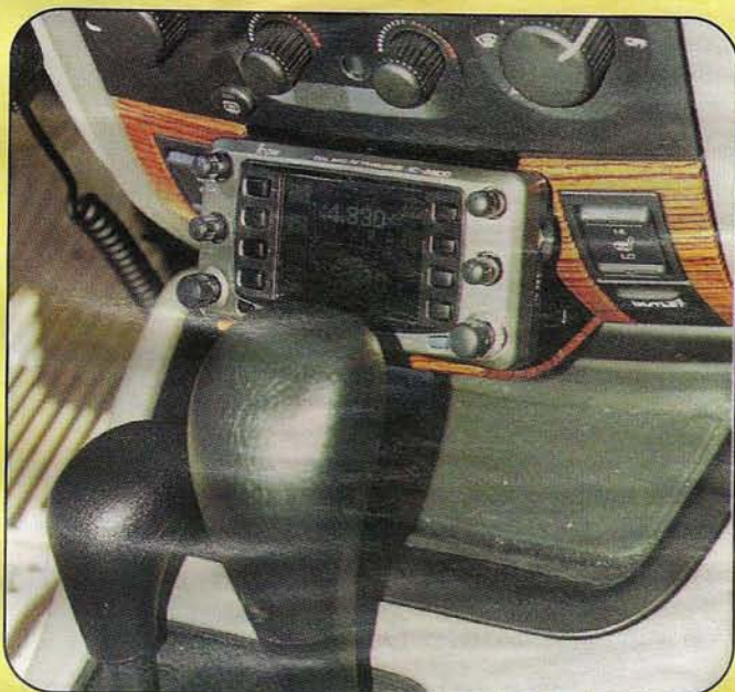
Photo G. The IC-2800's control head mounted easily to WB6NOA's dashboard with hook-and-loop fasteners, and there was no problem hearing the audio output from the speaker, which is located in the back of the control head.
