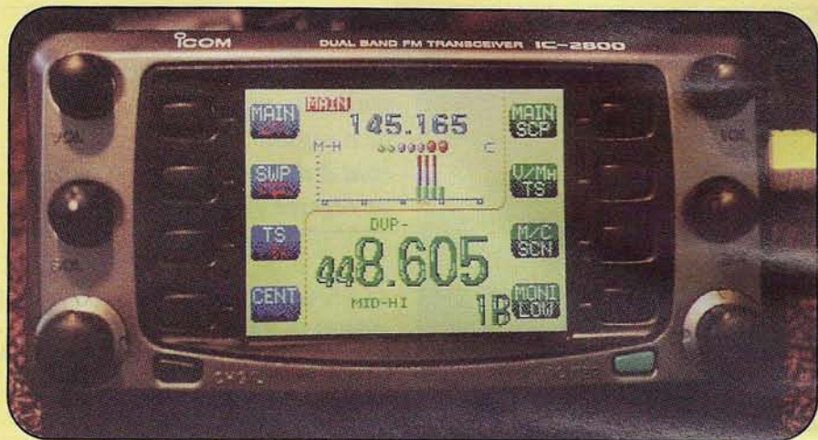
Photo B. The "funky" display, complete with a grapes, plums, and cherries S-meter, is one of four display options you may select for the IC-2800.
