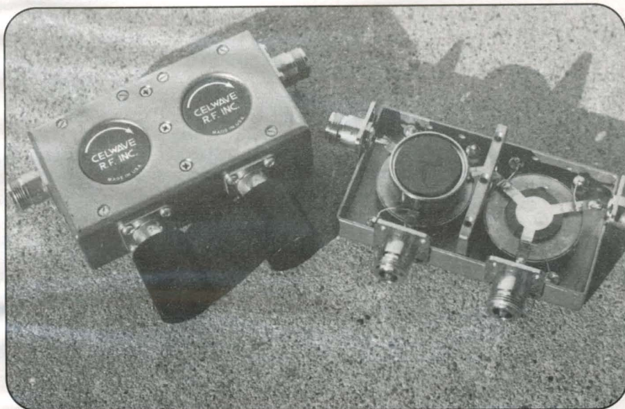
Photo A. Typical cell site circulators. These special filters are used to prevent interference when multiple transmitters and receivers operate in close proximity to each other. See "Microwave Mini-Glossary" for a more detailed explanation.
