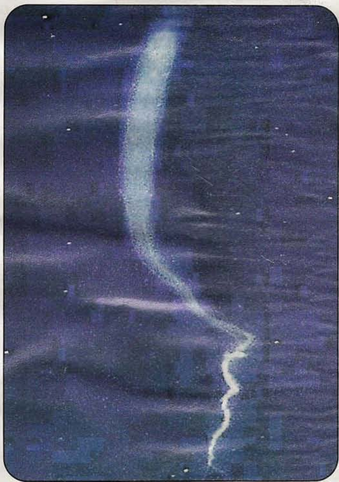
Photo. A trimethylaluminum (TMA) cloud over the Poker Flat Research Range in Alaska, following release from a NASA sounding rocket in 1978. Similar TMA releases were planned for July over the U.S. east coast. (NASA photo)
