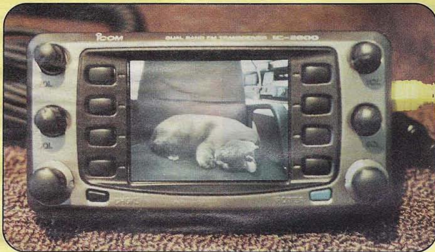
Photo D. The IC-2800 accepts a standard video input (via the yellow plug on right) to let you hook up a camera to keep watch on who's sleeping on the job or to monitor ATV images—but the unit itself does not transmit or receive video.
