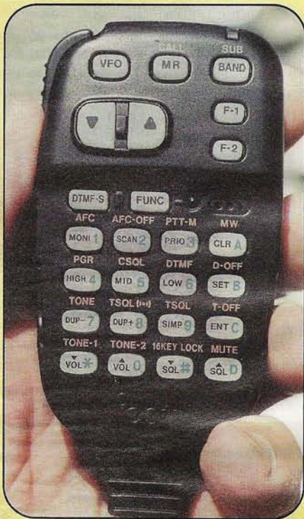
Photo E. This do-everything microphone is standard equipment with the IC-2800. See text for details of what you can control from the microphone (hint: nearly everything!).
