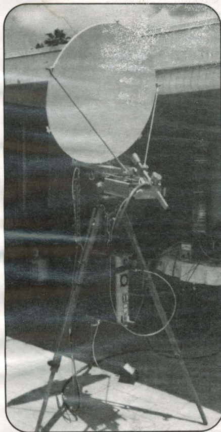
Photo B. Have tripod, will travel. Peter Bauer, W6DXJ, of El Cajon, California, is ready anytime, anyplace, to put a 10-GHz signal on the air with his tripod-mounted 30-inch offset feed dish and 15-watt TWT amplifier. (W6DXJ photo)
