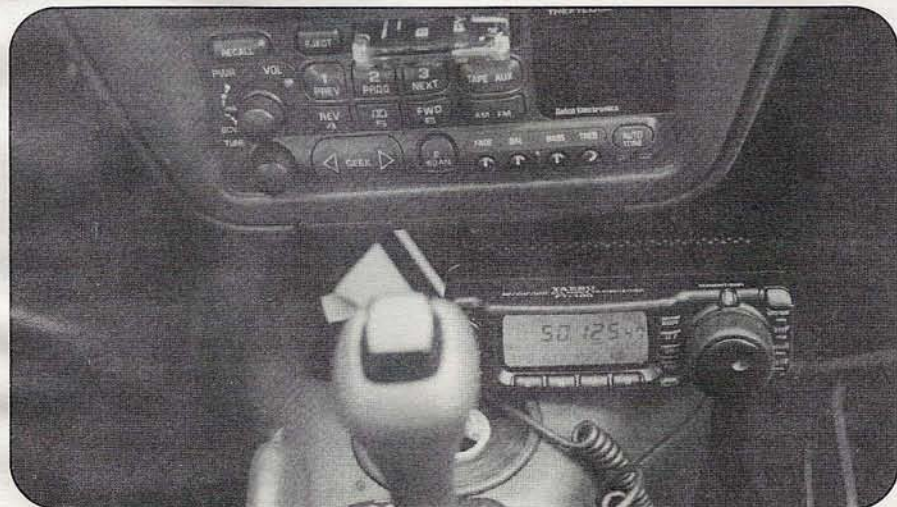
Photo D. Once he found the 3-inch grommet through his car's firewall to run the power cable to the battery, WB2AMU was able to conveniently mount the FT-100 to his car's center console. (WB2AMU photo)
