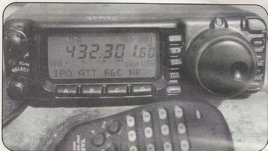
Photo A. The Yaesu FT-100 Field Commander operates on all ham bands between 160 meters and 70 centimeters (except 222 MHz), with 100 watts out on HF and 6 meters, 50 watts on 2 meters, and 20 watts on 70 centimeters. Features include all-mode operation and 349 memory channels. (WB6NOA photo)
