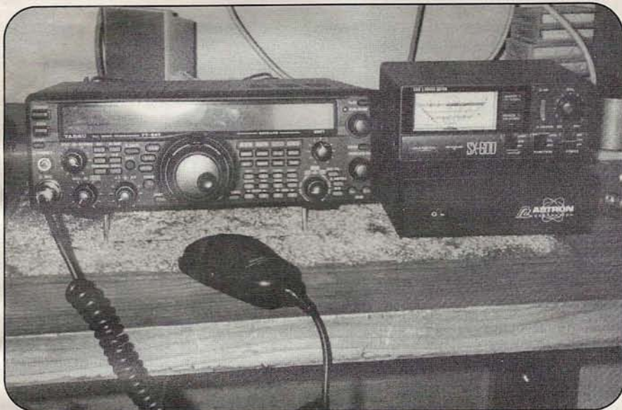
Photo B. The transmitting station consisted of a Yaesu FT-847 transceiver and a power meter to monitor the output power, which was varied to simulate varying distances and band conditions. (Photos B through D by Sara Witte)
