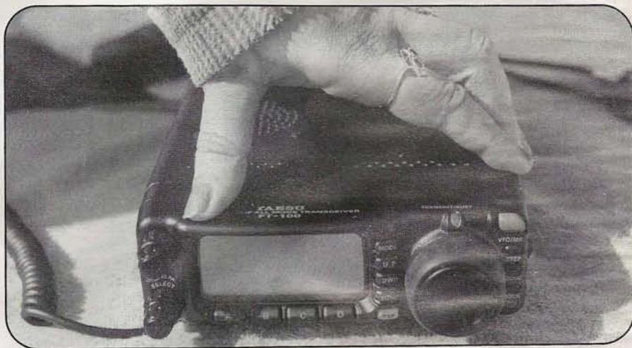
Photo B. Mobile or portable operation is a snap with the FT-100, and, at only 6 1/2 inches wide and weighing only 5 pounds—including the microphone—it's easily carried in one hand or an attaché case. (WB2AMU photo)
