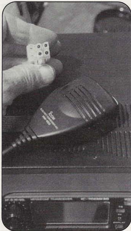
Photo B. While most rigs using the six-conductor Molex power plug have the locking tab on the top, the tight construction of the IC-706 Mk II-G made it necessary for ICOM to install it "upside down." The new model solves some of the internal problems that resulted when hams tried to connect the cord the wrong way.
