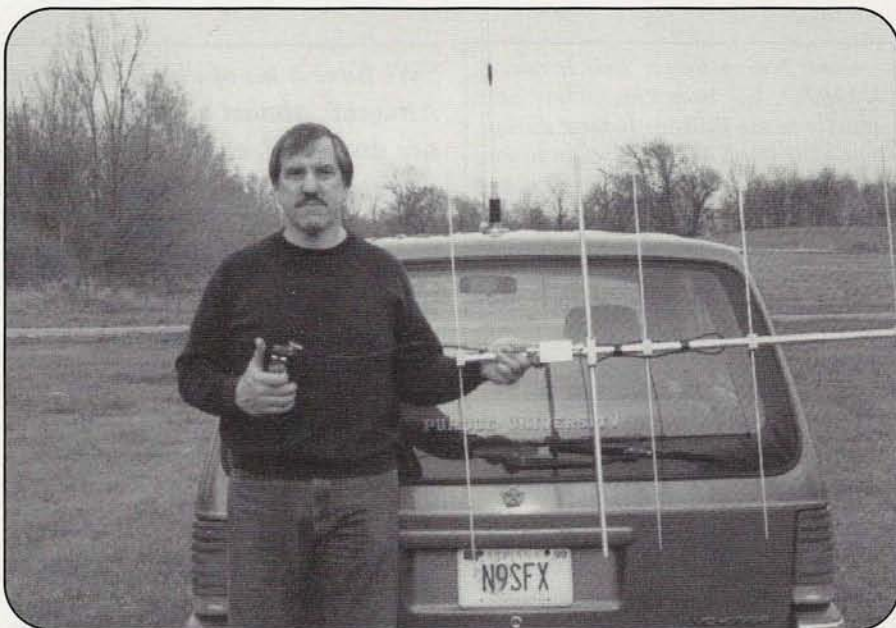
Photo A. The author, set to begin tracking down a mystery transmitter, with his HT, RF attenuator, and five-element Yagi. (Photos courtesy of the author)
