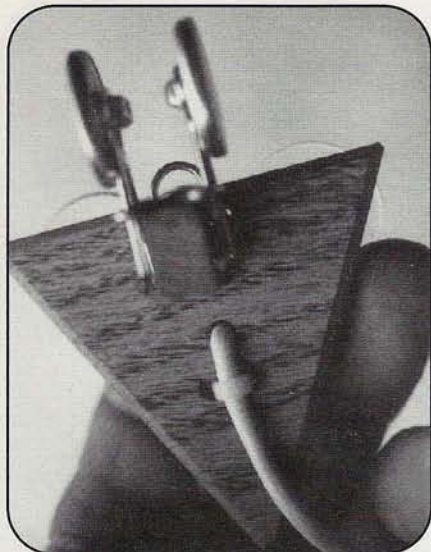
Photo B. Named for the popular brand of office binder clips from which it's made (along with a set of brass buttons and a wooden base), the Bull Dog iambic paddle set plugs into virtually any electronic keyer and takes up practically no space on your operating desk.
