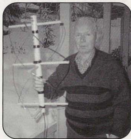
Photo A. The author holding his finished quadrifilar helix antenna, as modified from the original presented in QST in 1996 (see notes). (Photos courtesy of the author)
