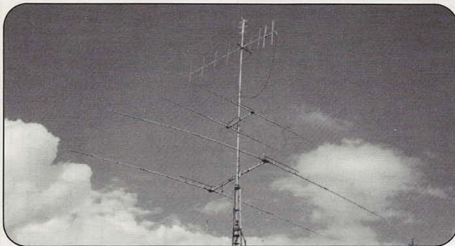
Photo C. The quadrifilar helix mounted on top of SM51BE's tower. The author found that top-mounting was necessary to keep the tower itself from blocking signals when satellites were "behind" the tower.
