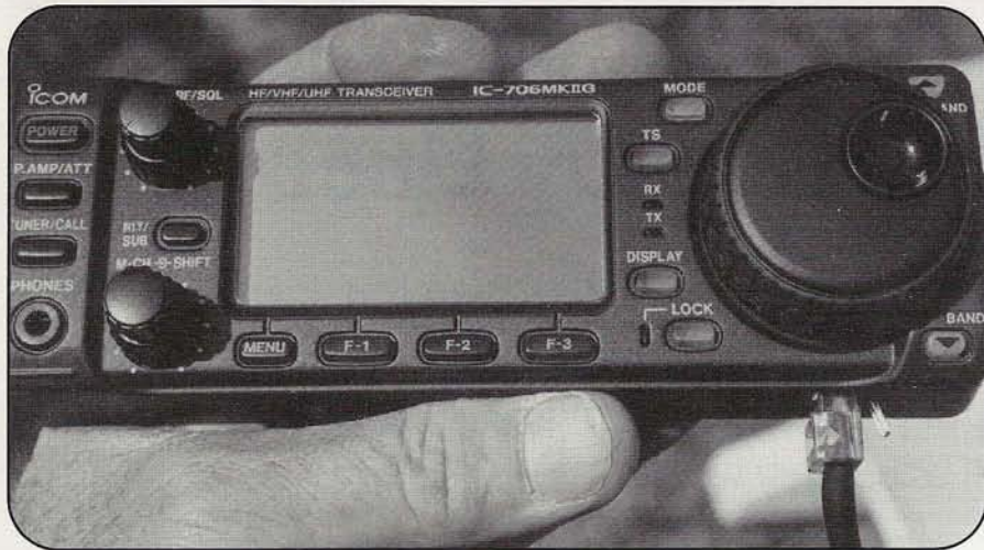
Photo E. The IC-706 Mk II-G has a removable control head which can be detached from the radio and mounted elsewhere, as long as you buy an optional connecting cable. Mic and speaker may be plugged into either the head or the main body of the rig, and there's a switch on the back of the control head to toggle the output to the "phones" jack between headphone and speaker levels.
