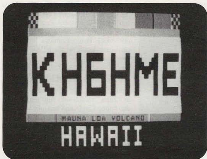
Photo D. KH6HME's ATV (amateur television) ID screen, as monitored by WB6NOA on 434 MHz, 2,500 miles away in southern California. (WB6NOA Photo)
