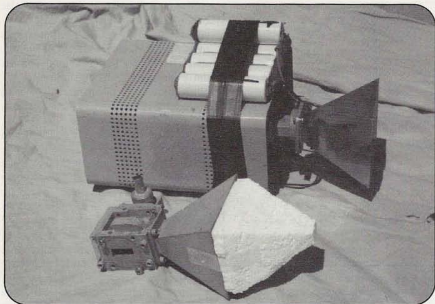
Photo B. Two variations on the common "Gunnplexer" system. At the top is a Gunnplexer with a horn antenna, while the bottom Gunnplexer horn has a radio "lens" to reduce phase error. See text for explanation.
