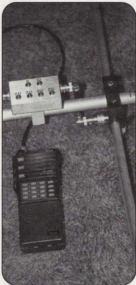
Photo B. Close-up view of N9SFX's 95-dB attenuator, clamped onto the mast of his antenna and connected to both the antenna and radio.
