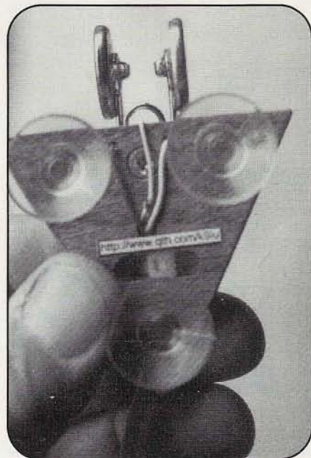
Photo C. The tiny Bull Dog paddle keeps a firm grip on your desk with three small, but effective, suction cups attached to the bottom of the triangular wood base. You really need to see one "in person" to appreciate how cute it is!
