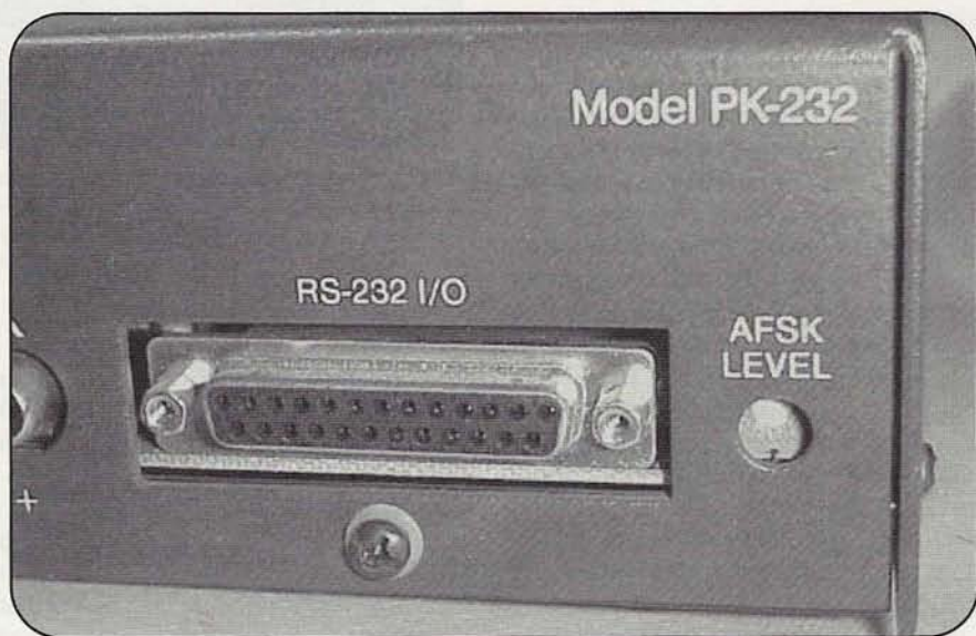
Photo C: The RS-232 connector and transmit level adjustment potentiometer (labeled AFSK Level) on the back of an AEA PK-232. Compare these with those shown in Photo B.
