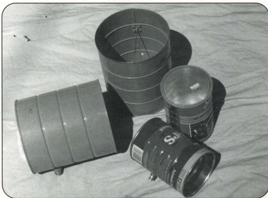
Photo. 1200-MHz and 2300-MHz horn antennas made from coffee cans. Your next feedhorn may be as close as your kitchen pantry.
