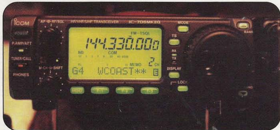
Photo F. At night, the ICOM display's sharp contrast makes the characters easy to see. The buttons are backlit as well, and the backlighting levels are adjustable.
