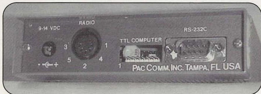
Photo B: The back panel of a PacComm Tiny-2. Note the well-marked RS-232 and radio ports. This model also has a TTL (transistor-transistor logic) port, required for some computers. Just inside the TTL port opening, on the left, the white transmit audio level adjustment potentiometer can be seen.
