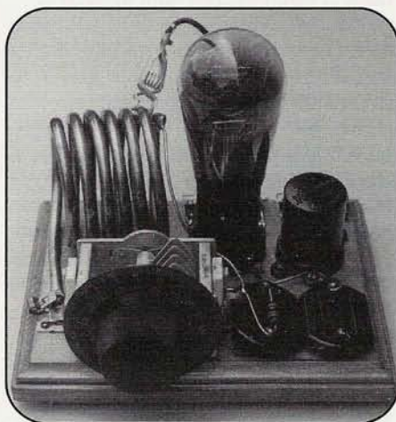
Photo A. This modern-day replica of a 1930s-style transmitter uses a type 45 tube in a basic Hartley oscillator circuit and pumps out a healthy 5-watt signal on any frequency its tuned circuit covers. When powered from a well-filtered and regulated power supply, it emits a beautiful sounding signal on today's bands.
