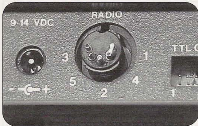
Photo D: A crude but effective audio loopback jumper, made from part of a 5-pin DIN connector. This connector is a TNC-2 standard, but other types of connectors are also used for the radio connections.
