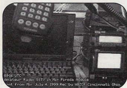
Photo C: Ham station ROMIR -- the amateur radio packet and SSTV setup aboard the Mir space station, as it was set up before the final long-term crew returned to earth in late August. See text for equipment description.
