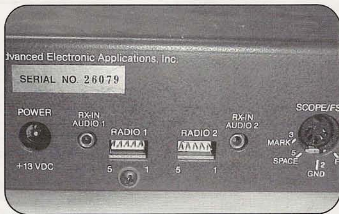
Photo E: The radio connector as found on the back of an AEA PK232 multi-mode data controller. Although it's very different in appearance from the one shown in Photo B, it serves the same purpose.
