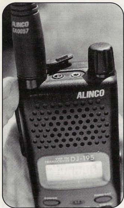
Photo D. There's only one dial on top of the radio, and it controls frequency, volume, and squelch, depending on which keypad buttons you press first. See text for details.
