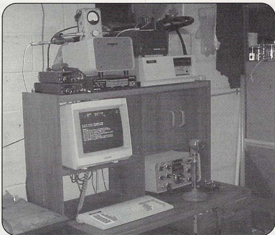
Photo A: The N2IRZ packet console, which runs on an old 4.77-MHz 8088 PC, an ancient AEA PK-232, and an even more ancient ICOM IC-25H radio. Not pretty, perhaps, but it works. Sometimes, I use the PK-232 on HF with my much more ancient Heathkit SB-102, for RTTY, Morse, and even 300-baud packet.
