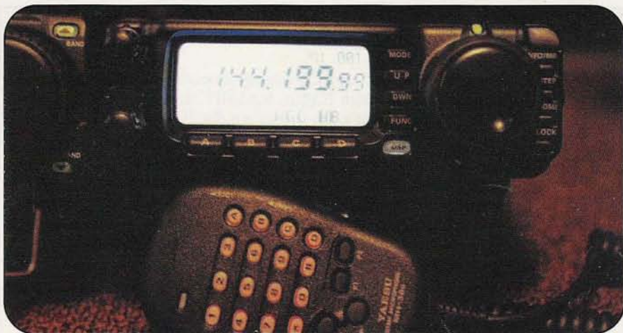
Photo G. The FT-100's display isn't quite as clear at night as the 706's, but it was preferred for nighttime viewing. The buttons on the radio are not backlit, but the microphone buttons are. As on the 706, backlighting levels are adjustable.
