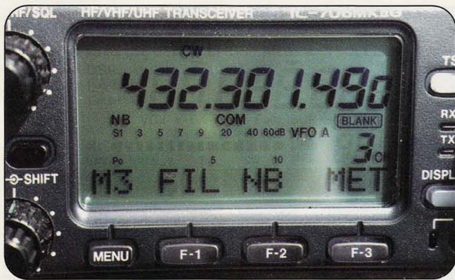
Photo D. The LCD display on the IC-706 Mk II-G is black on a light green background. Users found it easier to see at wide angles and preferred it during the day, but sitting out in the heat makes it all go black.
