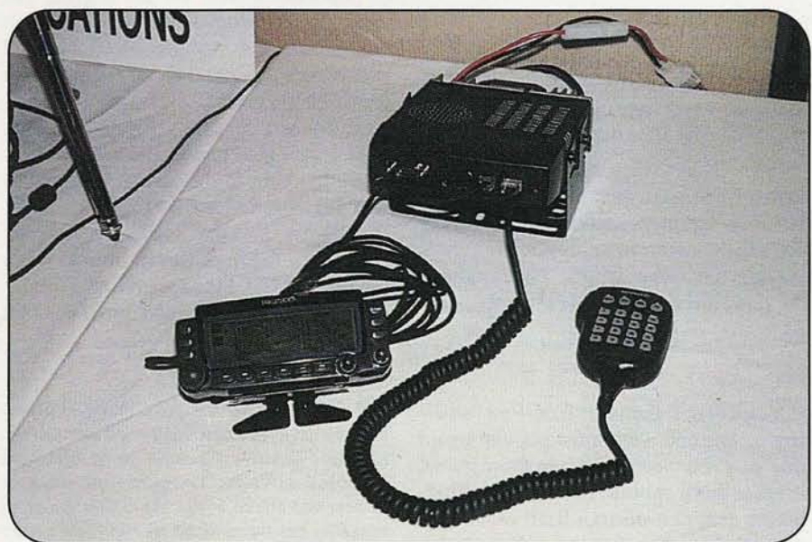
Photo D. The control head of this radio cannot be attached to the body, and a remoting kit is standard, as is an adhesive-backed clip that can mount the head to your car's dashboard or wherever else you'd like to put it. Note that the mic plugs into the radio body, not the control head.
