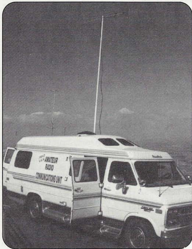
Photo D. WB6NOA uses the Maspro fold-up Yagis on top of the telescoping flagpole mast on his van. He says they're ideal for quick setup and tear-down.
