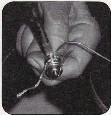
Photo F. Once the antenna is assembled, the final step in construction is to solder on a connector to the end of the coax cable that's not already attached to the antenna. In this photo, a PL-259 is being used. You may use any other coax connector that suits your needs.
