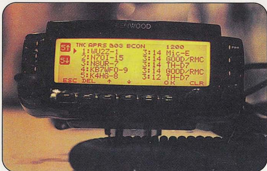
Photo C. The multifunction LCD screen also serves as a terminal unit for displaying received packet data. In addition, it will display a list (seen here) of the last 40 stations heard.
