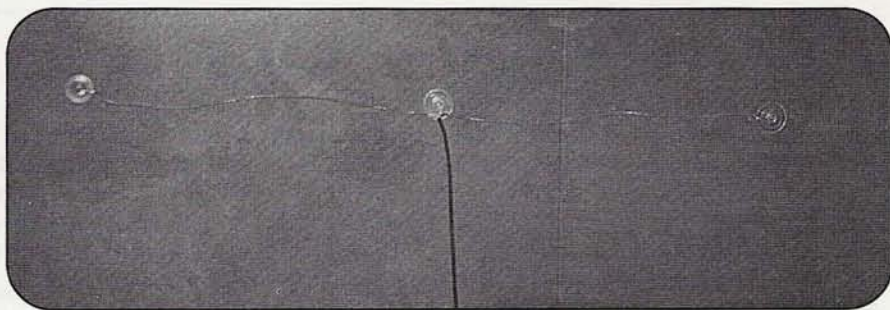
Photo E. The completed dipole is only 38 inches long and can be stuck up most anywhere. A window will work much better than this radiator, of course, but it's easier to see the antenna against the dark background of the radiator than against outside light.
