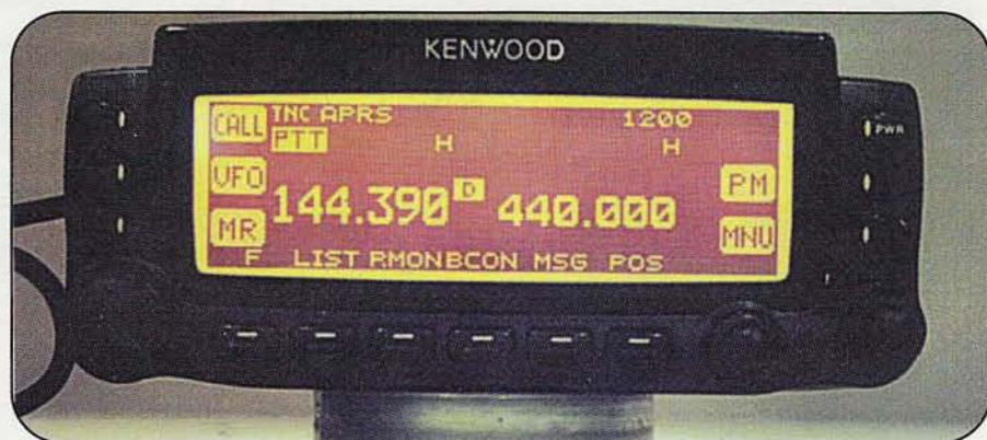
Photo B. It has no name yet, but Kenwood's new FM/packet mobile rig comes with a built-in 1200/9600-baud TNC, and puts out 50 watts on 2 meters and 35 watts on 70 centimeters.
