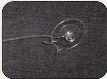
Photo D. The outer end of each dipole wire may simply be looped around a hook on the suction cup. If more flexible wire is used, you might want to cut it a little long and wrap some of the wire back on itself after looping through the suction cup hook.
