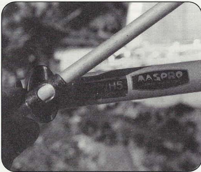
Photo E. To assemble the Maspro Yagi, just line up the colored dot on each element with the hole in the holder, rotate into position, and hand tighten the wing-nut underneath.
