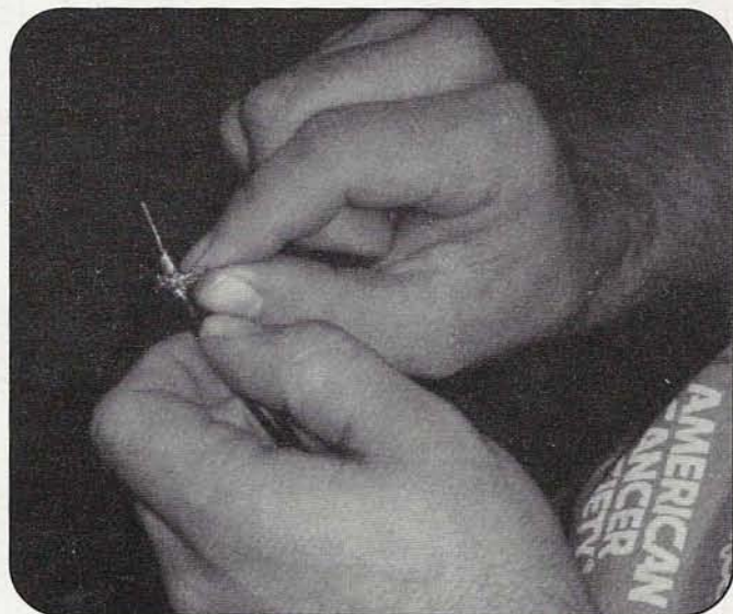
Photo B. One of the first steps in preparing the coax is to pull the braid back.
