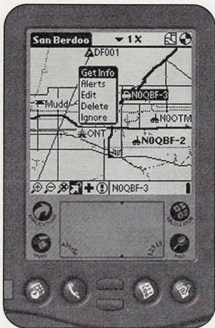
Photo C. The "pocketAPRS" screen as seen on a 3Com PalmPilot organizer. (Photo courtesy Mike Musick, N0QBF)
