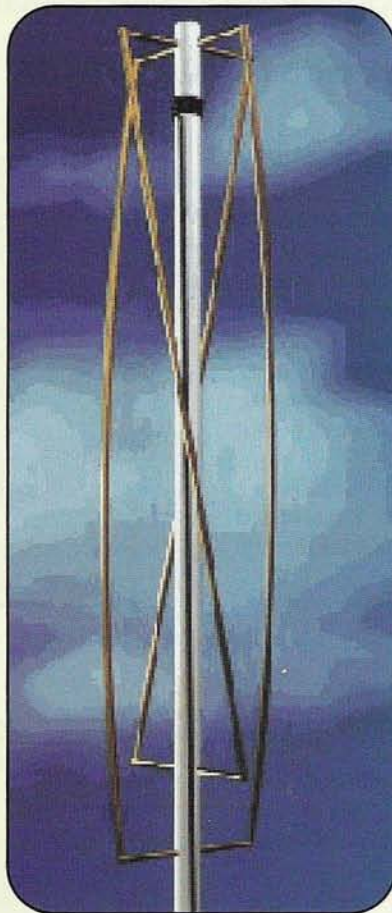
Photo 10. The Lindenblad antenna for 2 meters. Originally design for aircraft communications, this rather strange-looking design offers an omnidirectional pattern and circular polarization, which is ideal for horizon/low-elevation passes. Like the helix, it is either RHCP or LHCP; switching is not an option. (Photo courtesy Howard Sodja, W6SHP)
