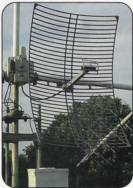
Photo 8. The "bar-b-que grill" antenna for S-mode downlink derives its name from the cast-magnesium/aluminum reflector. This model has better than 24-dB gain. Its original function was for Multipoint Microwave Distribution System (MMDS)—i.e., wireless cable television. (Photo by the author)
