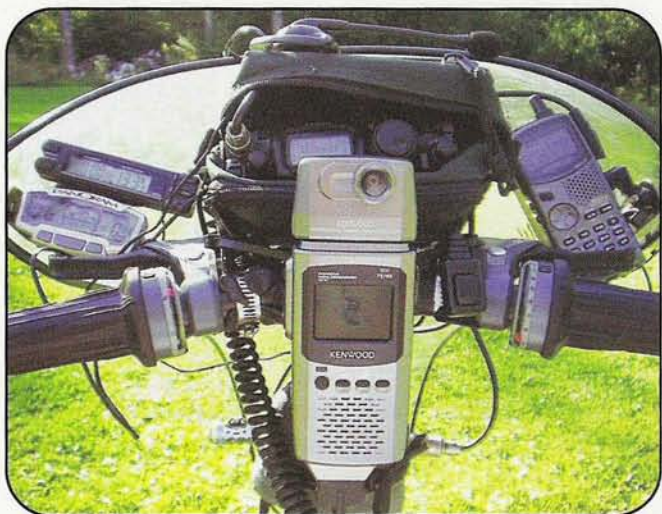
The mobile shack. Battery/solar-panel voltage as well as cycle computer on the left, FT-817 in the middle with the Kenwood VCH1 SSTV converter under it, and the THD7 APRS-enabled HT on the left.
