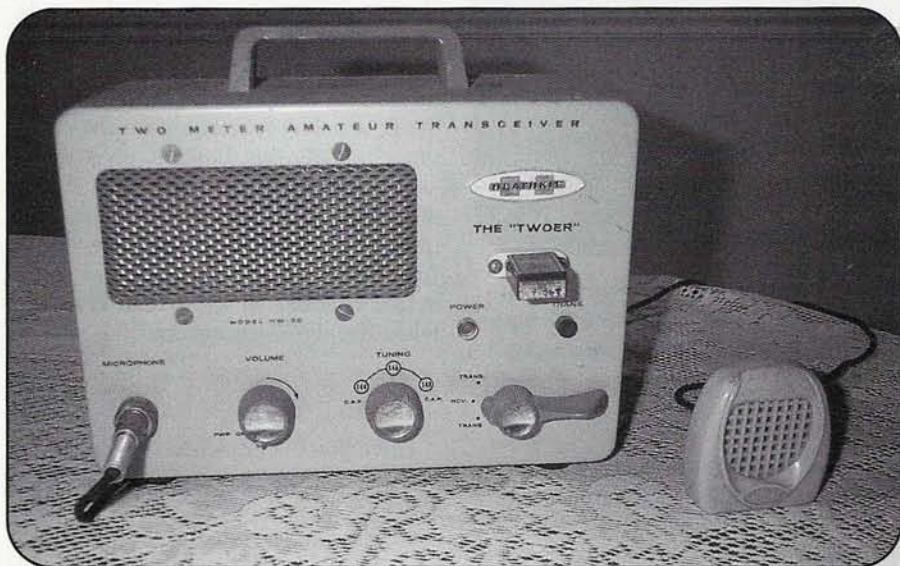
The Heathkit Twoer, a 2-meter AM transceiver with a crystal-controlled transmitter and a tunable receiver.
