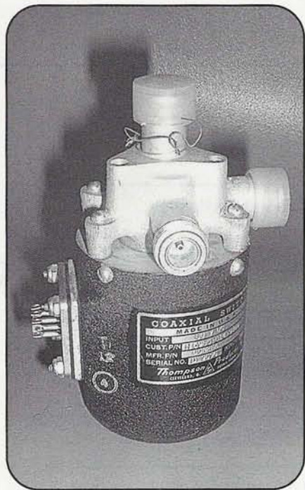
Photo 3. This Transco relay is similar to the mast-mounted relay on the author's tower. It selects which antenna is connected to the feedline. The relays use a solenoid-driven indexing DC stepper motor and are extremely reliable.
