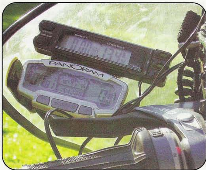
A close-up of the bike's cycling computer as well as the battery/panel meter that monitors the battery charging system.
