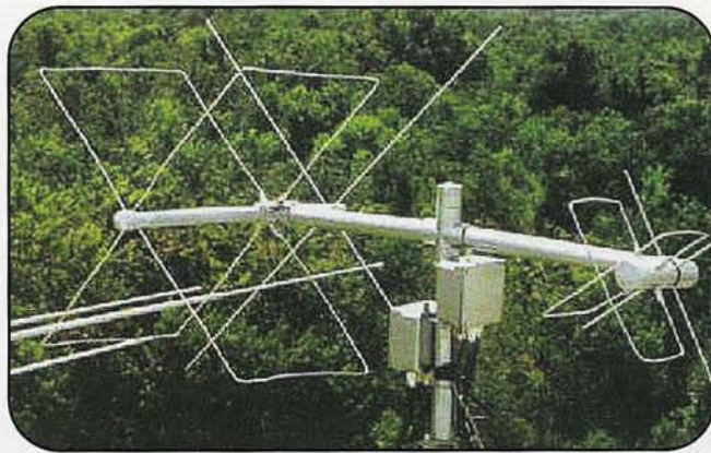
Photo 5. A Texas Potatomasher II, also by K5OE. The 2-meter element is to the left; the 70 cm to the right. The array is rotated for azimuth only. This design represents a great compromise between a stationary and directional array. (Photo courtesy K5OE)
