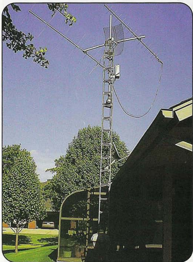
Photo 1. The author's satellite array. Just 20 feet high, it provides plenty of ground clearance, is easily accessed for maintenance, and is hidden from the public street. (Photo courtesy WA9AFM)
