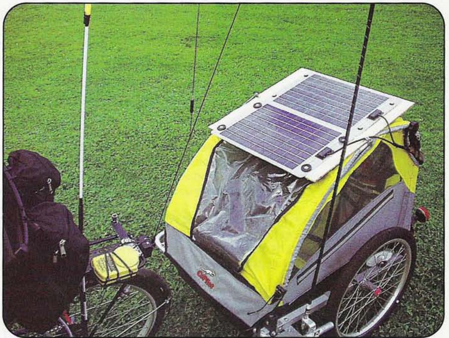
Have solar will travel! These two Solarex MSX-10L panels produce about 1.2 amps at 17 volts in full sunlight. Note the Tripmate GPS receiver used with the APRS and ATV systems in the lower left of the image.
