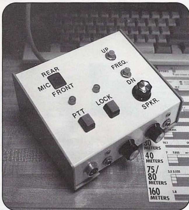
Photo 1. The Station Controller gives the operator independent push-to-talk and frequency up/down controls, plus a choice of microphones and other options. (Photos by AF1US)
