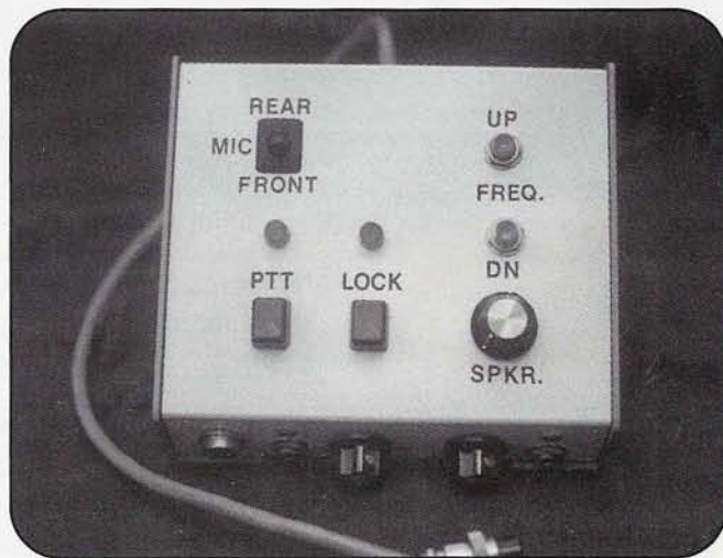
Photo 2. Top-panel controls on the Station Controller allow one to select a microphone, key the transmitter, change frequency, and even control speaker volume.
