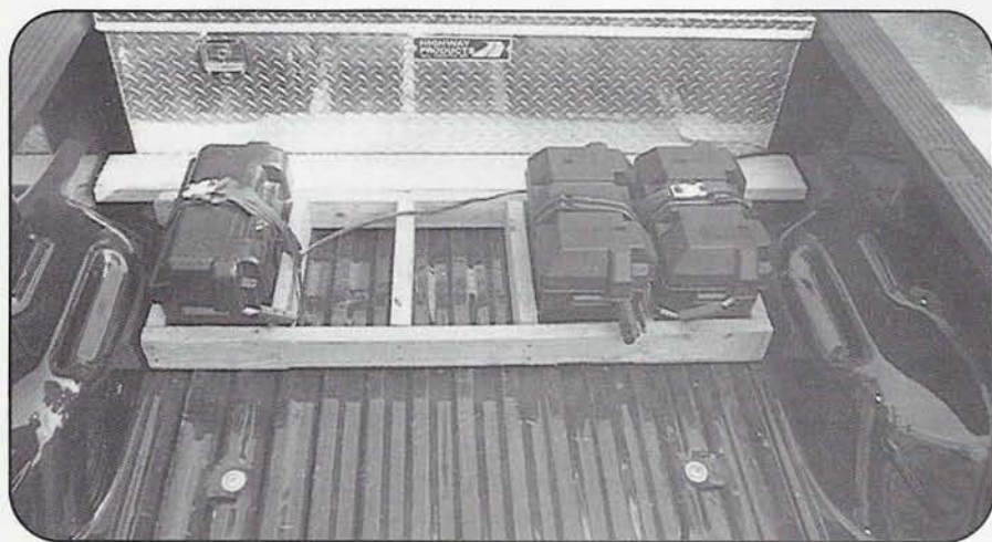
A simple 2x4 wooden frame keeps the auxiliary batteries in place. Plywood bottoms in the outer sections use the weight of the batteries to anchor the frame, along with a 2x6 crosspiece.
