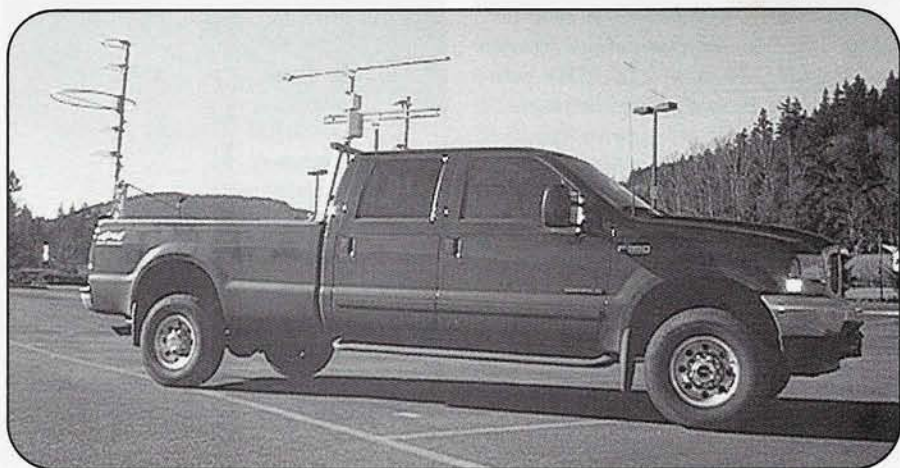
The W7DHC rover with 50, 144, and 222 MHz loops mounted on the rear mast. Mounted on the "headache rack" are 432 MHz loops, plus a 903 MHz Yagi, 1296/2304 MHz planar antennas, and a 3456 MHz loop. (Photos by the author)
