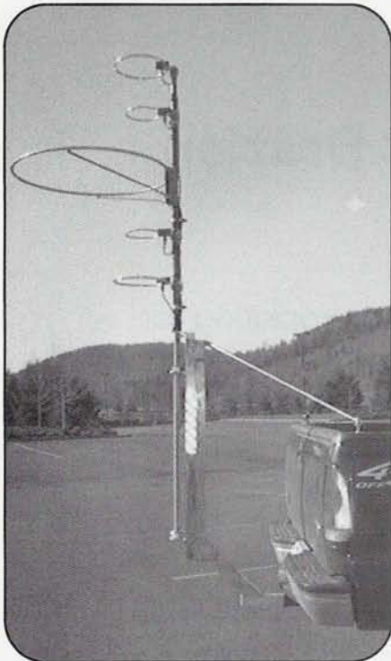
Loop stack on rear-mounted tilt-over mast with 144 and 222 MHz pairs mounted above and below the single 50 MHz loop. The stack can be removed easily and replaced with a mast for Yagis when needed.
