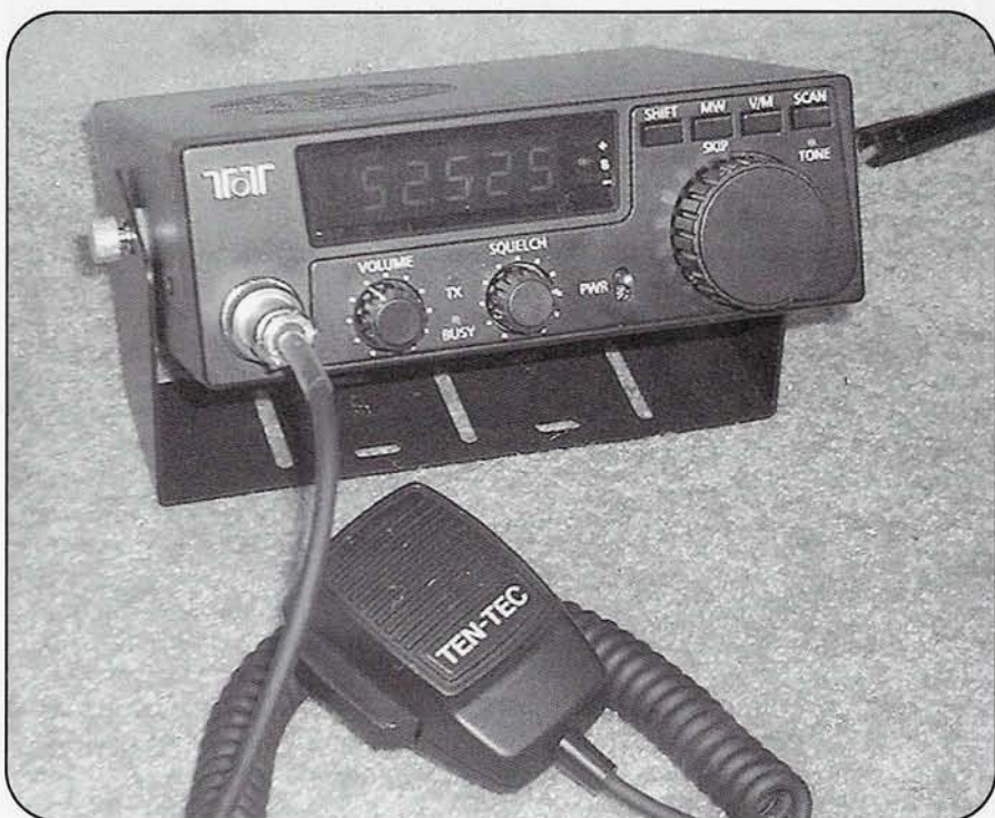
Photo A. The T-Kit 1260 6-meter FM transceiver with mobile mounting bracket and hand microphone.
