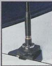
COMET CQ-5M Low-profile, "quick-disconnect" trunk lip mount. For quick storage, or theft prevention, the antenna and connector are disengaged from the mount base with the release of a lever. Offset washers provide up to 17 deg vertical antenna adjustment. Includes 16'9" of deluxe cable, 18" of mini RG-188A/U style coax for easy entry thru the weather seal. Gold-plated SO-239/PL-259 conns.
