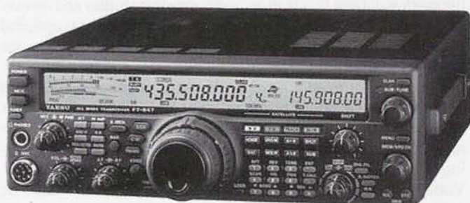
Photo 3. The "Earth Station," as Yaesu calls the FT-847, was the first amateur radio transceiver to cover HF, 6 meters, 2 meters, and 70 cm. The 847 replaces the "satellite workhorse," the FT-736. The 847 is the only amateur radio transceiver to include the Alaskan emergency HF frequency. (Photo courtesy RigPix)
