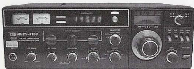
Photo 6. The FDK (later KLM) Multi-2700 was the first amateur radio transceiver designed with satellite communications in mind. It's a 2-meter all-mode transceiver and 10-meter receiver all in one box. Although there was no interface between the 2-meter and 10-meter units, the single-container design led the way to the satellite rigs we enjoy today. (Photo courtesy RigPix)
