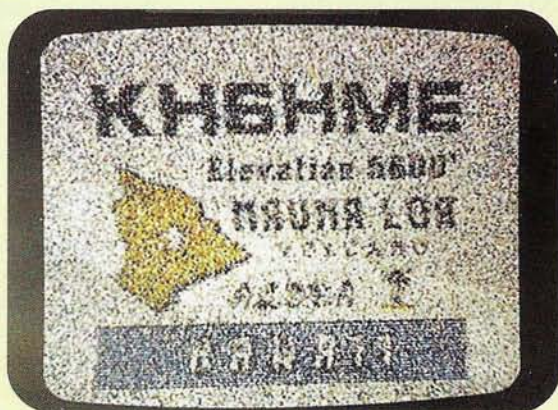
An ATV signal on 426.250 MHz over a 2500 mile path.
