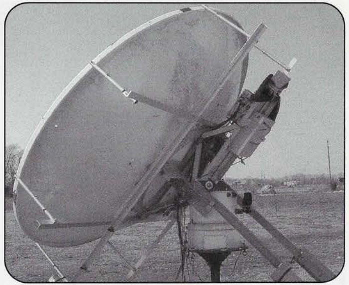
Photo 4. Back structure for the 3-meter dish at W5LUA.
