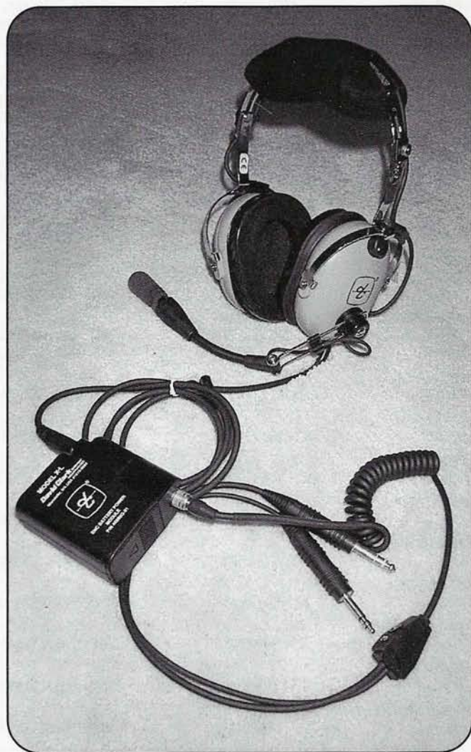
The David Clark Model H10-13X headset rests behind the electronic noise-canceling module (Model X-L) with the stereo phono plug for the earphones and the aviation microphone plug.
