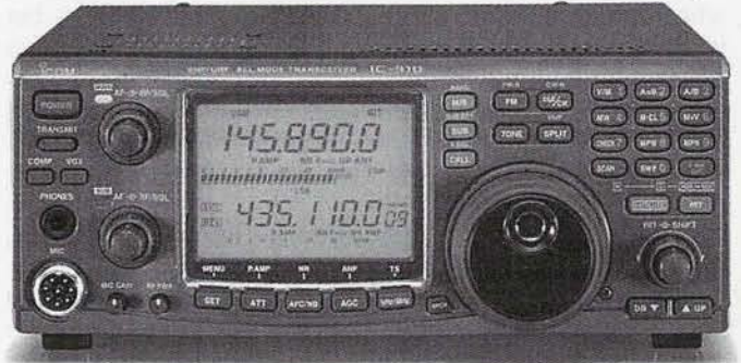
Photo 1. The ICOM IC-910H is the latest offering from ICOM for satellite work. The 910H is 2 meters/70 cm only with 1.2-GHz option. It replaces the IC-821H. The “set-and-forget” features are menu driven, with frequently used functions on the front panel. The small size and light weight are great for portable operation or limited desk space. (Photo courtesy RigPix, <www.rigpix.com>)
