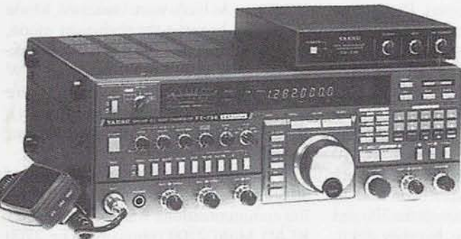
Photo 4. Although no longer produced, the Yaesu FT-736 is the workhorse of the satellite community and has a very loyal following. It comes standard with 2 meters and 70 cm, with full duplex as a standard feature; 6-meter-, 220-MHz, and HF boards are options. An ATV adapter is also available. (Photo courtesy RigPix)
