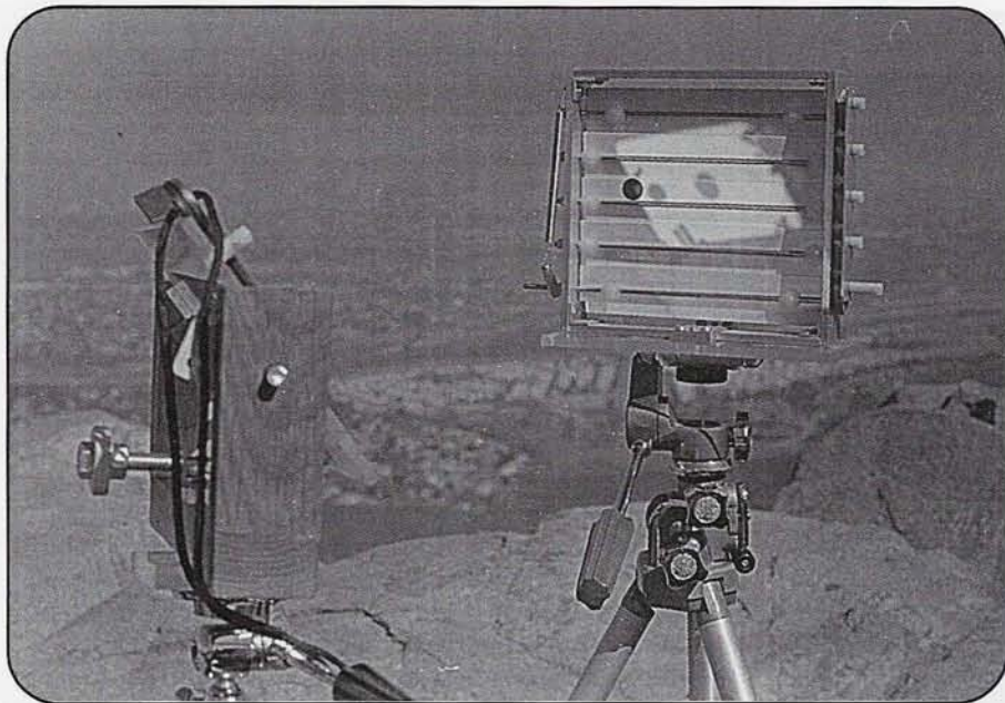
The mirror aimer (left) and shutter (right) with the shadow spot used for alignment visible on the louvers.
