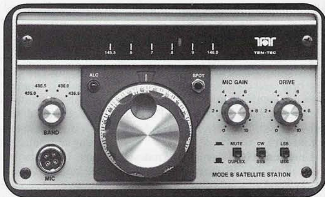
Photo 5. The Ten-Tec 2510B was produced in the early 1980s. The first edition, the 2510, had "operating" issues and was called back and redesigned, resulting in the 2510B. The unit was configured with a 2-meter/10-meter converter and 70-cm 10-watt transmitter. A PTO circuit allowed auto-tracking. It was a clever design for its day. (Photo courtesy Ten-Tec)
