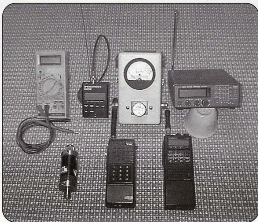
The author's test equipment. Top, left to right: multimeter, counter, bird equivalent wattmeter, scanner. Bottom, left to right: 10-dB, 10-watt attenuator; 144-MHz HT; and 220-MHz HT.
