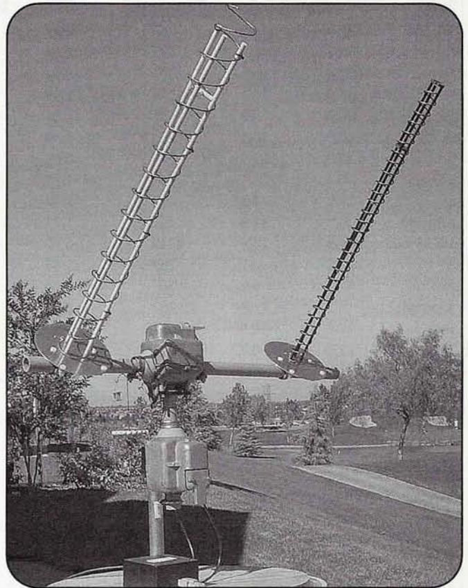
Photo 1. The author's two helical antennas rotated by U-100 rotors.
