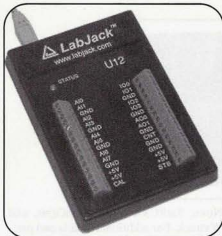
Photo 2. The LabJack U-12 USB-base multi-functional data acquisition and control device.
