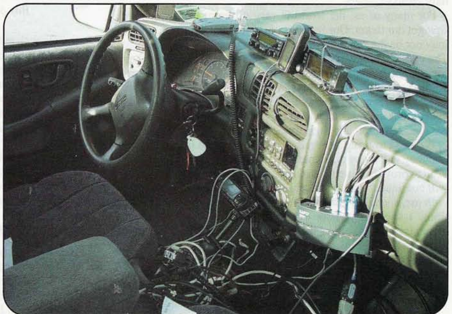
Recovery vehicle wired for 2 meters, 70 cm, HF, and APRS.
