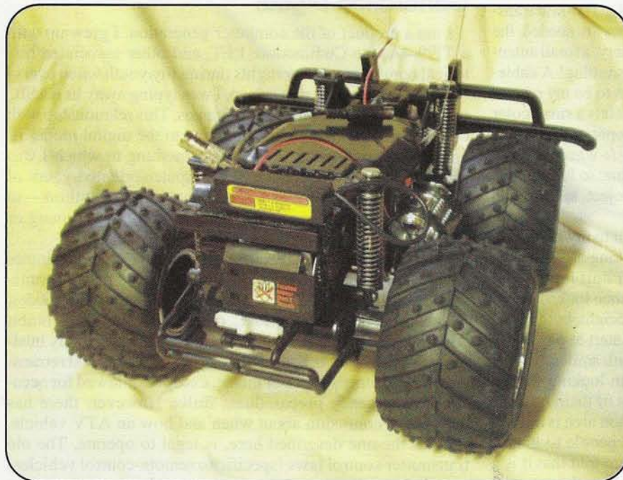
Exposing the bare "frame" of the truck, you can see the Videolynx transmitter attached to the rear of the truck above the motor using Velcro®.
