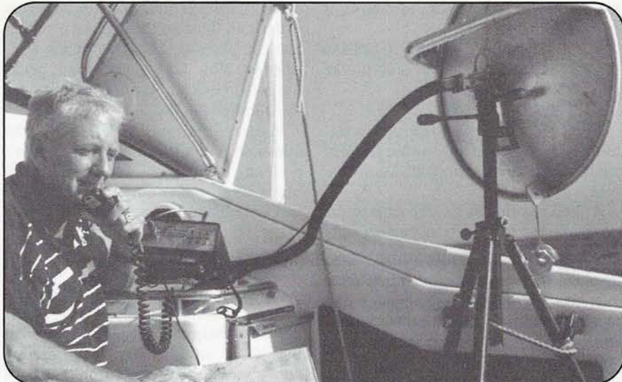
WB6NOA operating the microwave radio system at 100 miles out. The best DX was 450 miles with 100 milliwatts.
