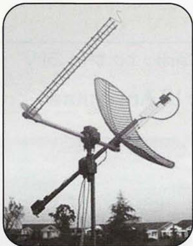
Photo 7. The SatEL Az/El system includes not only the controller, but also the rotors.
