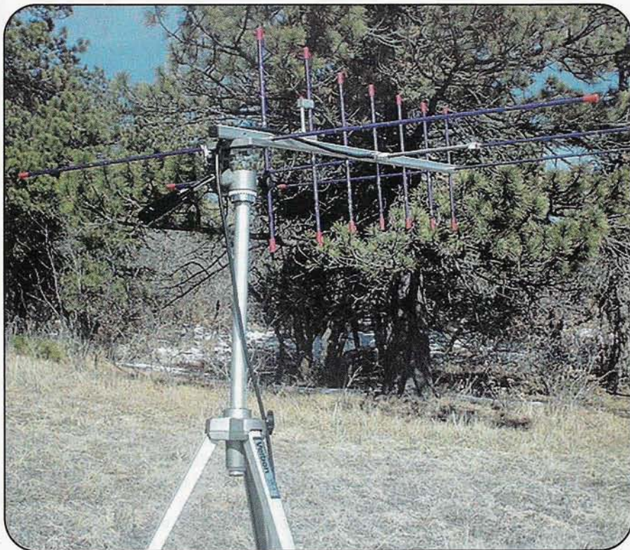
Photo C. Arrow dual-band 2-meter/70-cm antenna mounted on a camera tripod. (Photo by KØNR)
