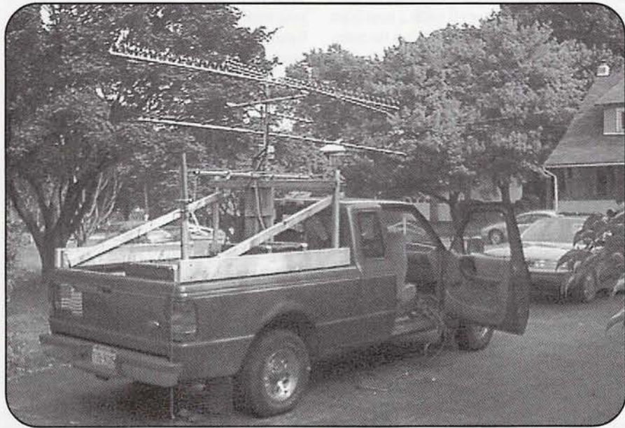
Photo A. Wood was used to create an antenna mount for the bed of K3YWY's 1993 Ford Ranger.
