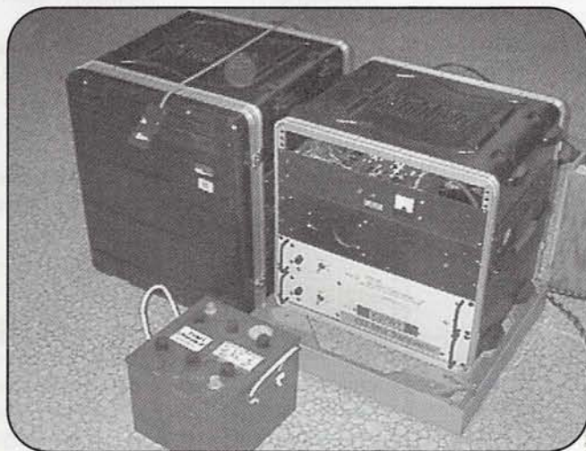
Photo B. The equipment configuration. The two travel racks add portability and protection from the weather. The green military battery that we use is shown in the foreground.
