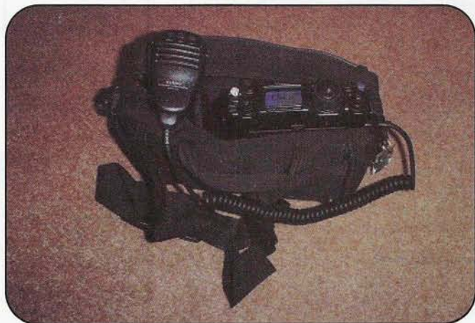
Photo B. The Yaesu FT-817 fits snugly inside a combination fanny pack/over-the-shoulder bag, ready for portable operation. (Photo by KØNR)
