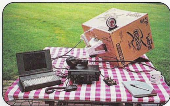
Photo F. Tony Monteiro's +20 dBi waveguide horn for 2401 MHz AO-40 satellite reception. (AA2TX photo)
