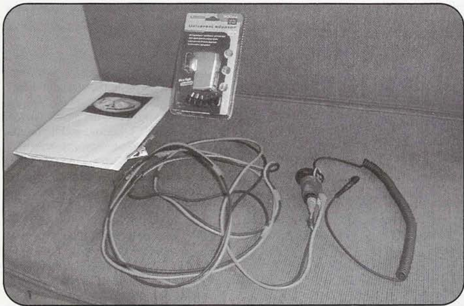
Here you can see the homemade charging harness and the proper wall charger. The store-bought unit could only be used with an extension cord because of the inaccessible power point.
