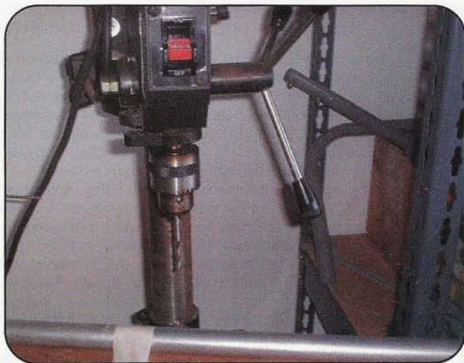
Photo C. Drilling the antenna boom.
