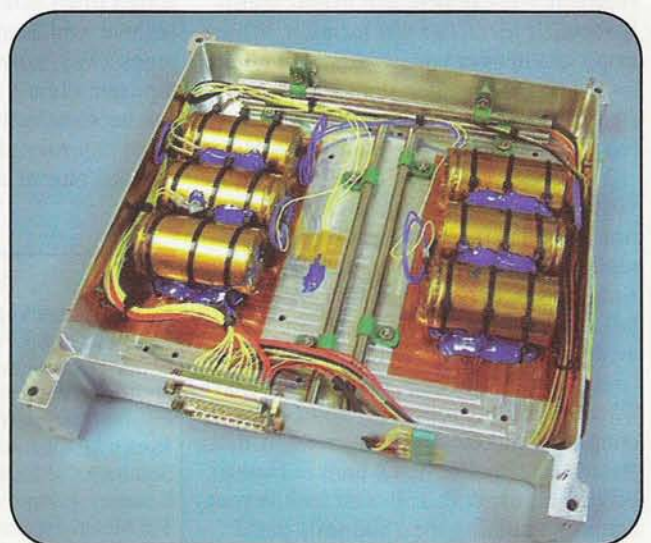
Photo G. Battery tray.
