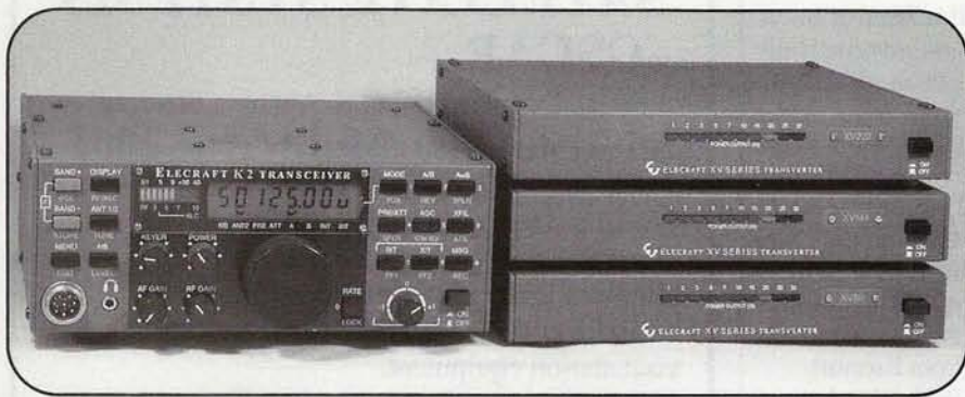
The K2 with the XV50, XV144, and XV222 transverters stacked at the right. (Photo courtesy Elecraft)
