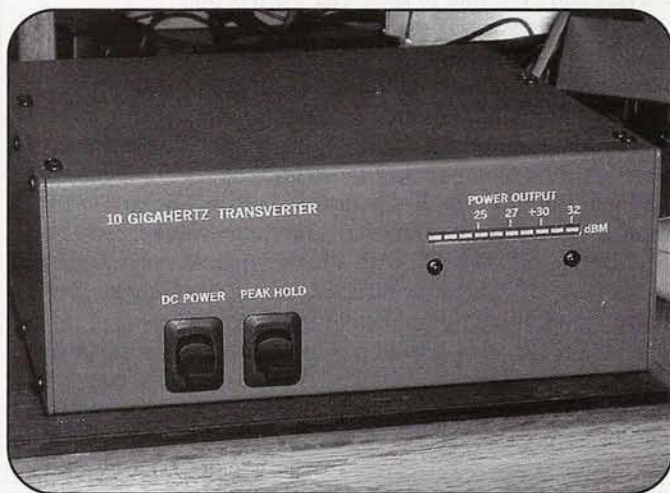
Bob Friess, N6CM, built a 10-GHz transverter for the K2 in an EC2 chassis. (Photo courtesy N6CM)
