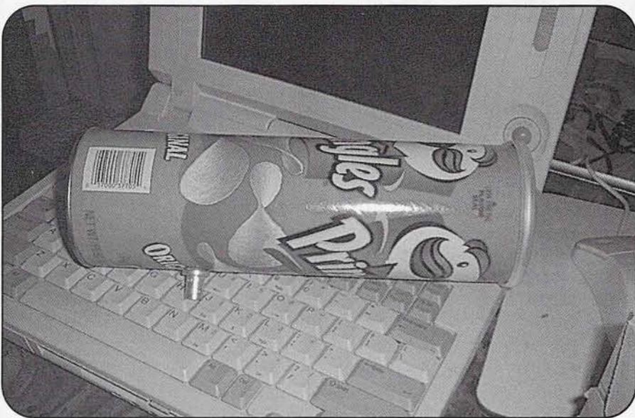
Photo A. Pringles®-can antenna and laptop.
