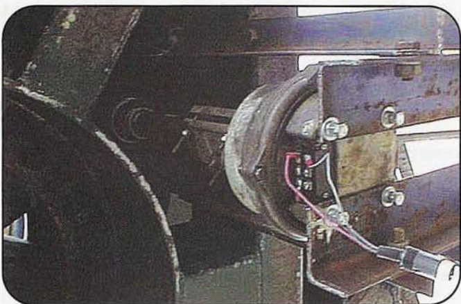
Photo 10. Using an Alliance HD73 rotator as a temporary azimuth rotator.
