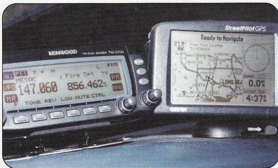
The Garmin Street Pilot® was the choice to tie into the ham APRS.
