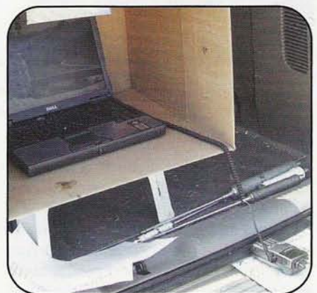
Photo 1B. Notebook computer in "sun shield" connected to the Kenwood TH-D7.
