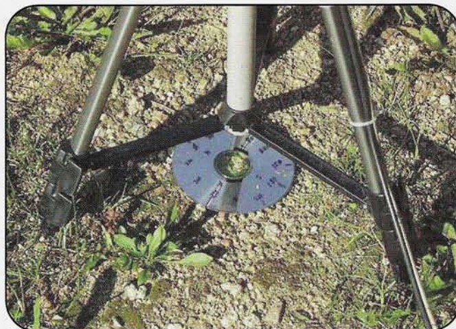
Photo 6. As an alternative, the azimuth direction-indicator disk can be placed on the ground.
