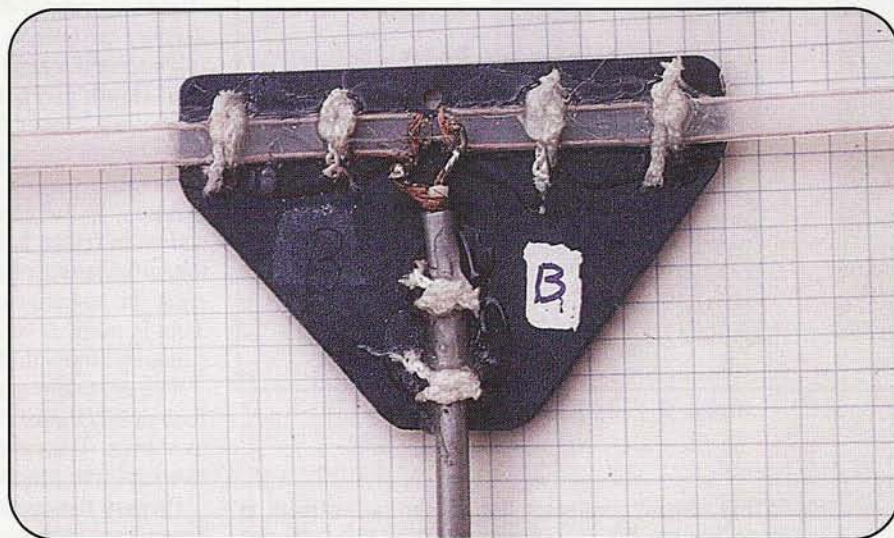
A close-up of the completed antenna center area.
