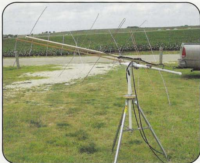
Photo 11. Working satellites from the "cotton patch"—WA5VJB's circular-polarized 2-meter, 4-element "Cheap Yagis" and 10-element, 70-cm "Cheap Yagi" on W5IU's "Cheap Positioner."
