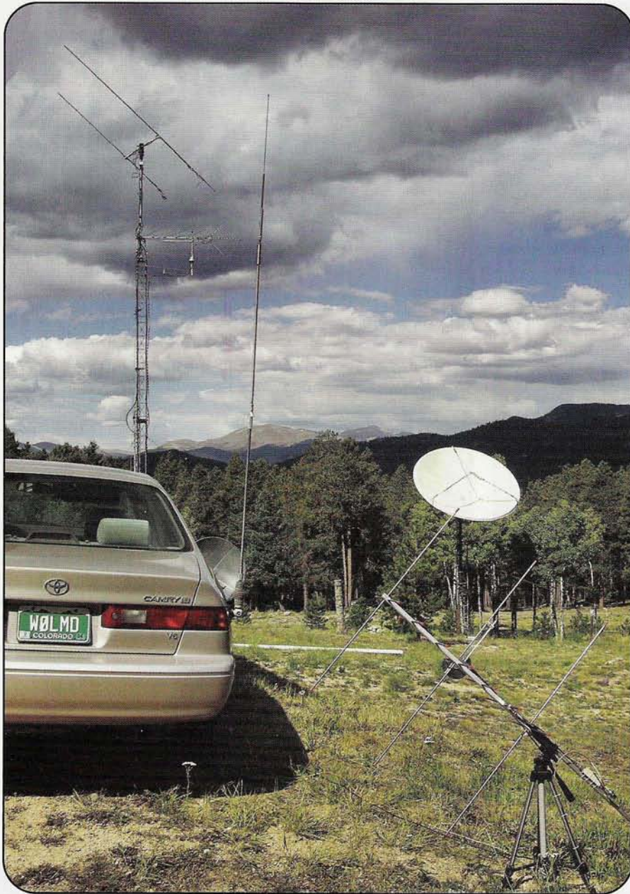
Photo 8. With this setup on his car, the author should easily be able to pick up AO-51 QSOs as soon as the satellite rises above the horizon.
