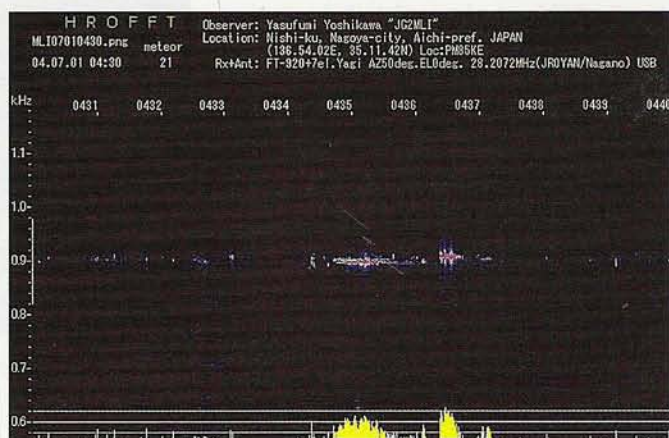
Figure 4. A plot of signals observed by radio meteor observation in Japan. (Courtesy of The International Project for Radio Meteor Observation)
