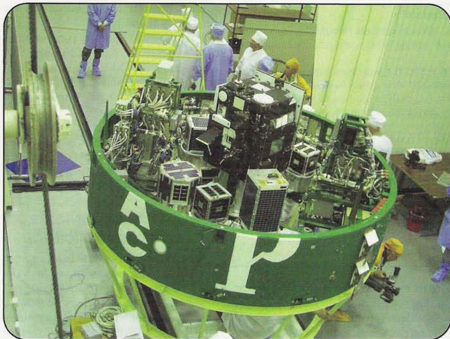
All satellites for this launch are now positioned on the dispenser plate. ECHO is in the foreground.
