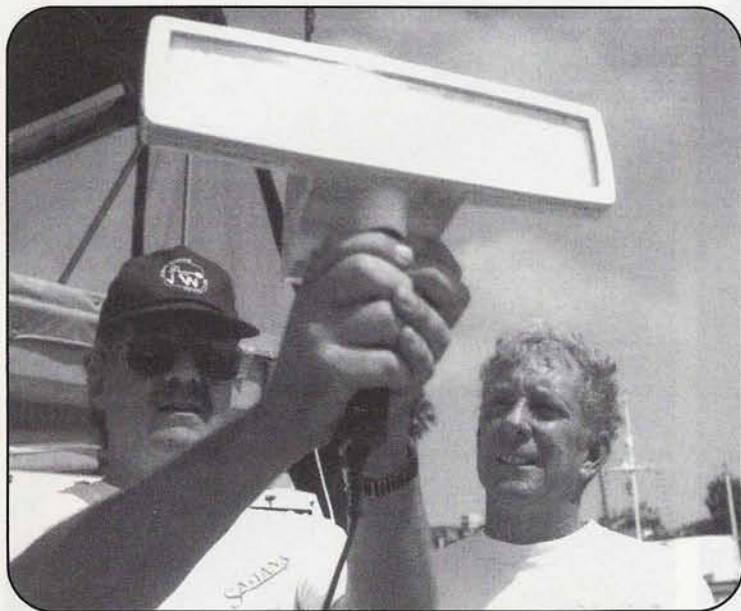
WB6NOA looks on during tests of a 10-GHz phased array antenna system.
