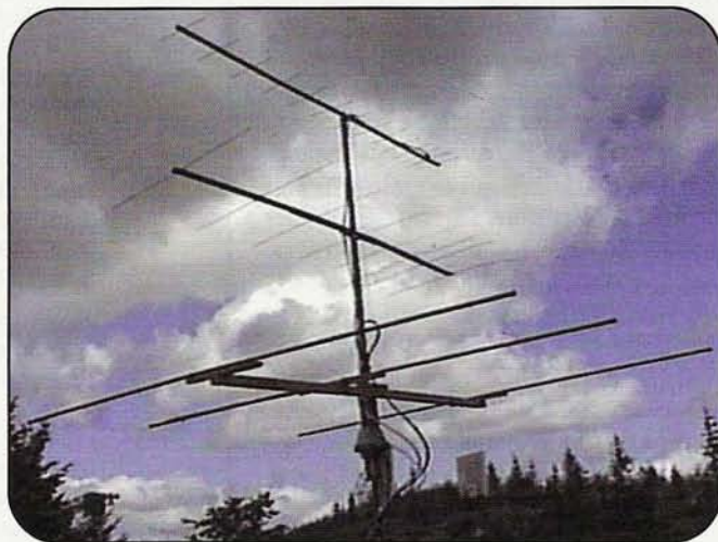
Photo C. A stack of homebrew Yagi antennas built by N3EG. (Photo courtesy N3EG)
