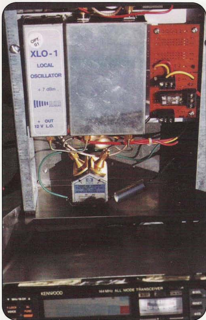
The SSB Electronics 10-GHz transverter with 2.2 watts output on X-band. The SMA connections are the 10-GHz way of "plumbing" the modules and 12-volt TR relay.
