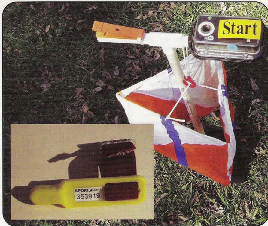
Photo C. E-punch is replacing the old multi-pin punches at formal events. The e-stick (inset) is worn on a finger so that the competitor merely has to make a fist and briefly dip the stick into the control station next to the flag.
