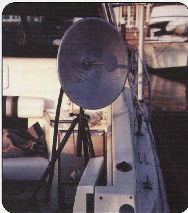
A dish antenna with Cassigrain feed for 10,000 MHz.
