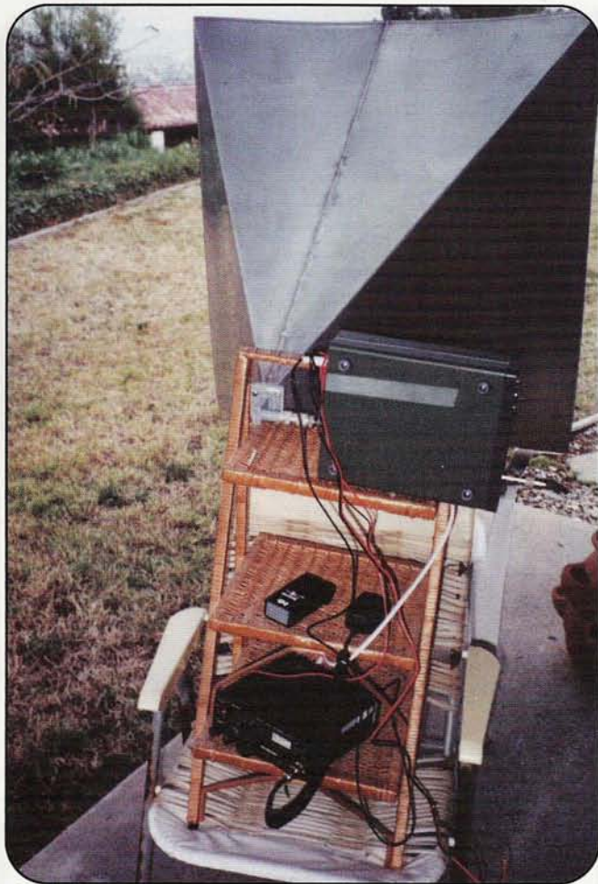
A homebrew 10-GHz monster horn with the transverter (green box) attached directly to it.
