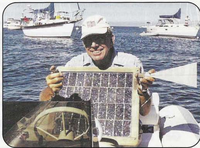
Tom, N6DCL, uses a horn antenna with 1 watt over a 100-mile path.
