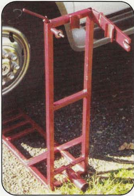
Photo H. Some shoot 'n' scoot rovers use an antenna base that is secured to the ground by driving a vehicle's front tire onto it. The tower is bolted quickly to the pre-existing hinges and then tilted up from the base. The example shown is from KL7JR.
