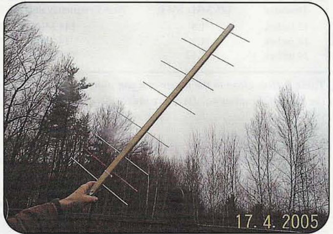
Photo C. Building Yagi antennas on hockey sticks. (Tnx to Denis in Quebec)
