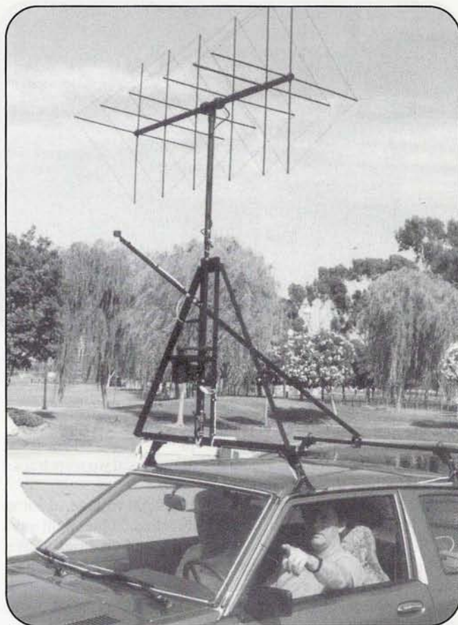
Unusual rotating VHF RDF beams are a common sight in southern California. JaMi Smith, KK6CU, built this motorized version in the 1990s. It turns at constant 6 rpm and displays bearings in polar form on a storage oscilloscope.
