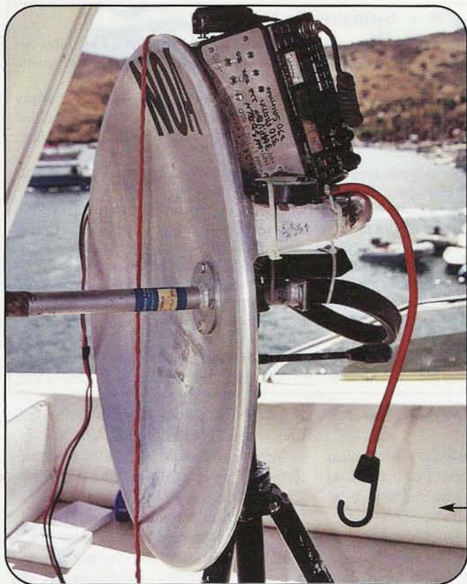
WB6NOA's 10-GHz maritime mobile setup. One watt and 300-plus miles to Mexico makes him smile!
