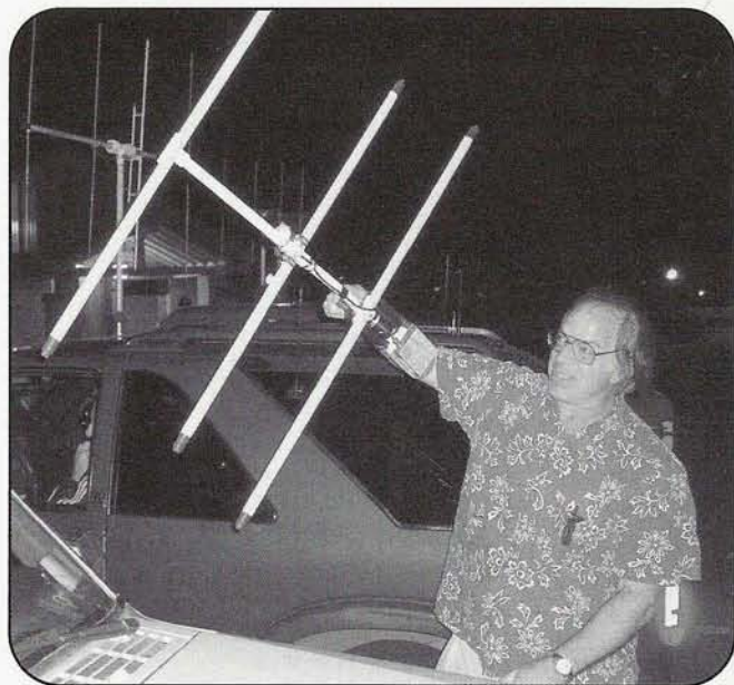
Getting back into the game, David Pepper, WA6TWA, sniffs out a hidden transmitter using a state-of-the-art 2-meter RDF set from Australia. (All photos by Joe Moell, KØOV)
