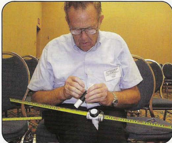
At the ARRL Southwestern Division Convention's RDF workshop, David Danner, K6AIX, of Canoga Park, California assembled a 2-meter tape-measure Yagi.
