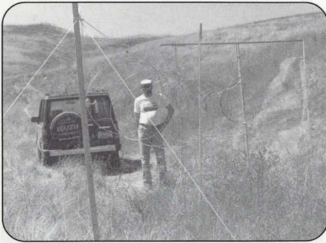
Huntmasters often use exotic antennas to help their signals bounce in the southern California hills. Gary Holoubek, WB6GCT, set up this 30-foot circularly polarized 2-meter helix for a Saturday night hunt.
