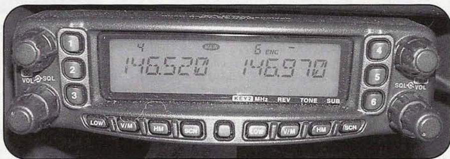
A VHF/UHF transceiver set up for dual receive on the 2-meter band, with one receiver set to 146.52 MHz.
