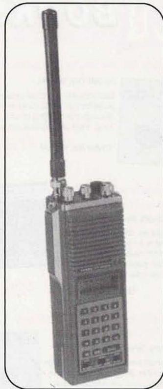
Photo C. The Yaesu FT-208R was an early synthesized 2-meter handheld transceiver. (Photo courtesy of the < www.rigpix.com > website)
