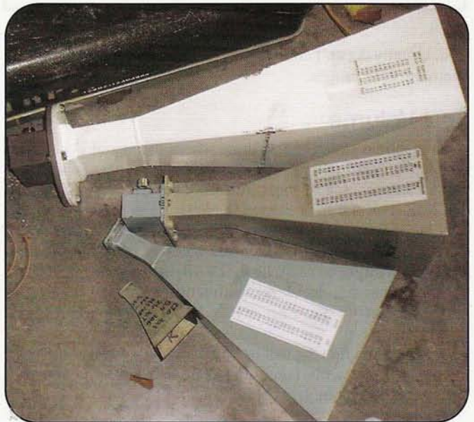
Photo D. Horn antennas are simple, hard to damage, and broadband, and their gain can be calculated with good accuracy. Thus, they make good reference antennas.
