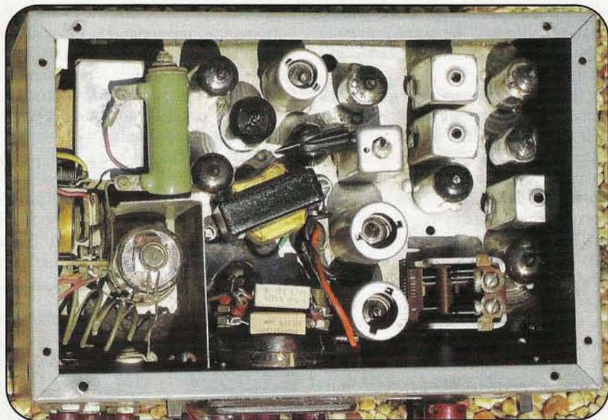
Top view of the now restored transceiver. Notice the new shunt resistor on the back of the panel meter.
