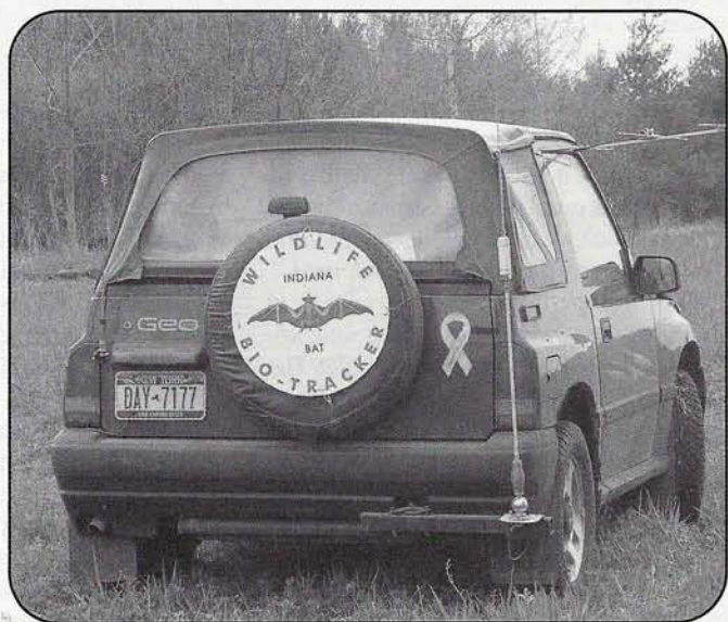
WN8Z's Geo outfitted for bat tracking. When cruising for signals, Pat has Yagis aimed left and right with a scanning receiver on each one, plus a third receiver on a vertical whip.
