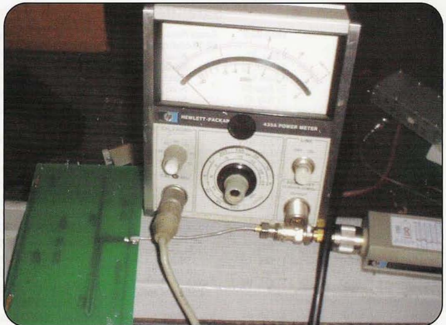
Photo B. The Hewlett Packard 435A power meter. Using a power meter and a test antenna is possibly one of the simplest ways to measure antenna gain.
