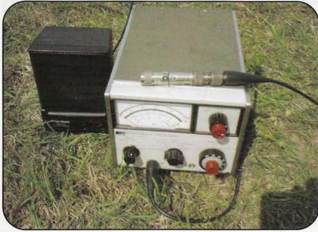
Photo C. The HP 415E is a tightly tuned 1000-Hz audio meter.
