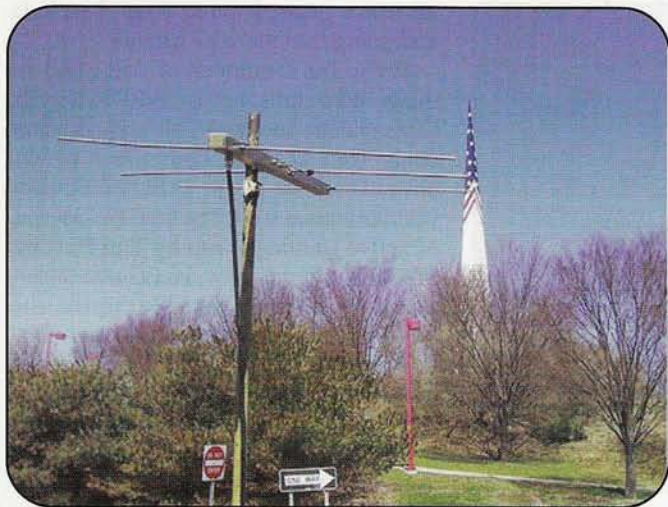
A three-element, 2-meter Yagi is a small antenna that is easy to set up for portable operations. Here is the setup that WB2AMU employed in searching for 2-meter tropo activity near a 250-foot hill that also features a public park with a Vietnam War monument. (Photo by WB2AMU)
