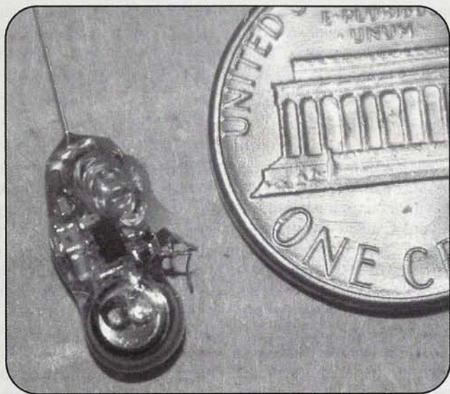
A radio tag for a bat next to a U.S. penny for size reference. (Photo courtesy of Carl, AB2SI)
