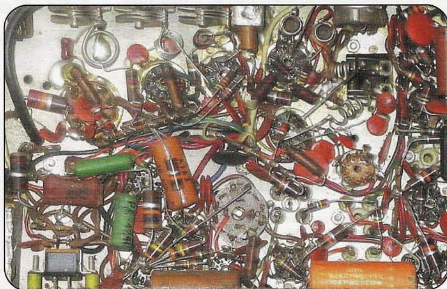
Bottom view of the restored transceiver. One can easily see how printed-circuit boards have simplified internal packaging of today's radios.
