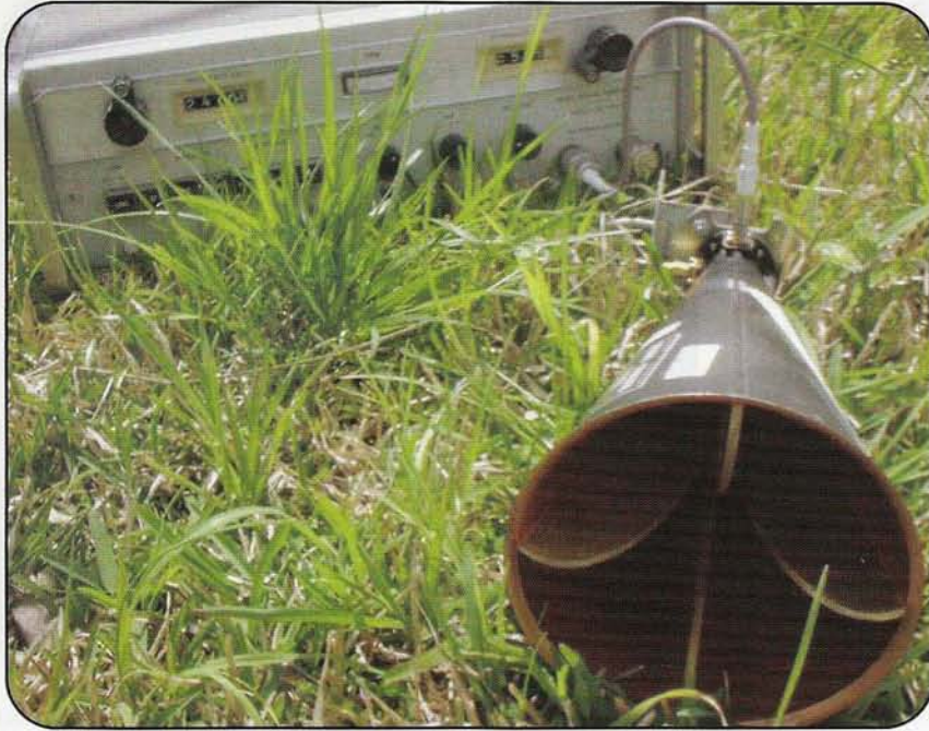
Photo E. the author's favorite setup is a wide-band antenna and a wide-band signal generator.
