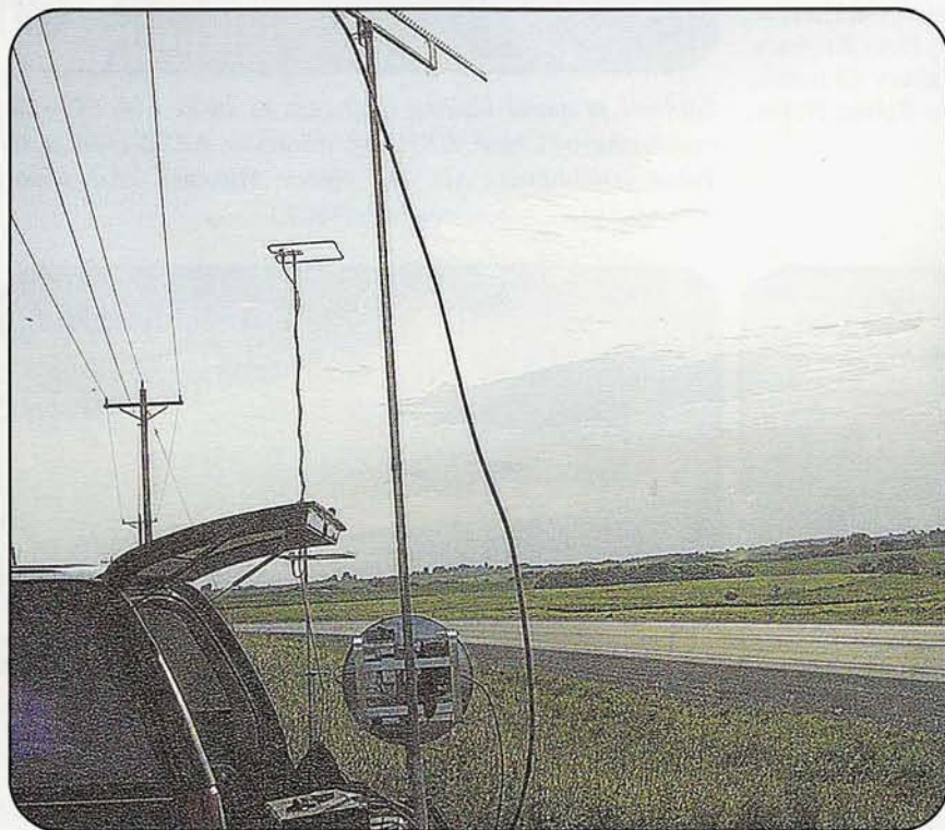
Photo C. NØDQS operated portable from Wisconsin, EN42nx. Note direct heading for the dish and skew path to the north for the 3.4-GHz loop antenna. The minor precipitation clouds can be seen in the distance.
