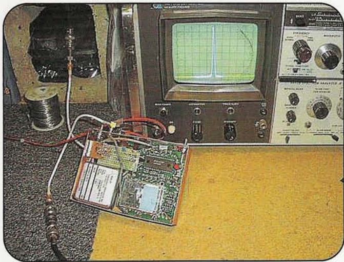
Photo B. Top of the synthesizer showing added perf-board transistor amp and 10-MHz TCXO used to provide clock input to the synthesizer via a new, added 7490-divide-by-10 chip.
