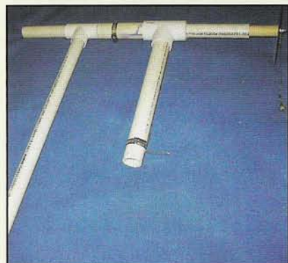
Photo C. Assembly of the horizontal boom and elevation bearing.
