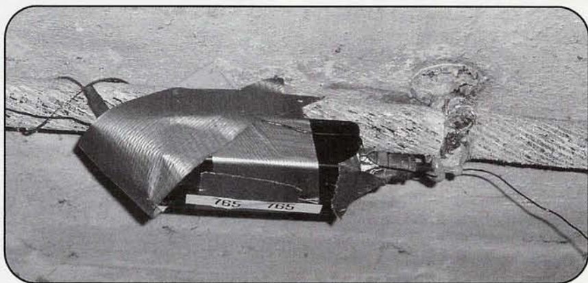
Photo 6. One of the 16 Hamcon 2003 ROCA transmitters was in the ceiling of an old Fort MacArthur tunnel. That made its signal highly directional. (Photo by KØOV)
