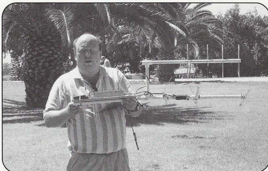
Photo 7. Travis Wood, AE6GA, had the most unusual RDF setup at the Hamcon ROCA. The circular-element quad on top was for close-in hunting on fox harmonic frequencies. (Photo by KØOV)
