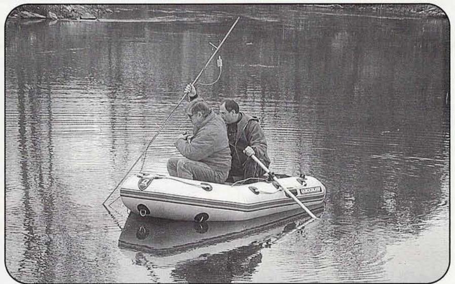
The author (left) and Ritch Williams, KA9DVL, try to locate the transmitter in the water using a submersible probe attached to a 10-foot pole.
