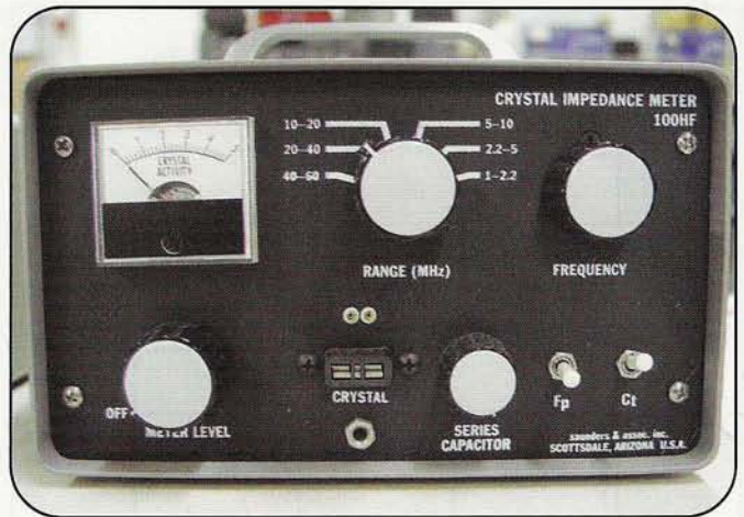
Photo E. The 100HF, an HF instrument used for production testing of crystals.
