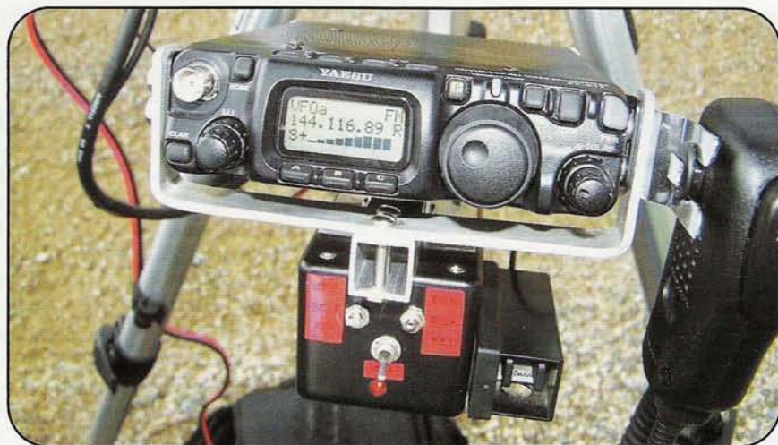
Photo H. The FT-817 (144 MHz IF radio) showing full-strength rain-scatter FM signals at 45 miles.
