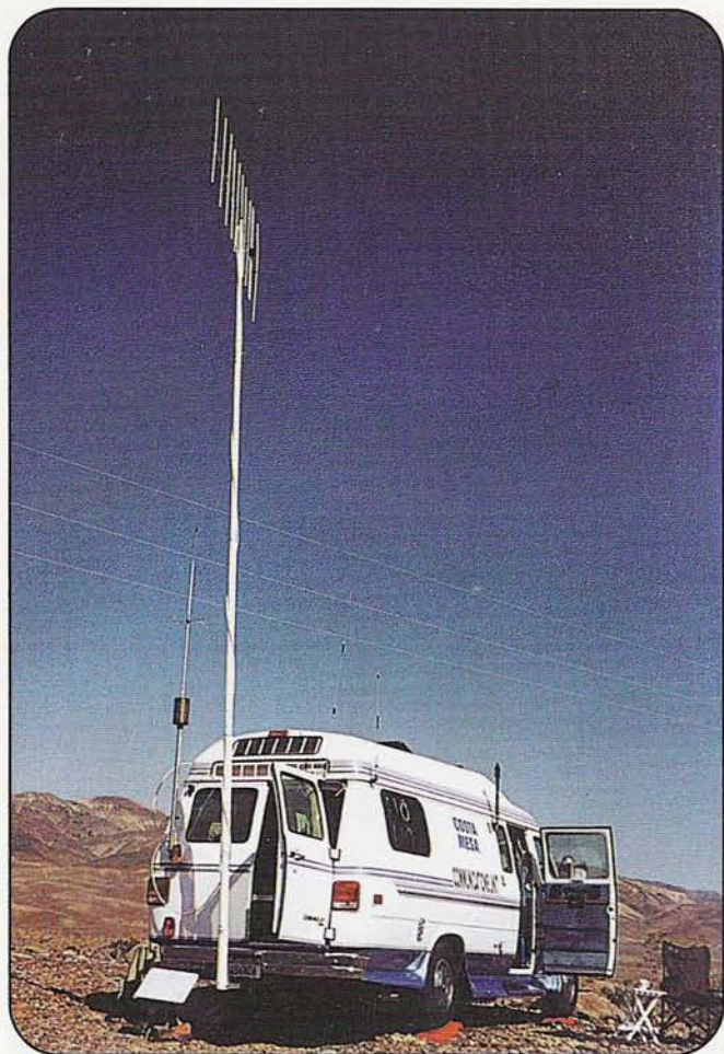
The flagpole will hold some large VHF and UHF antennas without “noodling.”
