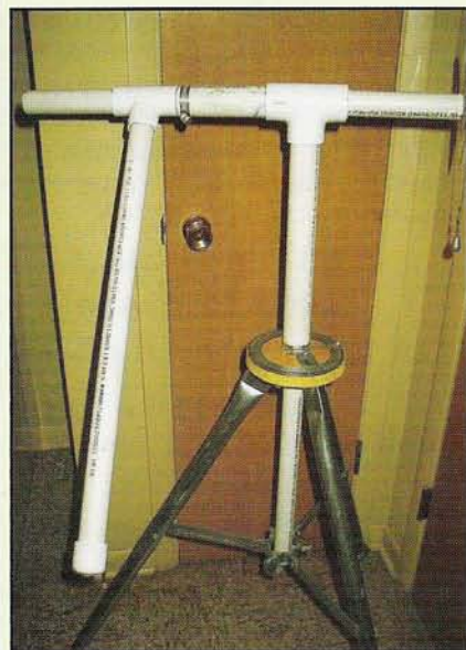
Photo A. The completed Az-El Antenna Positioner assembly mounted on a tripod. The dish mounts on the right and the Yagi on the left. (Note azimuth pointer.)
