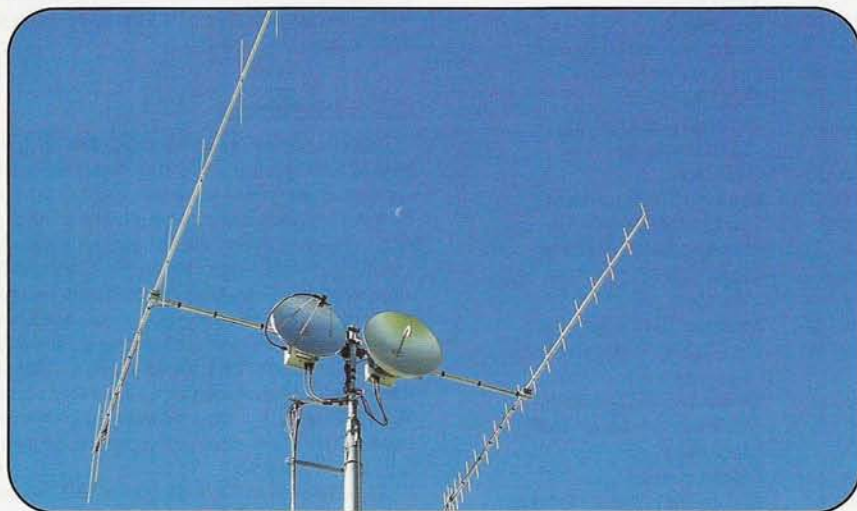
Photo A. Left to right: A 9-element 144-MHz Yagi, 5.7-GHz dish, 10-GHz dish, and 18-element 70-cm to 432-MHz Yagi.
