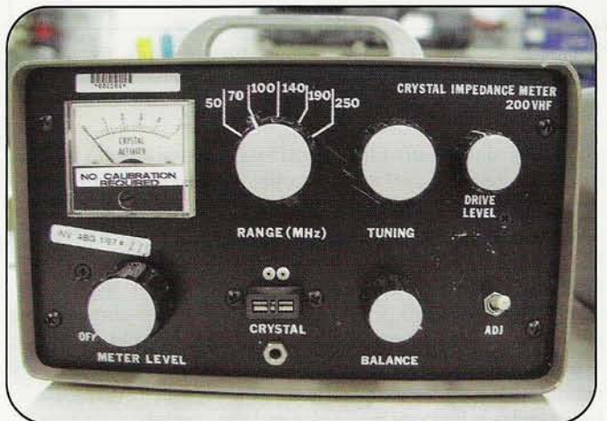
Photo F. The 200VHF, a VHF instrument used for production testing of crystals.
