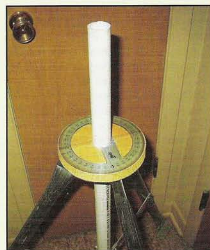
Photo D. RadioShack tripod showing the azimuth bearing post and azimuth indicator.
