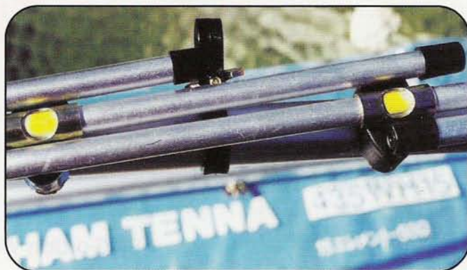
The yellow paint on the fold-up MASPRO antenna is for element centering.
