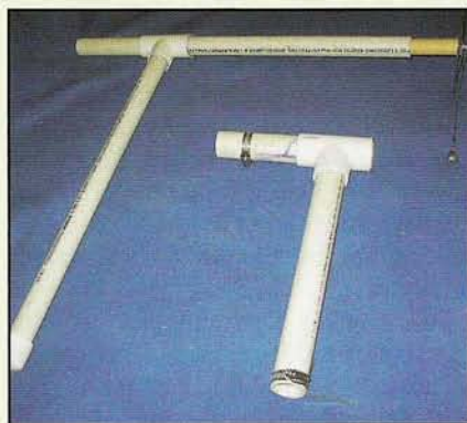
Photo B. The horizontal boom and positioner arm on the left showing the wooden dowel and elevation indicator assembly, and the elevation bearing assembly on right. (Note hose clamps for friction adjustment.)
