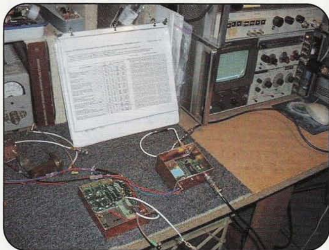
Photo C. The modified synthesizer operating at 2688 MHz on John, WB2BYP's workbench with a spreadsheet in the background for programming the synthesizer.
