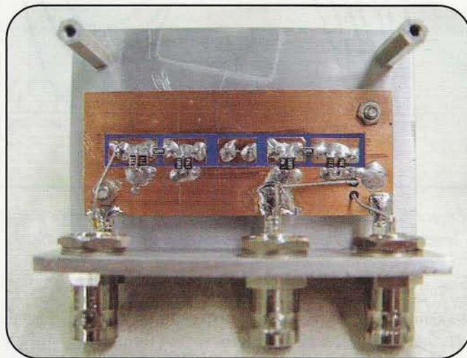
Photo D. A simple fixture for measuring crystal frequency with the cover removed.
