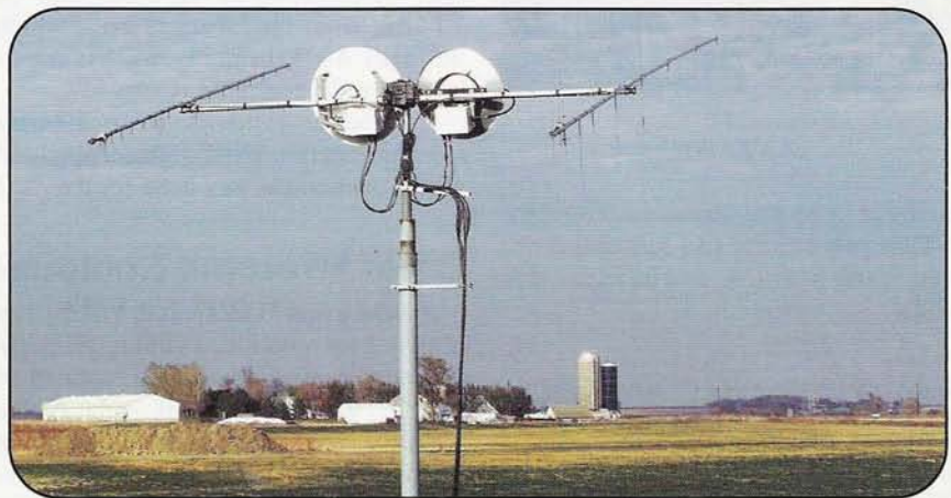
Photo D. The 5.7- and 10-GHz dishes at KMØT pointed toward EN34 with a bit of elevation.
