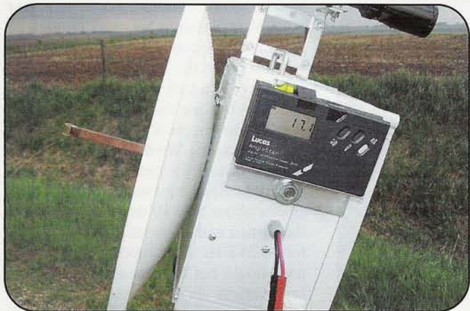
Photo G. Lucas DP45 AngleStar Digital Protractor showing 17.1 degrees elevation.
