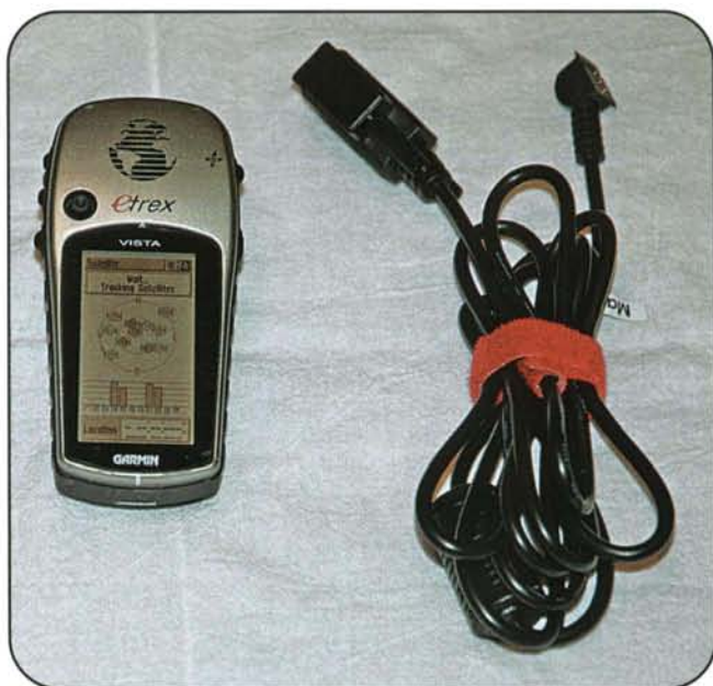
Photo 1. The Garmin eTrex GPS receiver and its cabling.
