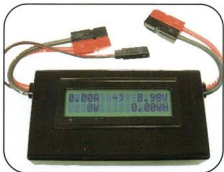
An Astroflight Whattmeter goes in line to measure a power system on the bench.
