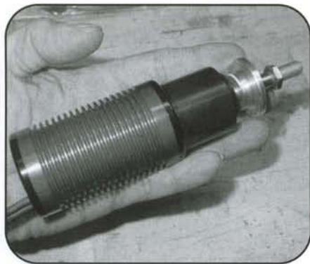
A big Hacker Gear motor that will put out well over a horsepower.
