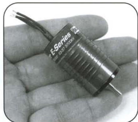
A Hacker Inrunner with about 200 watts of output.
