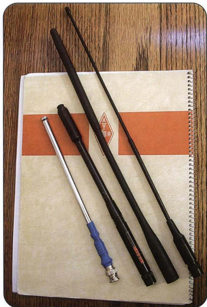
Photo D. Longer antennas provide better performance than the standard short "rubber duck" antenna.
