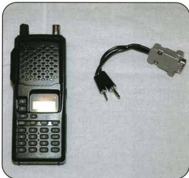
Photo 2. The ICOM IC-T2H handheld and the homebrew cable that connects to the TNC.
