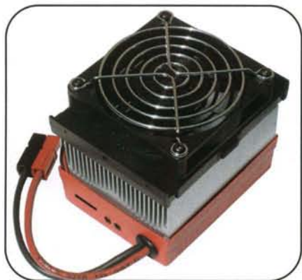
The West Mountain radio CBA will test just about any battery.
