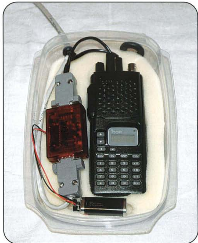
Photo 6. Radio, TNC, and cables neatly packed into the container, cushioned by a custom-cut piece of upholstery foam.
