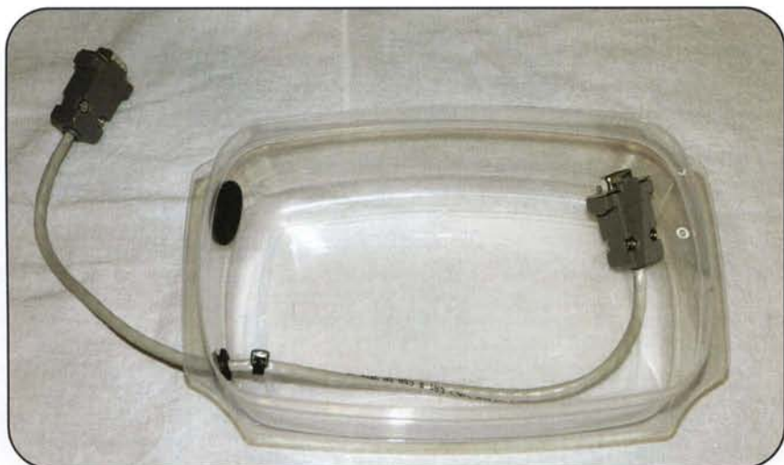
Photo 5. Modified container showing the installed homebrew serial cable.
