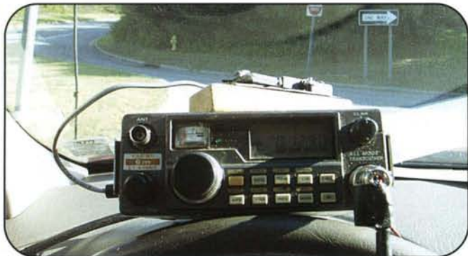
The FT-690 six-meter radio that WB2AMU used in the contest. The radio has 10 watts output, but that did not seem to be an issue with the good openings that were present.
