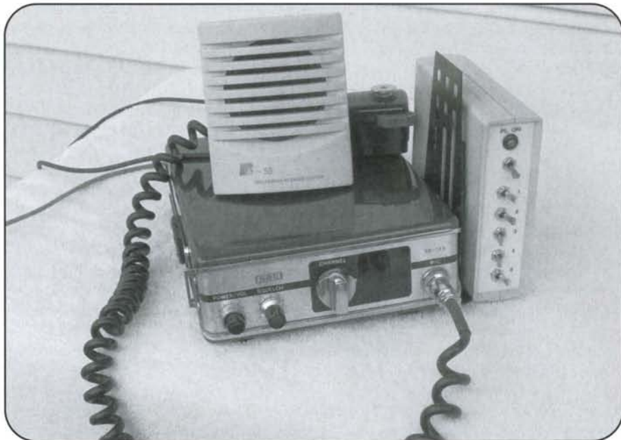
Photo 4. The renovated SB144 and the PL case look very attractive and make a nice addition to the shack.
