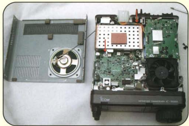
Photo B. Arrows point to the two screws holding the CPU/DSP module in place. Step 3 requires their removal. Step 4 requires the removal of the module.
