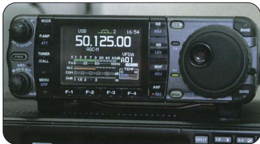
The IC-7000 has a beautiful operating display that shows frequency, memory information, power out, SWR, compression, and even radio temperature all at the same time.
