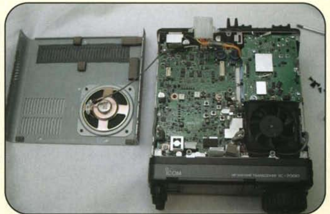
Photo C1. With the CPU/DSP module removed, the four 4094 shift registers are exposed. They can be identified by the Texas Instruments logo and part No. "HJ4094."
