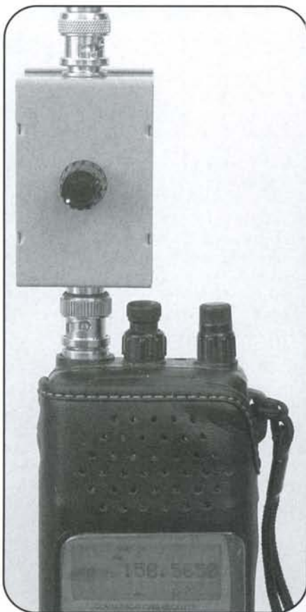
The Arrow Antenna offset attenuator box doesn't have labeling or calibration markings, but it's small enough to mount directly on the receiver.
