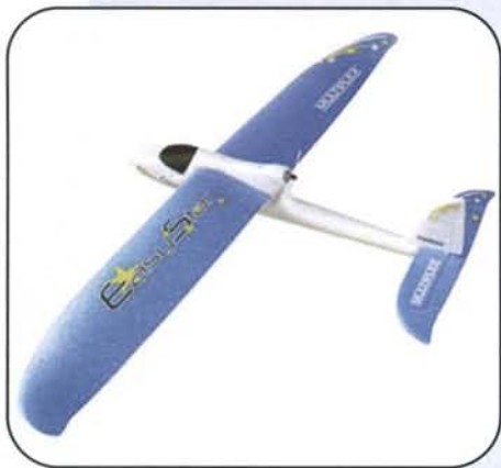
The Easy Star, a good foam trainer. Notice the prop out of harm's way.
