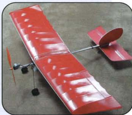
The simple, rugged, and inexpensive Slow Stick from GWS. Notice the aluminum-tube fuselage.
