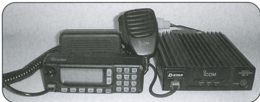
Photo B. The ID-1 transceiver is a 1.2-GHz transceiver that includes analog FM and D-STAR formats (DV and DD). (Photo courtesy of ICOM America)
