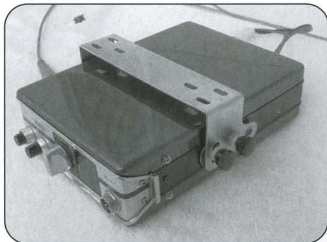
Photo 2. The mounting bracket arrangement
