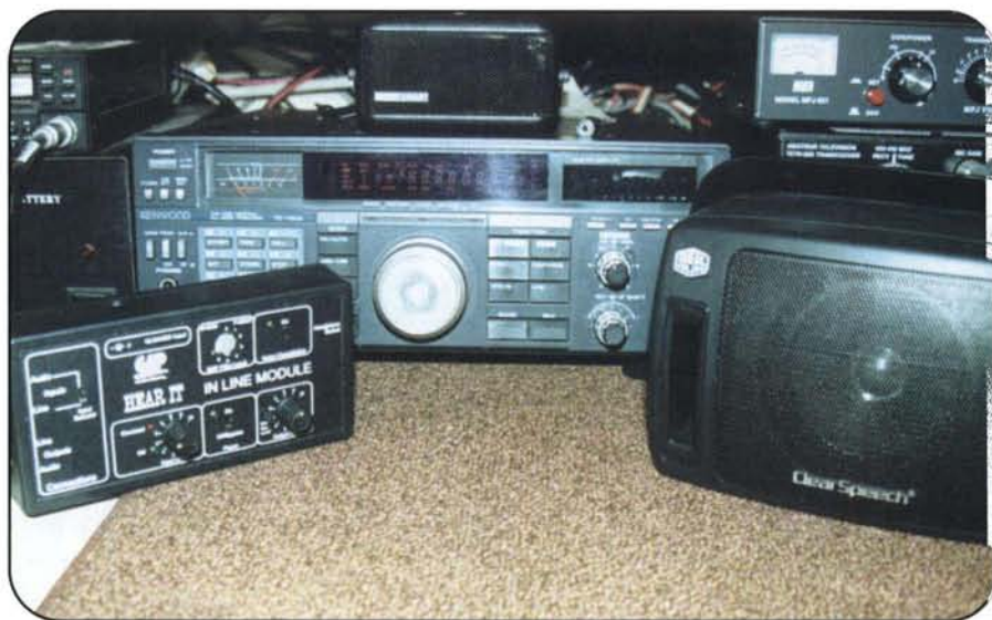
Shown here left to right are the GAP in-line DSP system, the SGC noise-subtraction DSP speaker (on top of the Kenwood TS-790), and the Heil Sound speech-amplified DSP speaker. All three systems worked well for monitoring beacons.
