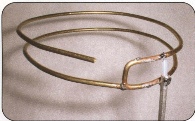
Photo H. Basic wire DDRR antenna.
