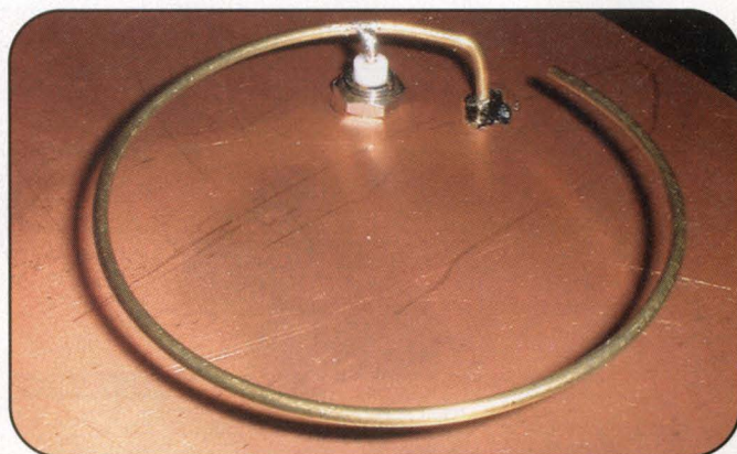
Photo A. The DDRR (Directional Discontinuity Ring Radiator) is a vertically polarized antenna. (All photos and artwork by the author)
