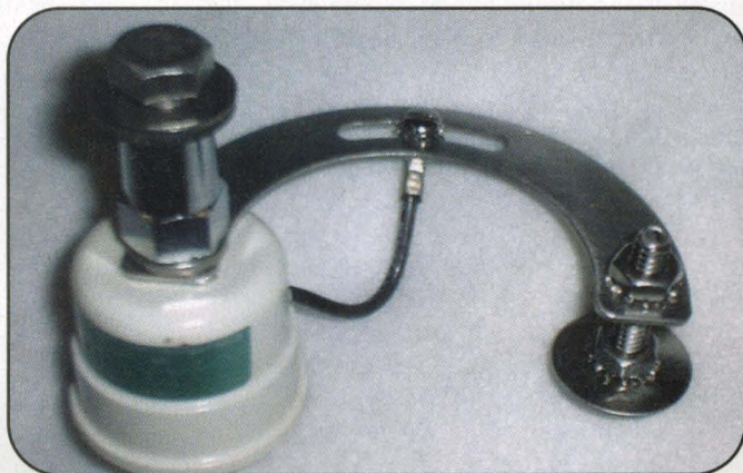
Photo C. A commercial 440-MHz vertically polarized DDRR antenna.
