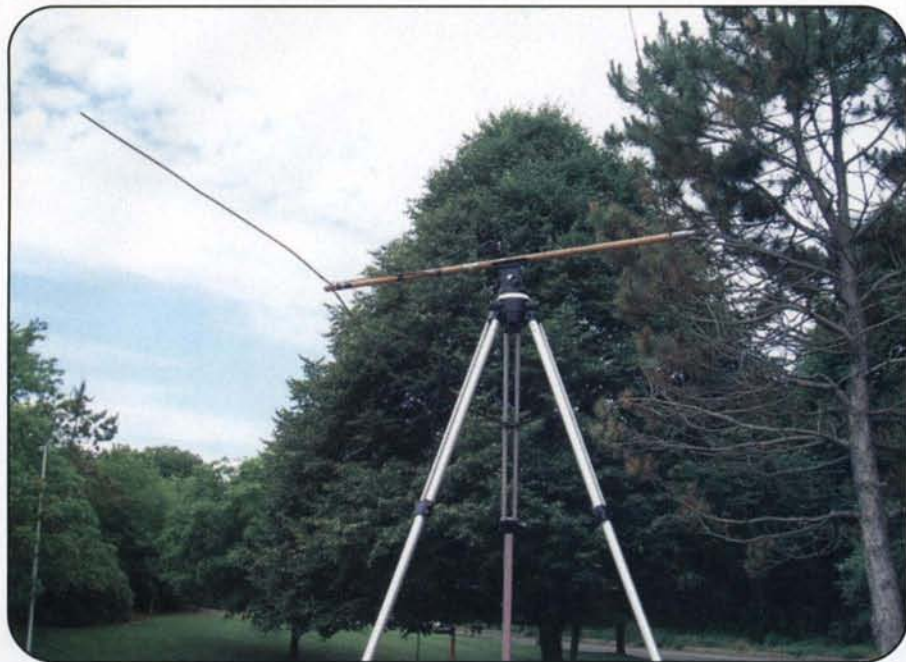
Photo D. A two-element Yagi that WB2AMU made for portable operation. It is designed to be mounted in a telescoping tripod, and because of its light weight, it can be positioned on the car roof while parked.
