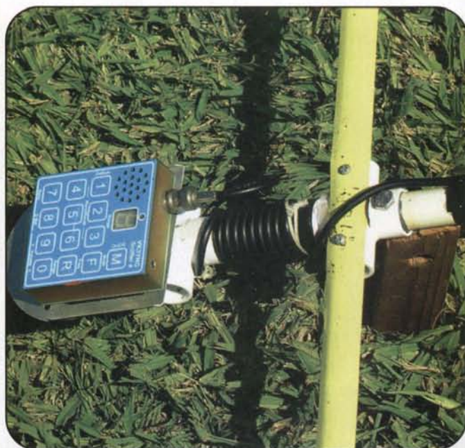
My Sniffer 4 is mounted on a swivel plate behind the reflector of the Yagi so that it can be face-up for either horizontal or vertical polarization. Note the coax choke balun to optimize the directional pattern and the wooden handle at the balance point to avoid wrist strain.
