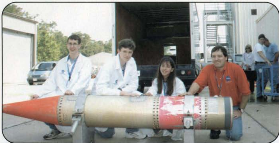
A CHS student team with the rocket payload section after recovery from the Atlantic Ocean. Notice the stripped paint from air friction and heating during the rapid ascent through the atmosphere with acceleration up to 17g's.
