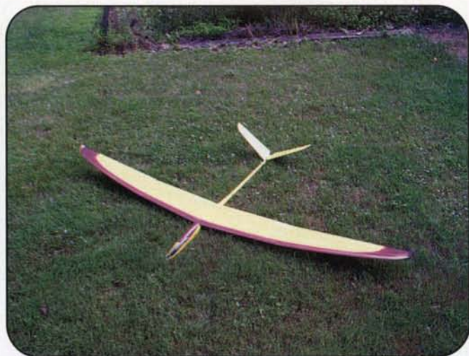
A hollow molded 2-meter fiberglass and carbon Gabby-E, the newest addition to my fleet and another folding prop.
