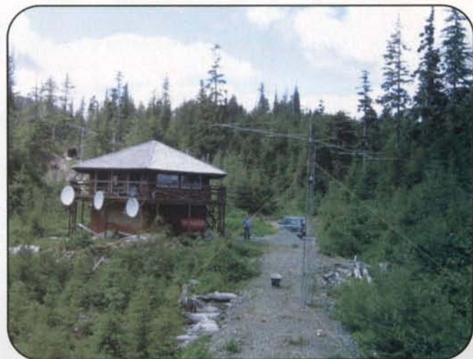
Here is the cabin as seen from the southeast. The 2-meter Yagi is on the porch to the left. The 6-meter Yagi is in the right foreground. The small dish is the satellite internet antenna. The other dishes are various satellite television antennas. All of this was 100% operational while we were there.
