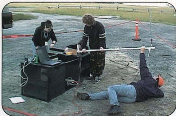
Experiment in action. The Yagi is pointed at the rocket high in the sky 10 seconds after a thunderous launch. The students who were tracking it were so disciplined that they never looked up to see the rocket launch, even though they were only 300 yards away.
