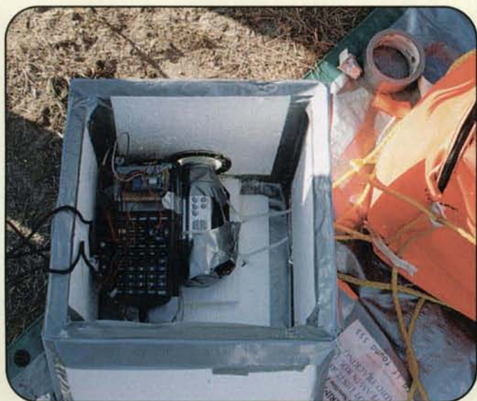
Calculator (TI-83) collecting data from a Vernier Data Interface connected to an analog 3-axis Honeywell magnetometer (HMC2300).
