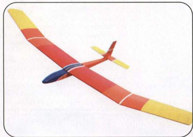
A simple rudder and elevator 2-meter glider, the "Gentle Lady."
