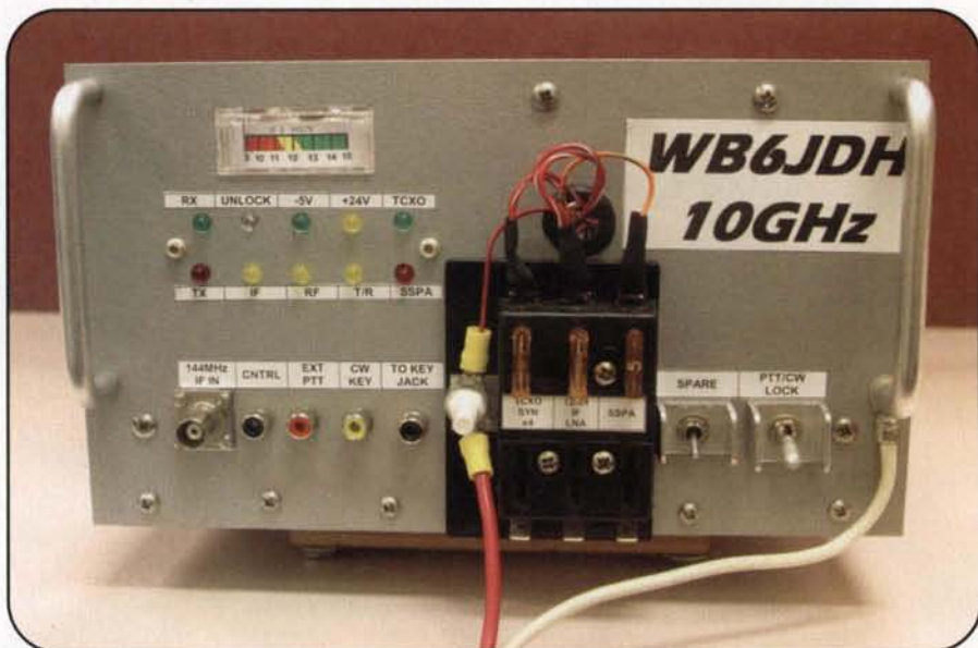
Photo B. Surplus material and previously exotic parts such as microwave mixers are easier to obtain these days. This X-Band system has a receiver noise figure of 0.7 dB, with transmit power of 900 mW measured at the antenna port. An 18-inch reflector is attached to the front of the chassis box with machine screws.
