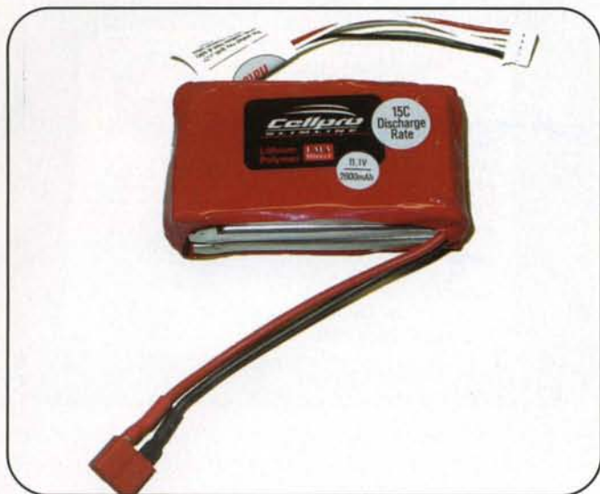
Photo 1. A LiPo pack showing the individual cell charging connector and also the standard discharge connection.
