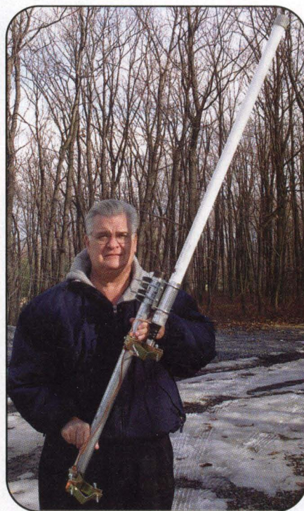
Gary Blacksmith, WA3CPO, holding the 23-cm omni antenna. It is designed to be well protected from intruding insects.
