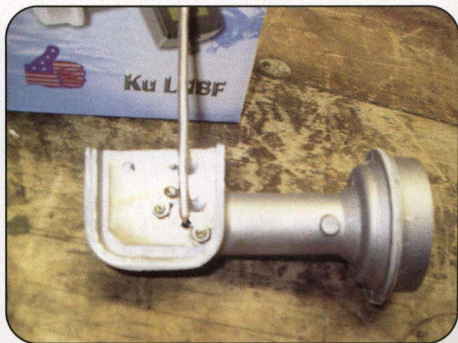
The KU-band LNB (low noise block) for 10 GHz ready to be resealed.
