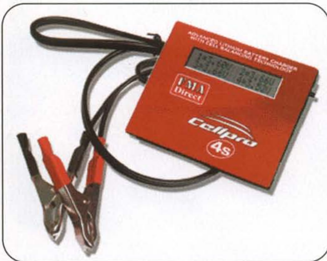
Photo 7. An FMA Cellpro lithium charger charges each cell individually through a pack's balancing connector and displays the charge rate and charge condition of each cell with completely automatic operation.
