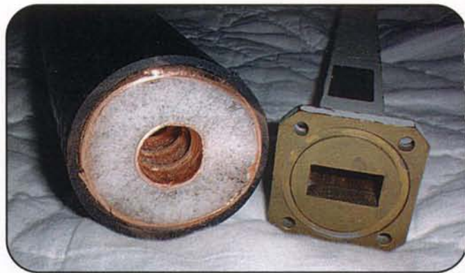
Photo A. Big coax vs. small waveguide.
