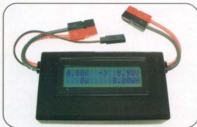
Photo 4. An AstroFlight Whattmeter is another way to measure power when connected between a battery and the load.
