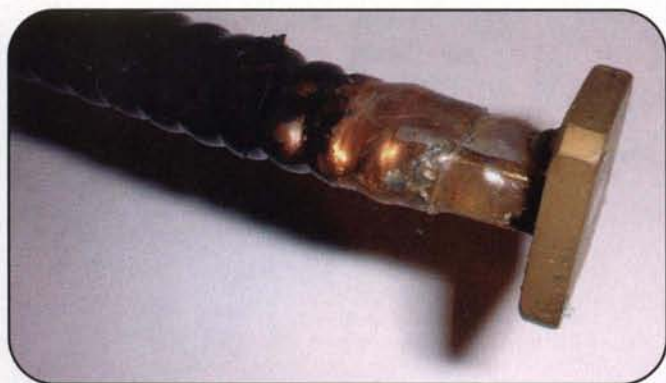
Photo B. Homebrew waveguide flanges for elliptical waveguide.
