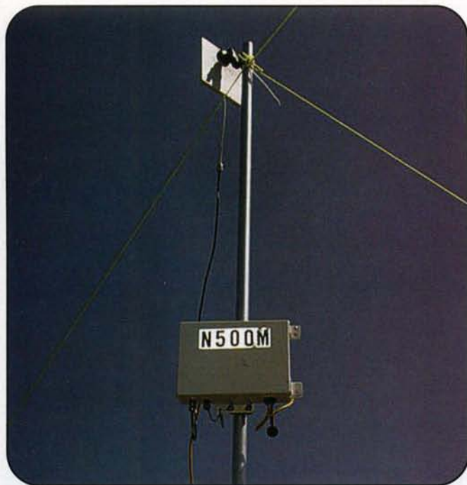
The Wild Ride command post. The radio is mounted in the steel enclosure and powered over the ethernet cable. (Photo by KD5OUG)
