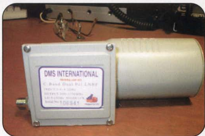
The DMS International C-Band LNBF (low-noise block with feed).
