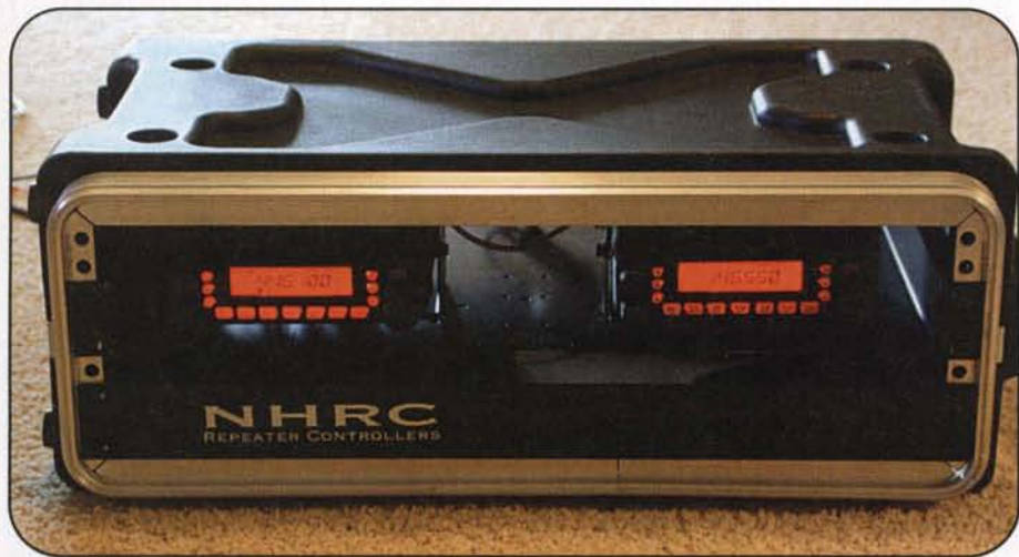
Photo C. The crossband repeater built using two independent FT-7800R transceivers controlled by an NHRC repeater controller.
