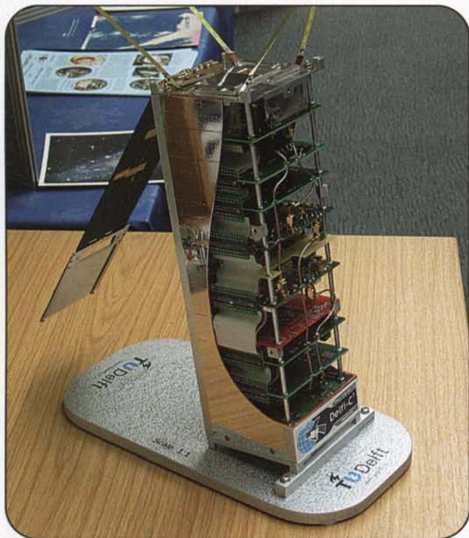
Full-size model of Delfi-C3, DO-64, roughly 4" x 4" x 12".
