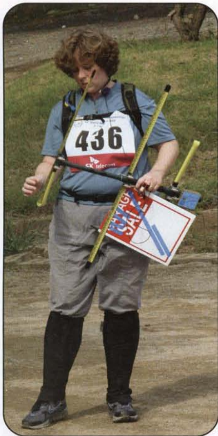
Jennifer Harker, W5JEN, unfolds her 2-meter measuring-tape Yagi in preparation for the 2-meter hunt at the 2008 World Championships. She designed the courses for this year's USA Championships in Bastrop State Park after earning her team position at South Lake Tahoe in 2007. (Photo by Dale Hunt, WB6BYU, courtesy W5JEN)
