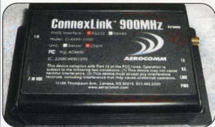
Photo A. The AeroComm 900-MHz, 1-watt modem.
