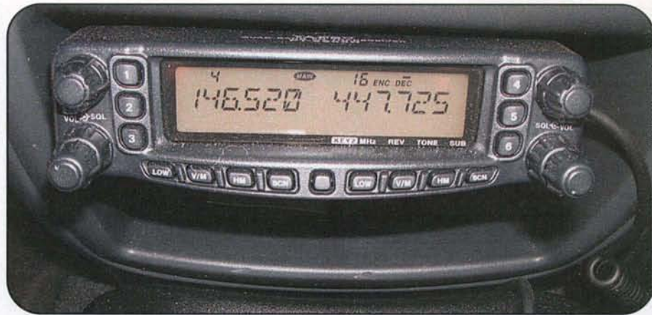
Photo A. A typical dualband radio that includes crossband repeat mode. (Photo via KØNR)
