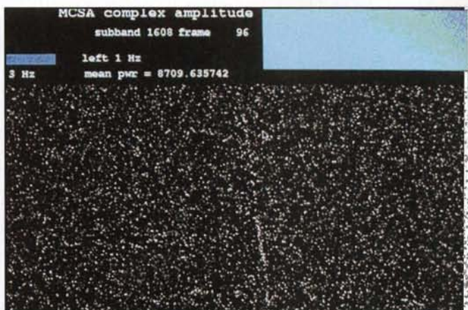
Figure 1. Drift-scan sweep of Quasar 3C273, about 3 dB out of the noise.
