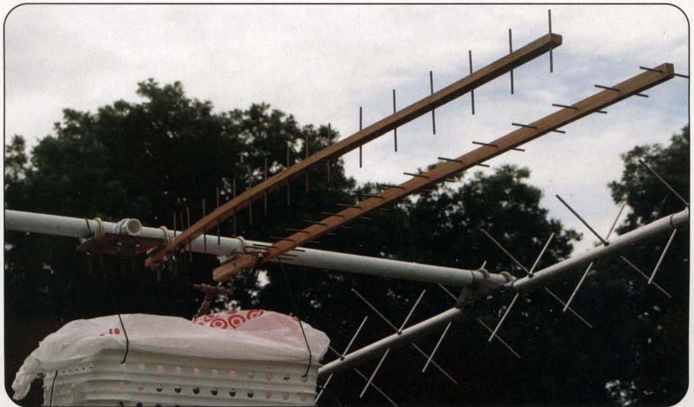
Cheap circularly polarized L-band Yagis with white box full of up-converter and amps. Note the expensive rain cover on the white box.
