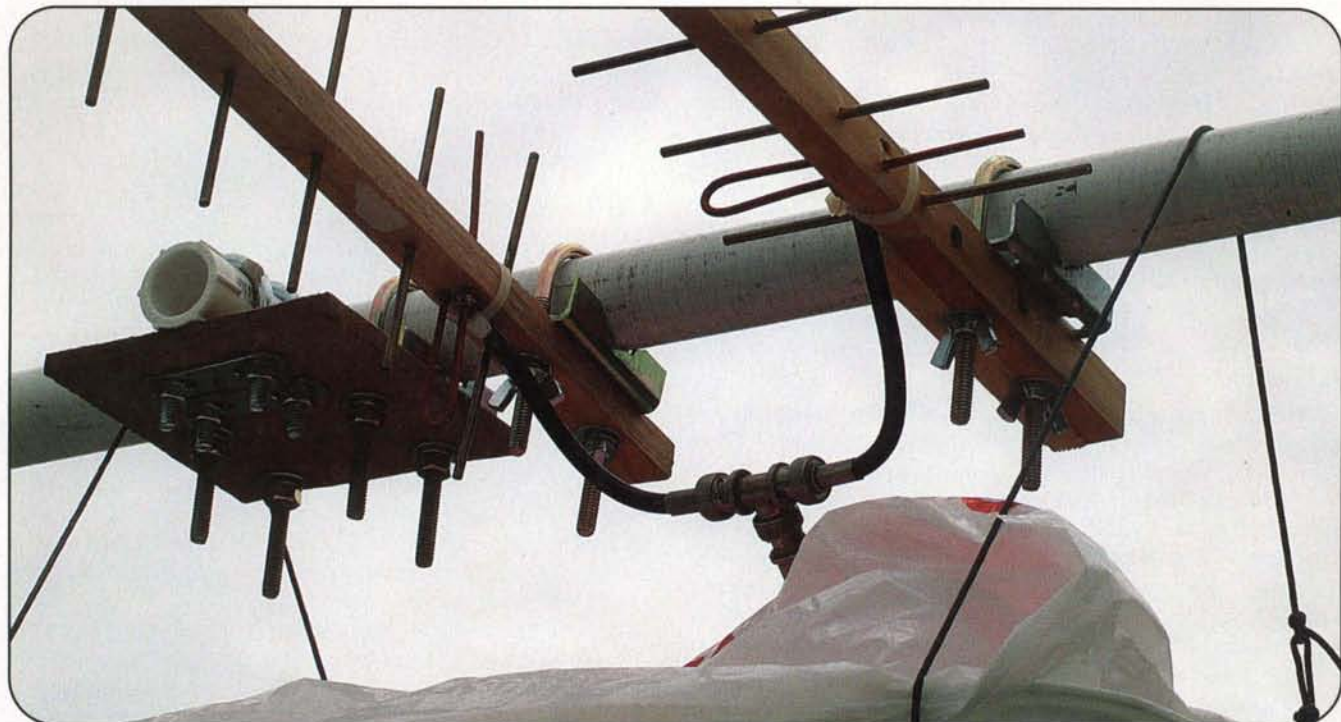
Feed details for L-band Yagis. Note that Yagis are rotated 90 degrees with respect to one another, and one is spaced a quarter wavelength down the boom from the other. The power splitter is made from two equal lengths (each an odd multiple of a quarter wavelength long) of 72-ohm coax.
