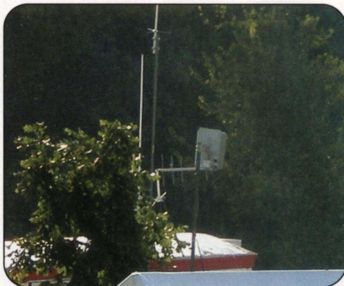
This is a view of the antenna on the communications trailer and the antennas from the Amateur Radio Field Operations Command Center. The HSMM antenna is pointed towards the church for Internet access, but the laptop computers in the Command Center were able to access the HSMM signal from the side lobe of this antenna. It was about 100 feet away. (Photo by AE5IB)
