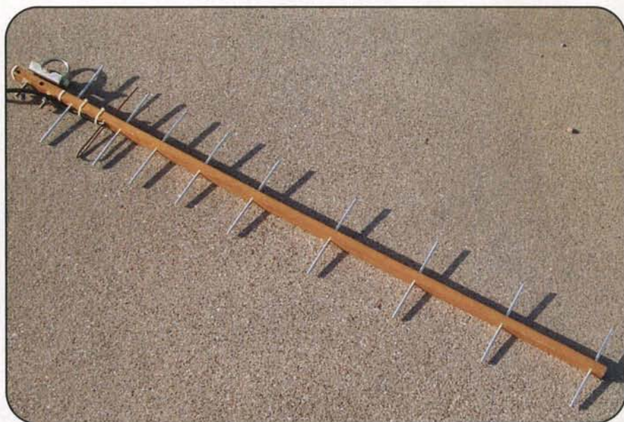
Photo A. Cheap Yagi for 915-MHz ATV.
