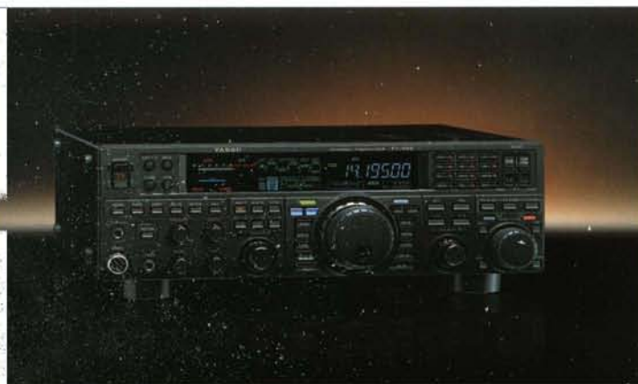
HF/50 MHz 100 W Transceiver FT-950
