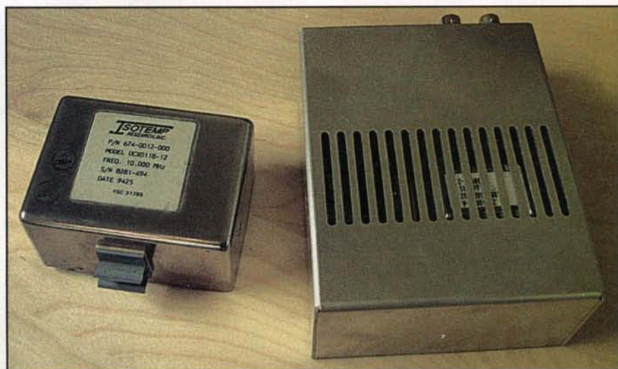
Figure 4. Two high-stability 10-MHz reference oscillators.
