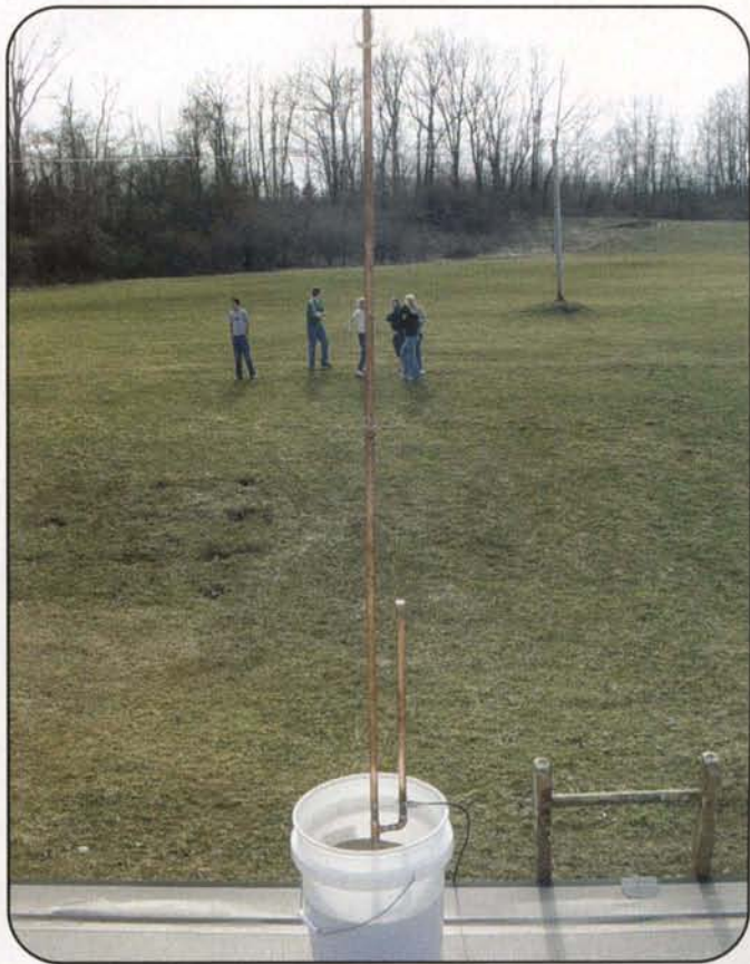
A homemade 2-meter copper cactus antenna stuck in a bucket of sand on the roof of the school. (All photos courtesy of the author)
