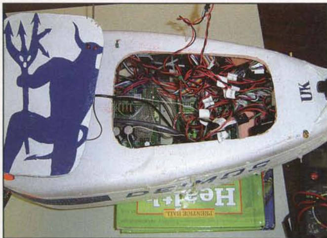
The three-processor, two VHF radio, redundantly powered system is packed into the fuselage for the trip to space.
