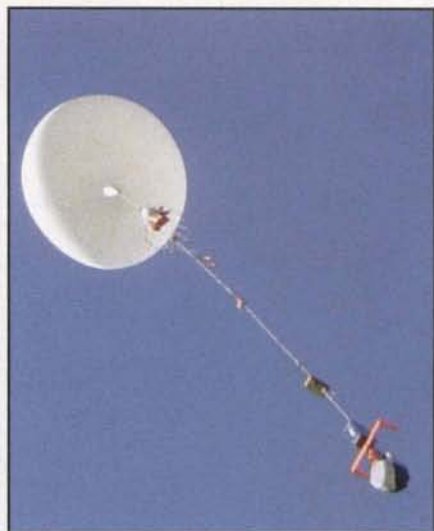
Next stop, the edge of space. BIG BLUE II at T+4 seconds (wings folded inside the fuselage).
