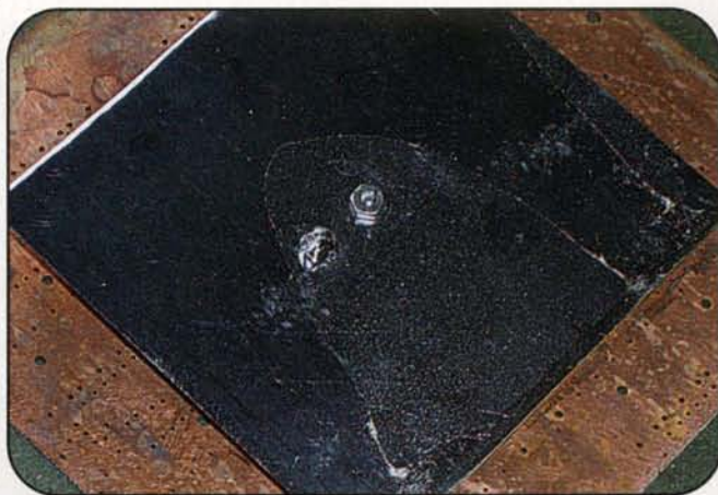
Photo C. A version of the patch antenna with a center bolt for better mounting.
