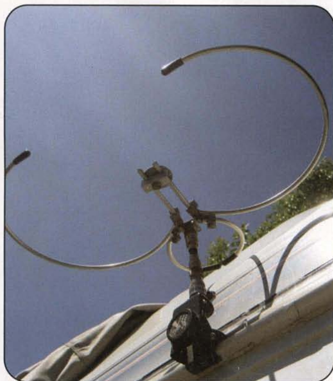
A dual-band KU4AB.com loop with solid-rod construction on WB6NOA's communications van, 144.2 and 432.1 MHz with one feedpoint!
