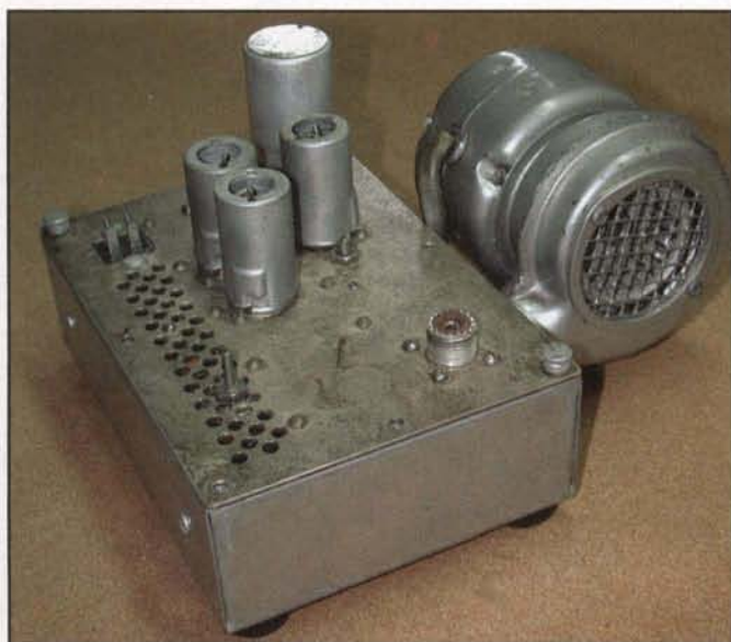
Photo D. A seldom seen and unique variation of the W2AZL converter, one using the rare Western Electric 416B triode, a tube designed for operation up to 4 GHz.
