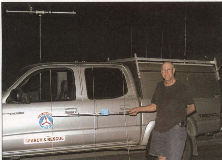
Photo 7. For ELT/EPIRB/PLB tracking, Bob Miller, N6ZHZ, prefers the folding three-element beam and VK3YNG Sniffer4 that he is holding, because this high-sensitivity system provides maximum range. The rotating Yagi atop his truck is for 2-meter transmitter hunting. In its place, he can mount his home-built cubical quad for 121/243 MHz. (Photo by KØOV)
