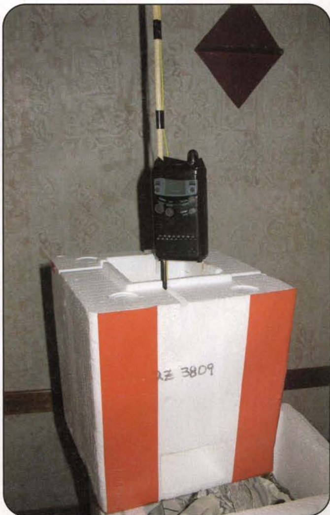
Photo 2. Alinco DJ-S11T with vertical dipole modification.
