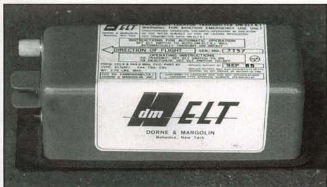
Photo 1. Old-style Emergency Locator Transmitters like this one are still installed in thousands of commercial and private aircraft. They do not transmit an ID or GPS coordinates, so they must be tracked by RDF when activated. (Photo by Tom Curlee, WB6UZZ)
