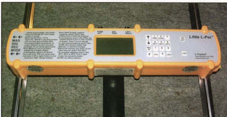
Photo 4. The LL-16 Little L-Per by L-Tronics is popular with Civil Air Patrol and other agencies that are responsible for ELT/EPIRB/PLB tracking. (Photo by KØOV)
